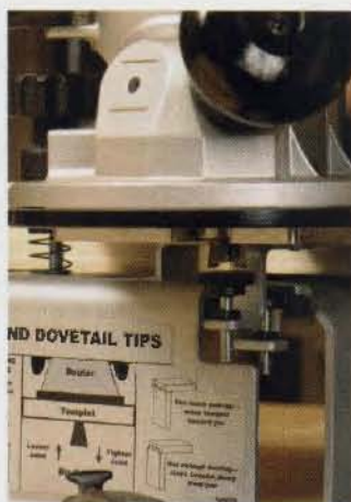
Another unique guide. The Porter-Cable is the only jig with built-in guides for setting bit depth. Instructions on the jig mean fewer trips to the manual.
