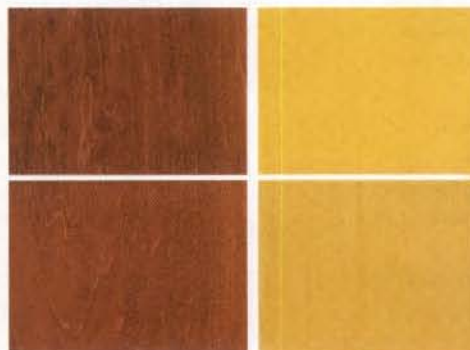
More lightfast. Alcohol-based, non-grain-raising dyes suffered some damage from the sunlight but not as much as the water-based dyes.
