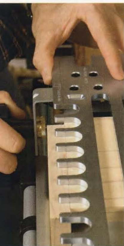
Helpful guide lines. The templates have scribe marks that are aligned easily with the back of the tail board, making setup fast.
