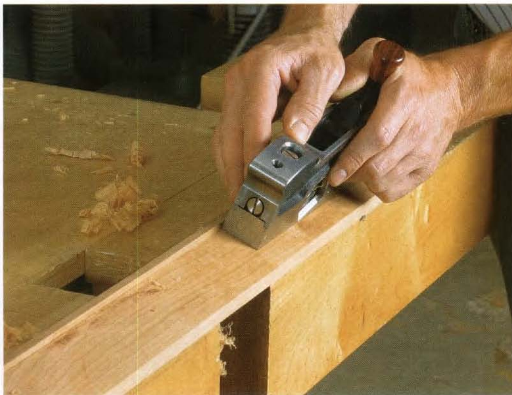
Clean up machine marks. Decorative rabbets on the door fronts (right) and the top and bottom moldings (above) of a case have surfaces that will be exposed when the cabinet is assembled. The shoulder plane is perfect for cleaning up the machine marks left by the tablesaw or router.
