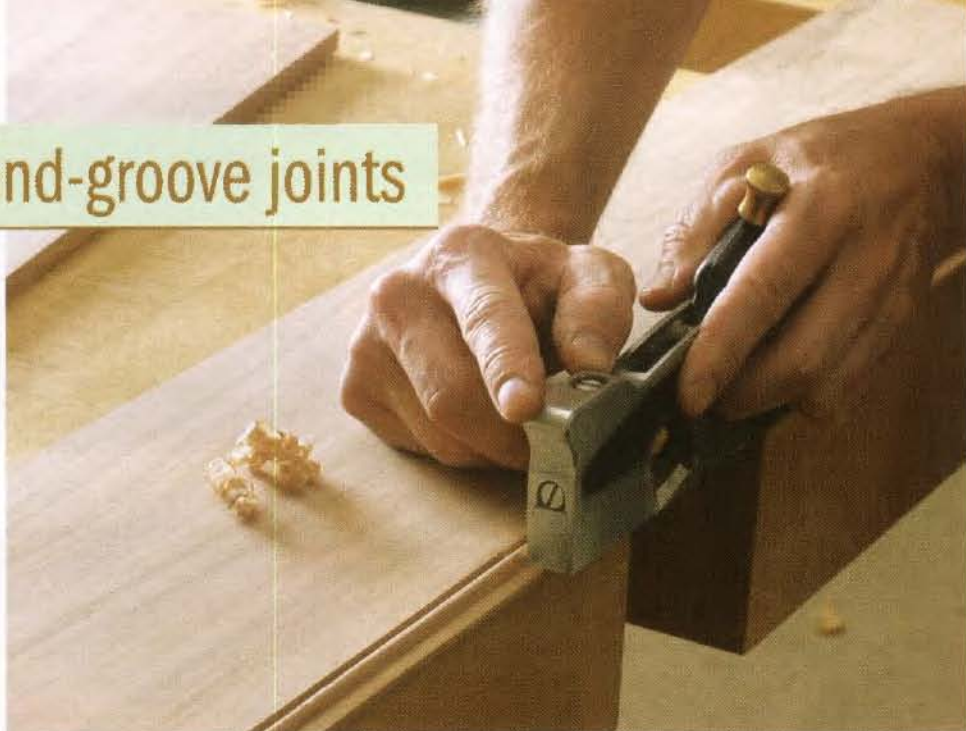
Tweak a tongue. A tongue-and-groove joint is a chore to assemble when the tongue is too tight. A few swipes on each side of the tongue solves the problem in short order.
