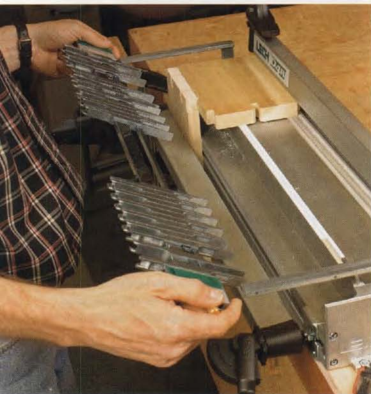
Flip and continue. For through-dovetails, once the tails are cut the template is simply flipped over to cut perfect pins.
