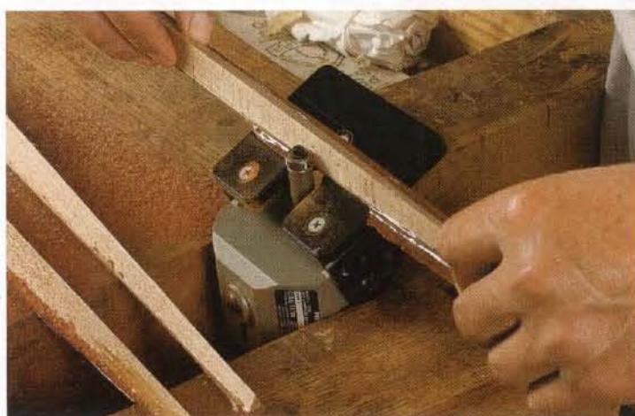
Trim the veneer. Use a laminate trimmer with an adjustable base to remove most of the overhanging veneer.
