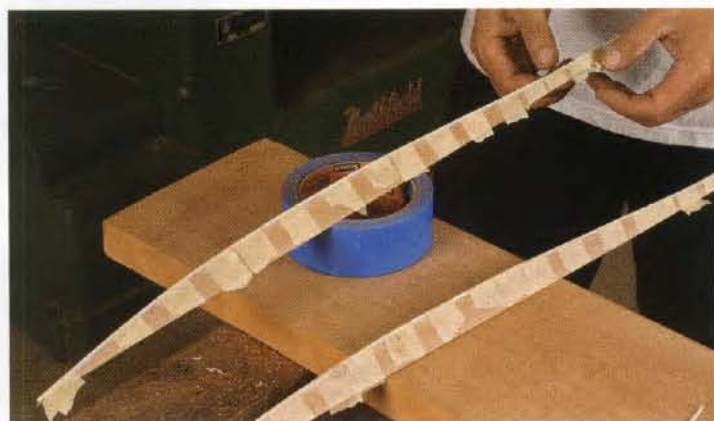
Apply the stringing. A thin bead of glue and plenty of masking tape secures the ivory or holly stringing in each leg section (above). The rabbet should be very slightly shallower and narrower than the stringing so that the latter can be sanded to final size (left).
