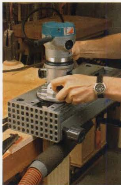
Good old pencil marks. After cutting the tails, you mark the jig at the centerline of each template finger and then align the pin fingers with those marks.
