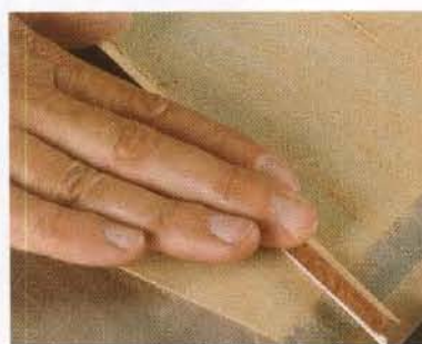
Apply the stringing. A thin bead of glue and plenty of masking tape secures the ivory or holly stringing in each leg section (above). The rabbet should be very slightly shallower and narrower than the stringing so that the latter can be sanded to final size (left).
