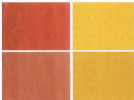
Water-based powder dyes faded fast. After only five weeks, the extent of the sun damage, particularly to the red-dyed areas, is obvious.
