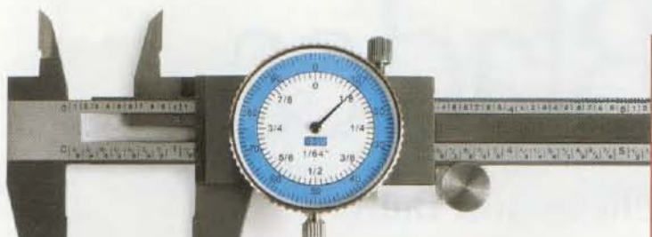
Hartville Tool. With a large blue decimal scale on the outside and a smaller, black-and-white fractional scale in the center, the dial on this model is a bit hard to read.
