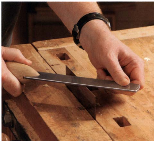
Part file, part burnisher. Glen-Drake's file-burnisher has three working surfaces: a flat, extrafine file, a flat burnisher, and two rounded, narrow edges for concentrated burnishing.
