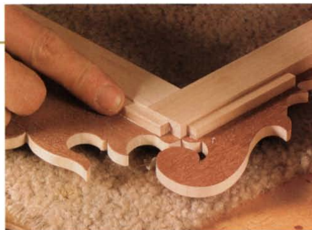
Add glue blocks. Apply small sections of wood to the back of the frame to reinforce the veneered attachments.
