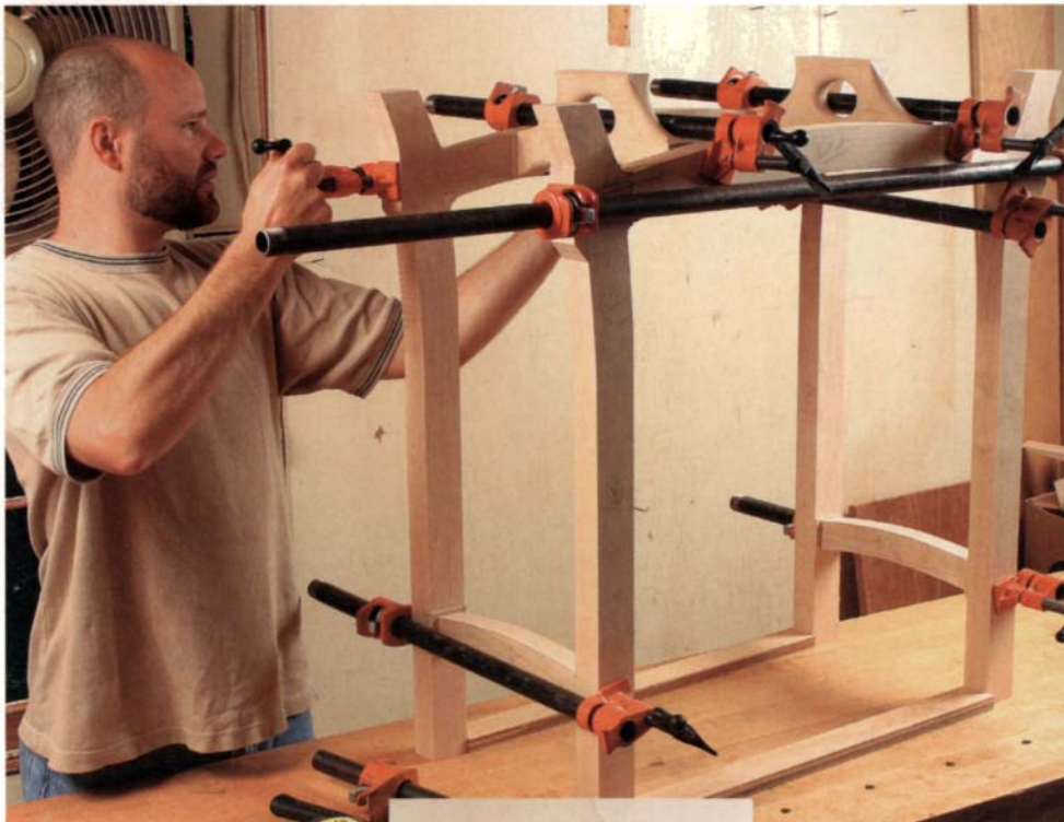
Clamping requires square surfaces. Note the stock left in strategic areas to serve as clamping pads. Be sure each joint closes completely.
