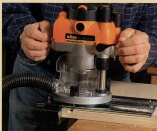
Versatile fence. The Triton's fence serves as an edge guide for straight cuts. It also comes with a circle-cutter pivot for routing circles from 6 in. to 14 in. dia.
