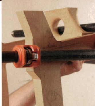
Clamping requires square surfaces. Note the stock left in strategic areas to serve as clamping pads. Be sure each joint closes completely.
