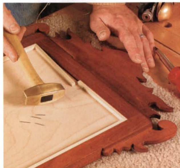
Install the mirror. After finishing the frame, place four dabs of clear silicone caulking on the inside of the frame and then lower in the mirror. Use tacks or a pin nailer to attach mitered trim to hold the mirror and plywood backing in place.
