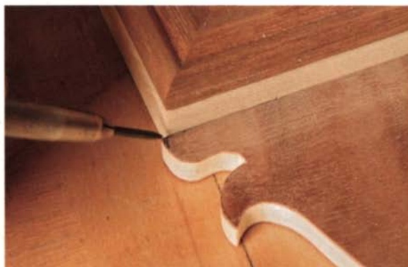
Fit to length. After the top and bottom crests have been cut out, hold them against the frame and mark any overhang for removal.
