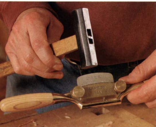
Tap or twist. All of the standard-angle shaves Gochmour tested allow for easy blade adjustments via thumbscrews on the lever cap (above) or with the tap of a hammer (below).
