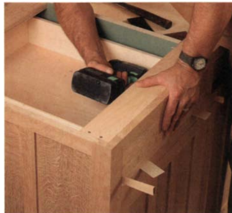
Install the drawer and then the front. Shims ensure that the space between the frame and the drawer front is uniform on all four sides.
