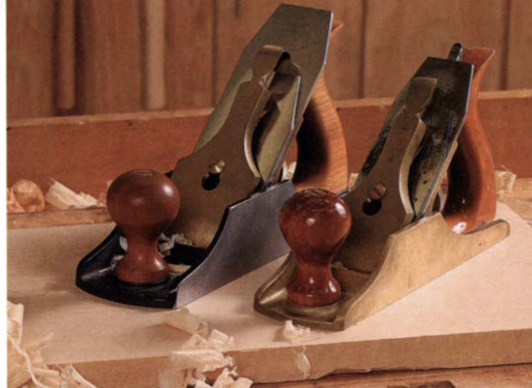
Tale of two planes. The 9-in.-long No. 4 (right) has a 2-in.-wide blade. The No. 4½ is 10 in. long and has a 2½-in.-wide blade. The No. 4½ weighs close to 5 lb., about 1 lb. more than the No. 4.
