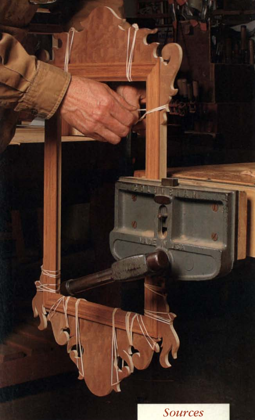
Add glue blocks. Apply small sections of wood to the back of the frame to reinforce the veneered attachments.
