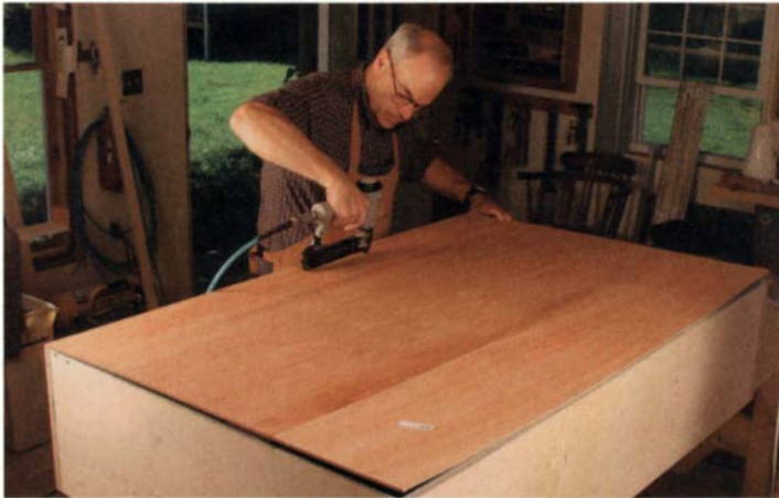
Brads secure the back. Gibson uses brads to attach the 1/4-in. plywood back of the cabinet. This gives the inside a finished look and adds stability to the box.
