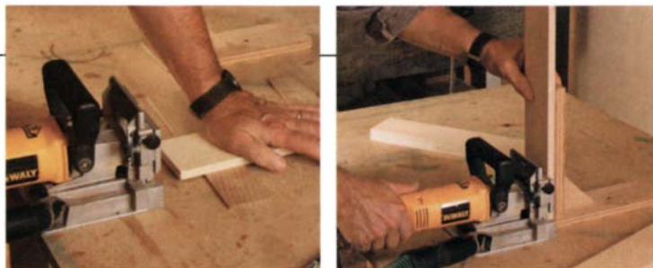
Biscuiting the drawers. To center the slots in 1/2-in. plywood sides, place the workpieces on 1/8-in. shims (left). Gibson uses a right-angle jig to support the drawer sides (right). A 1/8-in. shim is needed under the end.
