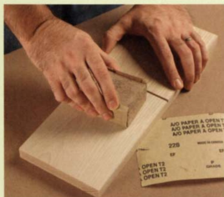
Sand the surface. Because bleaching raises the grain, sand the wood with P220-grit paper before applying a finish.
