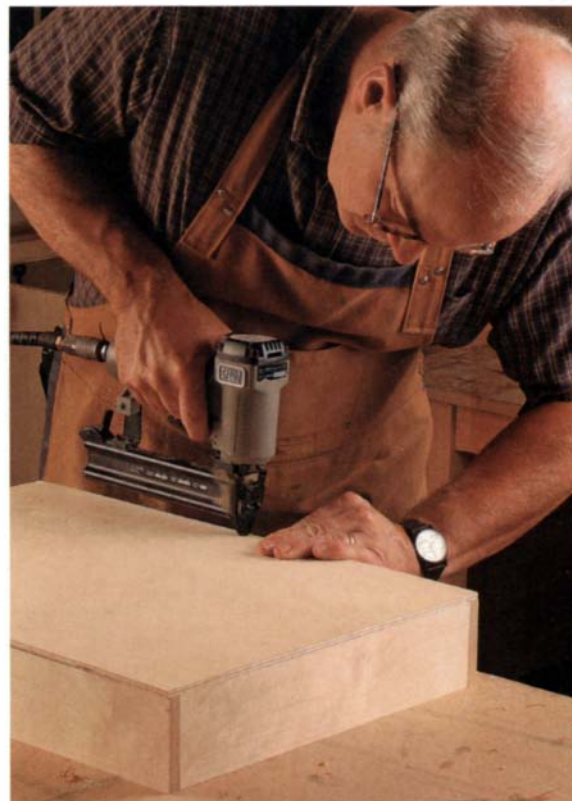
Glue and brads attach drawer bottoms. This simple approach provides strength and durability.
