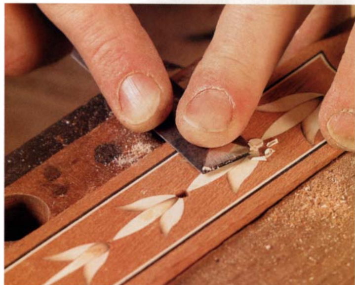
Inset the plugs. Drill holes for the circles with a brad-point bit and insert the plugs with a little hide glue. When dry, pare them flush with the leg.
