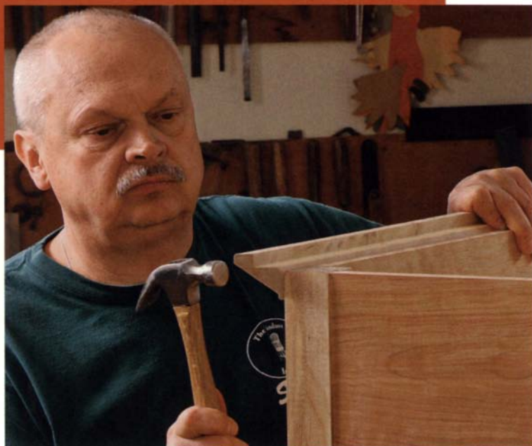
Tack the cornice into place. The molding's angular profile accentuates the square corners of the piece.
