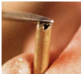
Custom plug cutter. The author files teeth on the end of a brass rod (above) and uses a drill press to drill the holly plugs. Clear tape prevents the plugs from falling out when slicing them free with a handsaw (right).
