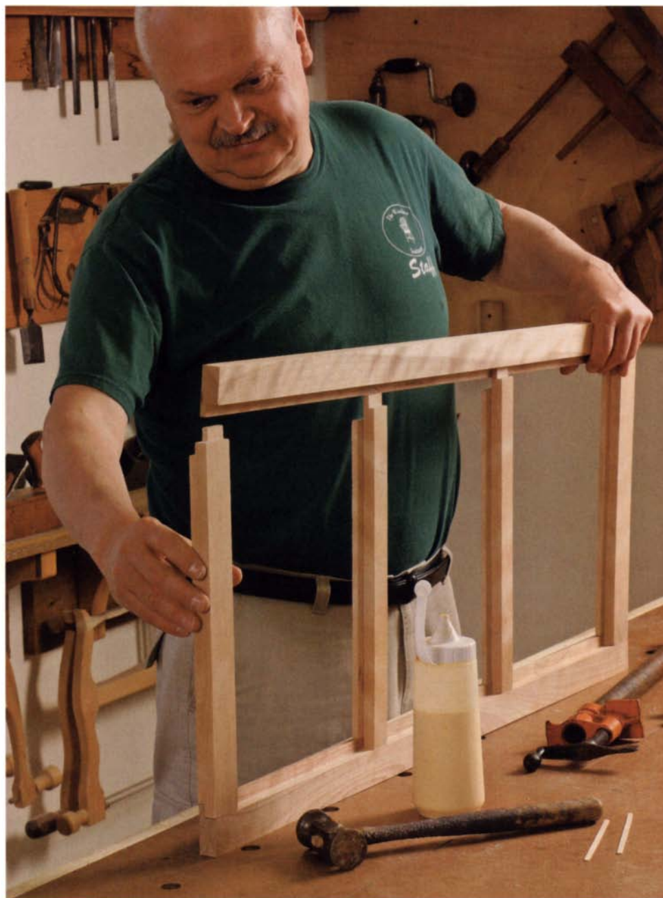
Assemble the door frames. Dry-fit the doors, check them for square, and prepare surfaces for finishing before breaking out the glue bottle.
