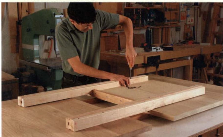
Mount the slides. Use screws to secure one end of the slide to one of the top halves (left). Then screw the opposite end of the slide to the other half (above).
