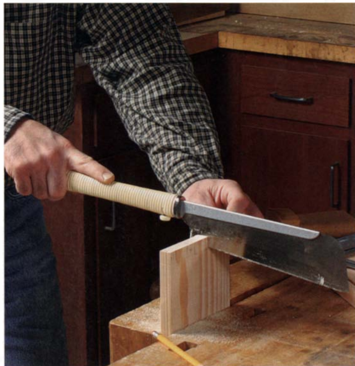
Hold the saw at the far end of the handle. Cut only on the pull stroke, and let the saw's weight do the work.
