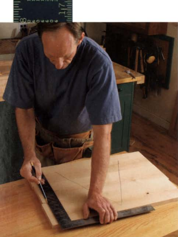
Framing square for bigger jobs. When scribing a line across a wide workpiece, like a panel, a framing square is Gochnour's tool of choice.
