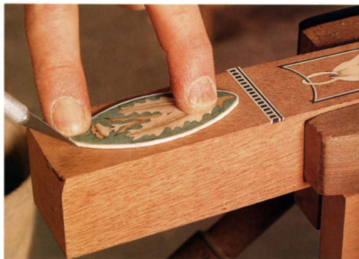
Crowning glory. The pilaster of each leg is decorated with an oval inlay that can be bought or shop-made.
