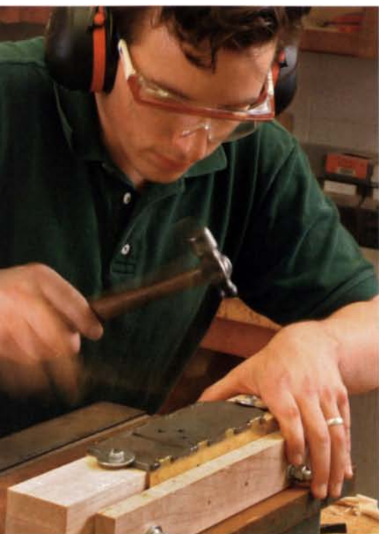
Pounding metal. Using a wooden jig resting on an improvised anvil, the author joins the dovetails together with a ball-peen hammer.
