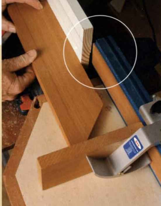
Good cuts need good support. A pair of extension wings with stop blocks support long pieces and make for accurate cuts.
