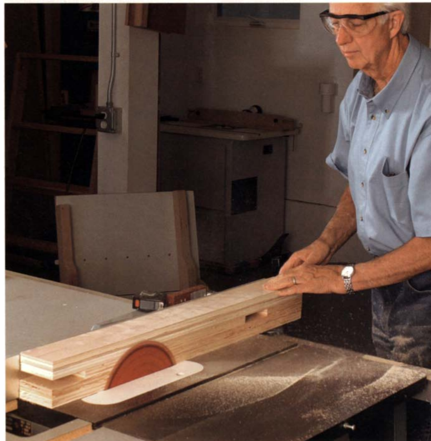
Clean up the edges. After the legs, aprons, and stretchers have been assembled, run both edges past a sawblade to clean up glue residue and leave them at the final 3½-in. width. Cut the first edges with the fence at 3⅞ in., and the opposite edges at 3½ in.
