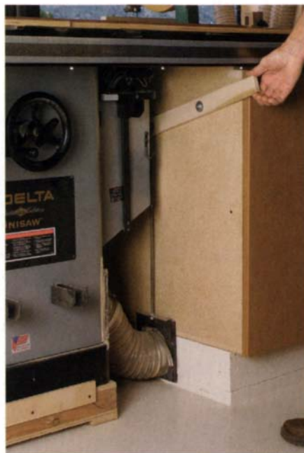
Easier to operate. To avoid bending down, the author attached a simple lever to the blast gate for the tablesaw.
