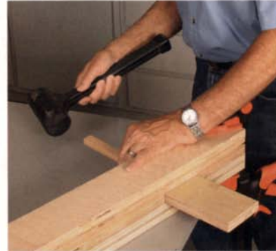
Clamping the leg. When the sections have been glued together, turn the assembly upward and apply the clamps. Waxed paper protects the work surface. When the glue has dried, knock out the taped spacer block with a mallet and a thin piece of wood to reveal the mortise.
