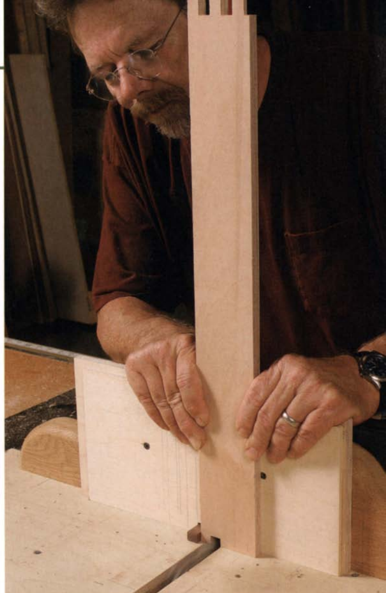
The ends of each piece are identical. For the first cut, butt the top edge of the workpiece against the key.
