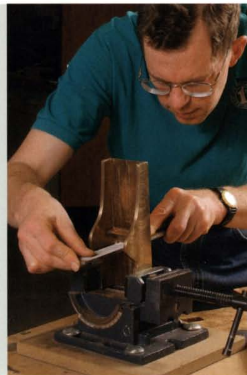
Opening the mouth. The mouth needs to be filed open very gradually until the blade just has clearance.
