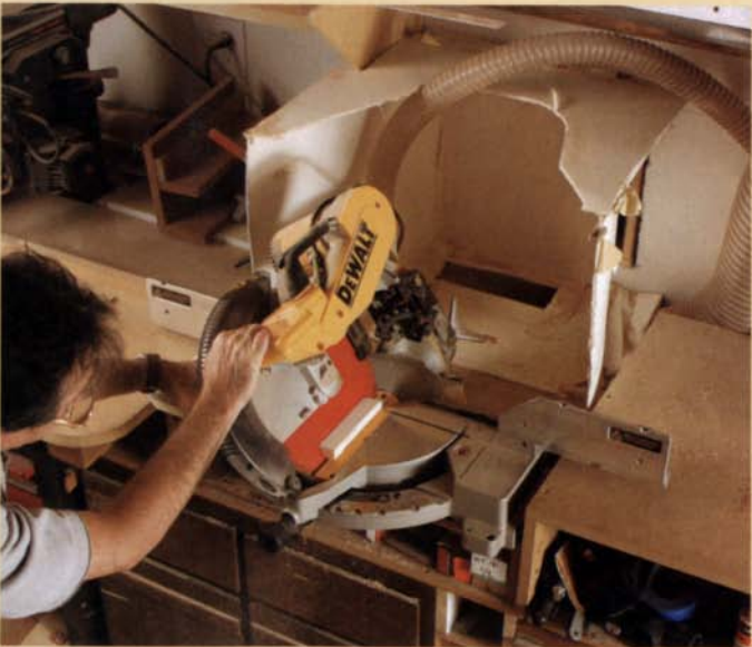
A built-in miter saw. Putting a miter saw into an existing bench provides support for long pieces and a dust-collection booth.
