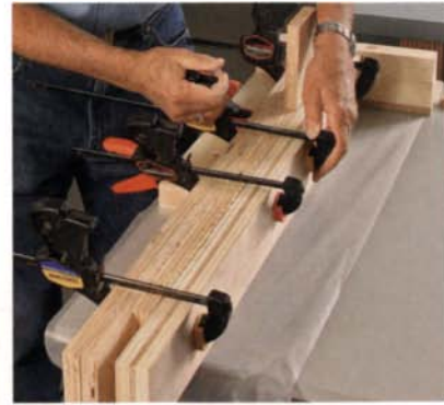
Clamping the leg. When the sections have been glued together, turn the assembly upward and apply the clamps. Waxed paper protects the work surface. When the glue has dried, knock out the taped spacer block with a mallet and a thin piece of wood to reveal the mortise.
