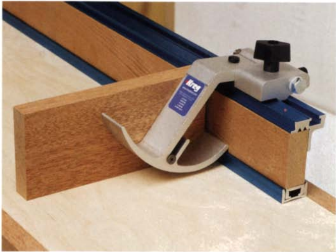
Stop block for miters. The author screws a block of wood to the stop block to give mitered ends a larger surface to register against.
