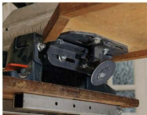
A good connection. This two-part coupler (available at www.sawhelper.com ; 800-441-1388) ensures that removable extension wings align evenly with the saw's table.
