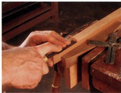
Clean up the cut. Use a chisel to square the arc left by the jointer. Veneer the back of the leg first (right), then the two sides, and finally the front.
