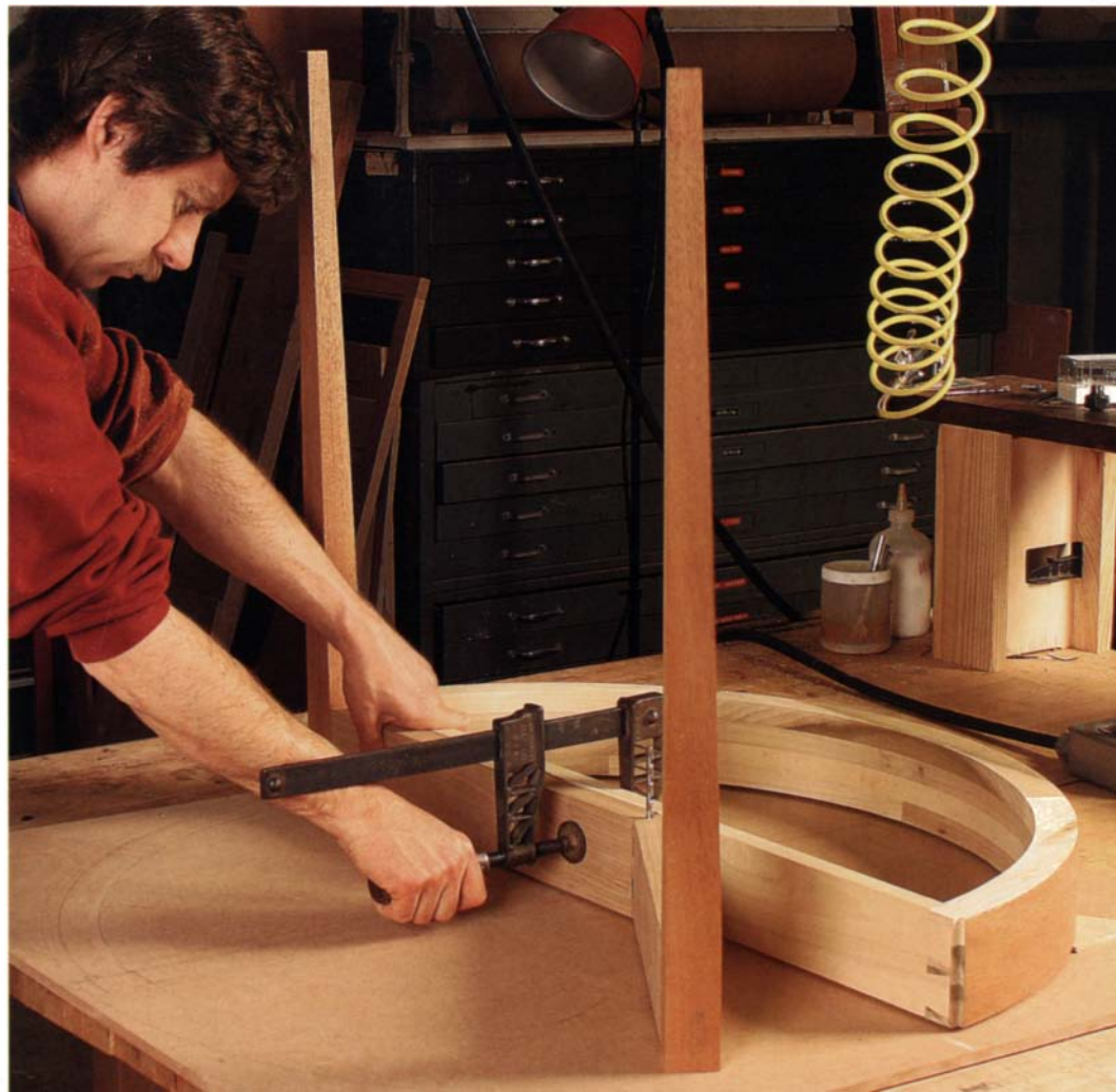
Attach the rear legs. The back legs are mortised to the swinging rails, and both the legs and the back of the apron are notched to fit (above). With the knuckle joints temporarily pinned (right), dry-assemble the rear legs and packer block to the apron to check the clearance for the tabletop.
