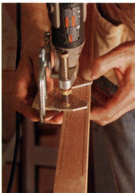
Groove the legs using a Dremel tool or laminate trimmer fitted with a router base and guided by a fence. Groove the arch at the top of the stringing by extending the bit out from the collet, which allows the shank to be guided by a template.
