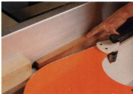
Set the jointer to cut the same thickness as the veneer. Use a stop block clamped to the fence to limit the length of the cut.
