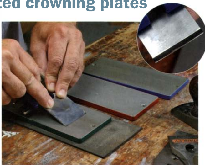
A perfectly crowned plane blade. The four diamond-coated plates are dished a precise 0.0025 in. across their width, ensuring an equally precise crown on plane irons.
