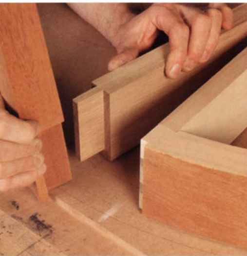
Attach the rear legs. The back legs are mortised to the swinging rails, and both the legs and the back of the apron are notched to fit (above). With the knuckle joints temporarily pinned (right), dry-assemble the rear legs and packer block to the apron to check the clearance for the tabletop.
