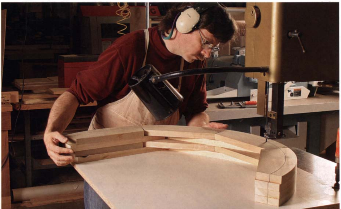
Use the pattern as a template. After the first layer of the bricklaid core has been glued, trim the overhang with a flush-trimming bit guided by the full-size pattern.
