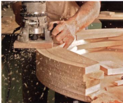
Flush-cut each layer. After each layer is glued, flush-cut it to the rest of the core using the previous layer to guide the router.
