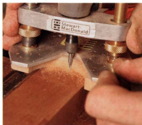
Groove the legs using a Dremel tool or laminate trimmer fitted with a router base and guided by a fence. Groove the arch at the top of the stringing by extending the bit out from the collet, which allows the shank to be guided by a template.
