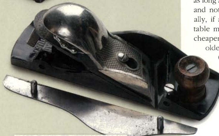
Millers Falls No. 7 skew block plane with removable side plate
