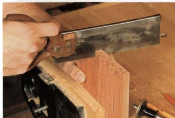
Hand saw the pin lines. With the knife lines as a reference, use a dovetail saw to cut along each pin line.
