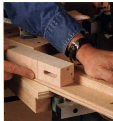
Locate the taper's start. Align the beginning of the taper with the edge of the jig and tighten the infeed knob.
