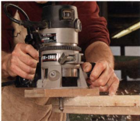
Use the pattern as a template. After the first layer of the bricklaid core has been glued, trim the overhang with a flush-trimming bit guided by the full-size pattern.
