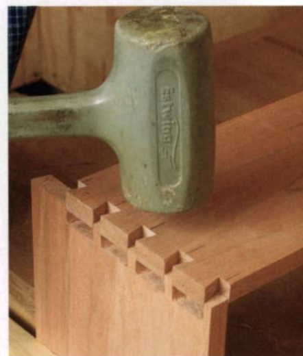
Test the fit. Good-fitting dovetail joints should go together with only moderate hand pressure or a little persuasion from a mallet.
