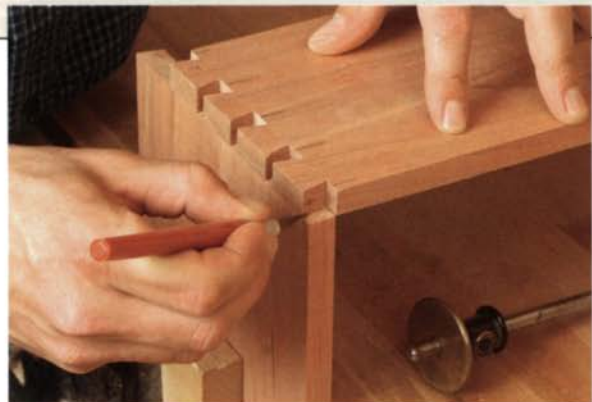
Mark for the pins. Use a marking knife to scribe the pin lines on the ends of the top and bottom.
