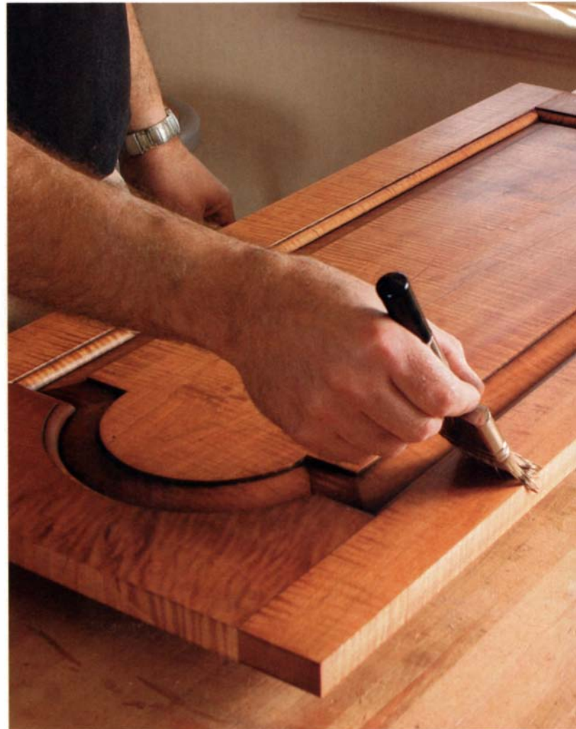
A final coat of shellac. After the glaze has cured overnight, seal it with a final coat of thin shellac. Finish with a coat of wax.
