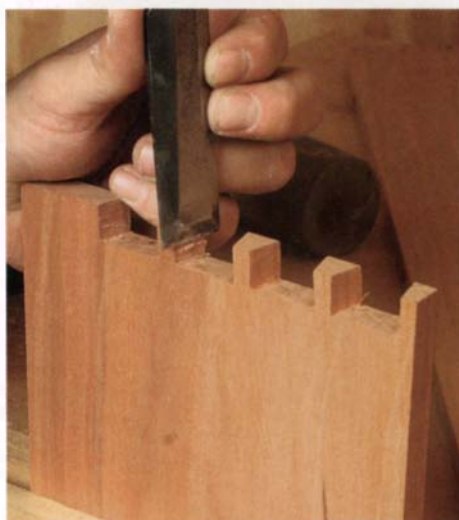
Trim the excess. After routing, a thin web of wood sometimes remains in the pin. Use a chisel to remove the web and shave away excess stock as needed.
