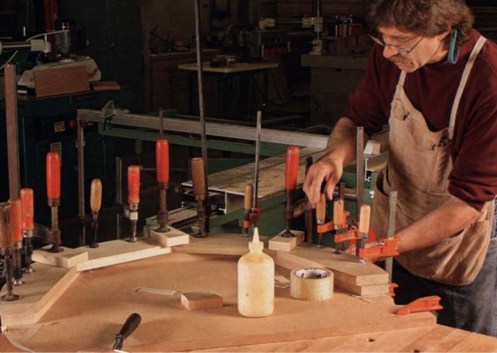
Build the apron's core. The poplar core is bricklaid by alternating three- and four-section layers. Use plenty of glue and clamps to ensure a solid bond between the layers.
