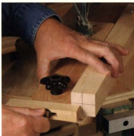
Locate the taper's end. Marks on the stock align with the edge of the jig, which is the cut line. After fixing the outfeed knob, adjust the stop to clear the blade.
