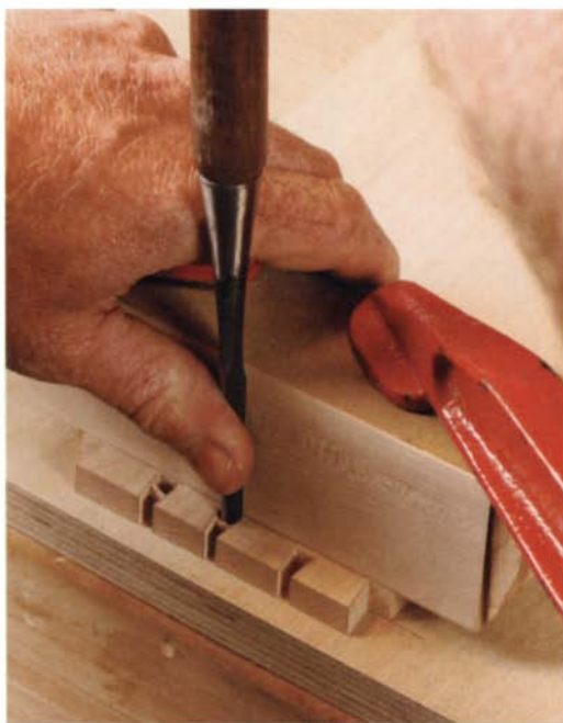
Chopping the tails. Use the second angled chopping block to guide the final cuts on the tails.
