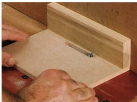
Slot the jig on a router table. The jig's hardwood fence rides along the router table's fence, accurately slotting the jig's MDF base.
