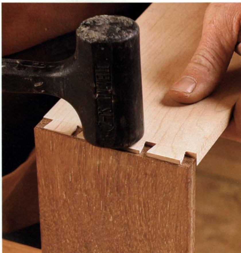
A perfect fit. The secret to well-fitting dovetails is to gradually pare away small amounts of wood, checking the fit regularly.
