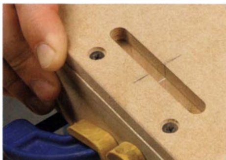
Mark centerlines on both the jig's slot and the workpiece. Line up the centerlines and clamp the stock in the jig.
