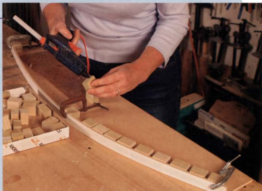
Use more blocks to stiffen the template. Glue more blocks to the base and the back of the strip. Take care not to alter the curve.
