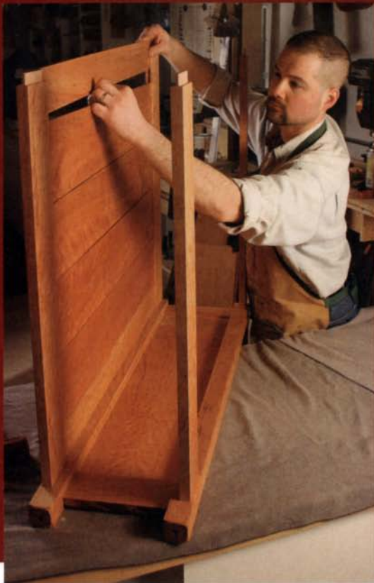
Next come the stretchers and the back. You may want to enlist a helper when putting together the shiplapped back.
