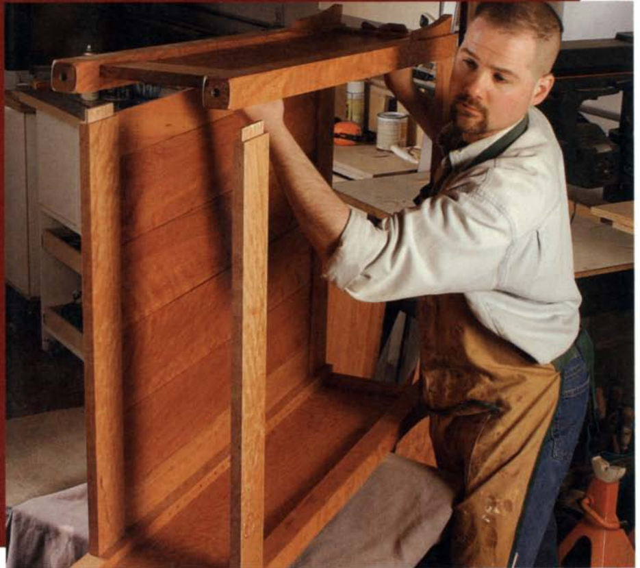
Top off the assembly with the final side. Use pine blocks on each side of the corbels to transfer clamping pressure to the posts.
