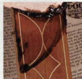
Wipe on a gel stain. Thick gel stains are less likely to seep into the protected inlay areas than liquid dyes and stains.
