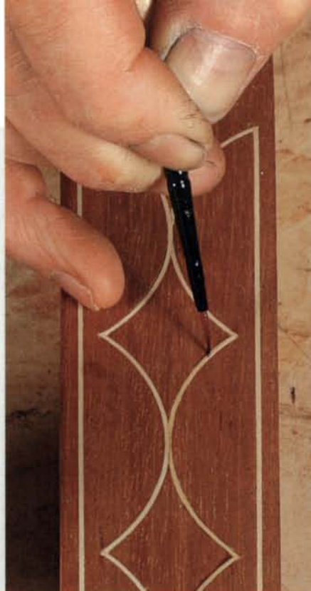
Brush on the sealer. With a new #1 artist's brush, apply several coats of either shellac or lacquer to the stringing.
