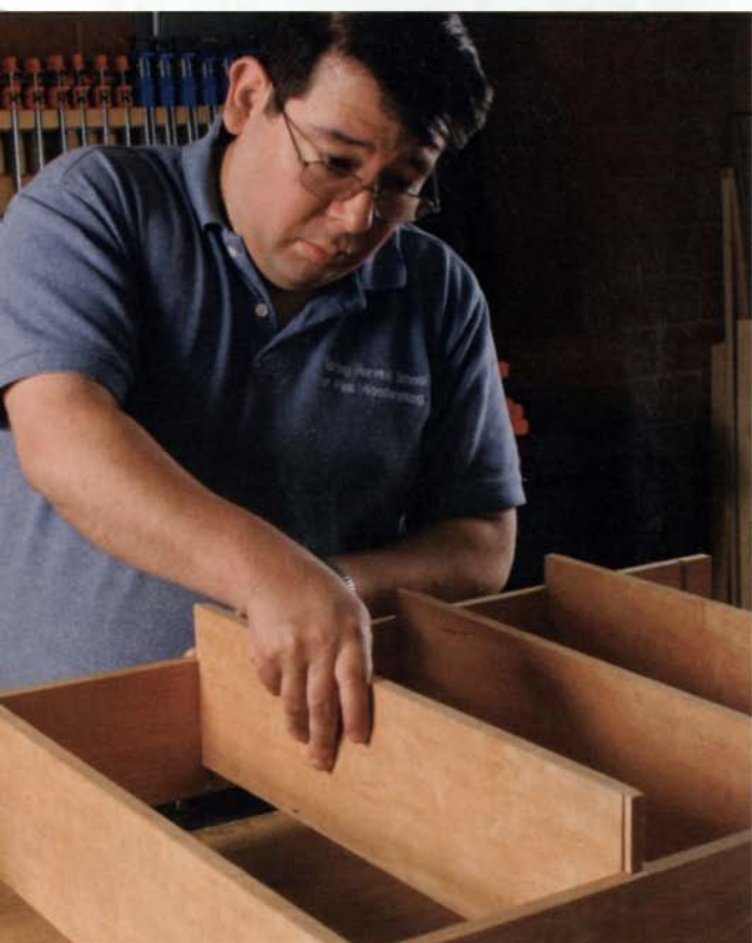
Sliding into place. The shelves will be hammered home and planed flush to reveal snug-fitting dovetails.
