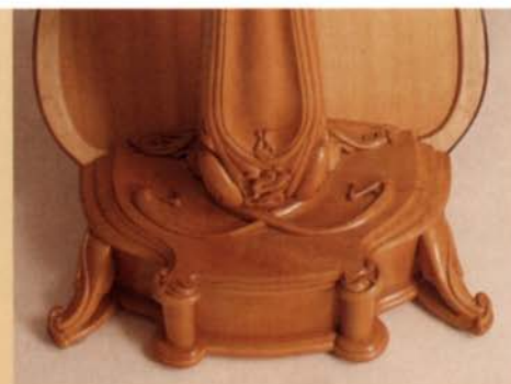
Form and function. The base features decorative carvings on top and serves as a precisely fitted mounting surface for the harp's soundboard.
