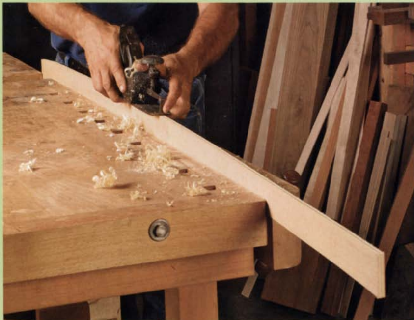
Plane a convex curve. With the sole of the compass plane set to the desired curve, make several passes, putting pressure on the nose of the plane until the curve in the workpiece is fair.
