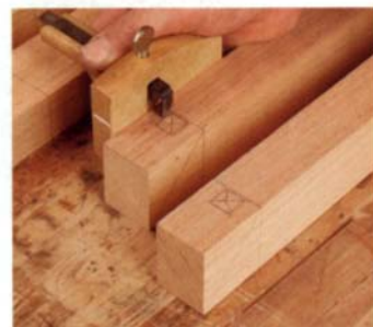
Lay out the mortises on both sides of the workpiece. Locate the mortise \frac{1}{16} in. up from the inside edge of the joint.
