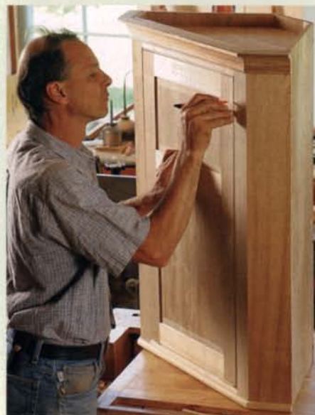
Mark the hinge locations. With the door held in place, transfer the hinge locations from the face frame to the door.
