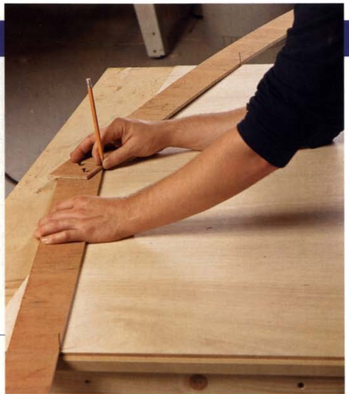
Arc jig. This simple jig allows you to draw a perfect arc of almost any size without having to calculate the radius.
