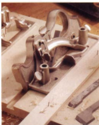
The Stanley No. 444 dovetail plane is hard to find. It's also one of the more complicated planes to set up.
