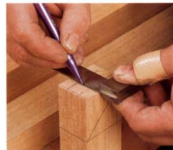
Lay out the tenons. Locate them so they will align precisely with the mortises. Also, lay out all sides of the sawcuts that will form the cheeks of the tenon.
