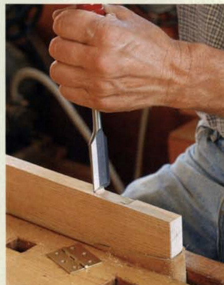
Chop the mortises. When cutting the hinge mortises in the stiles, protect the door from the vise with a piece of leather.
