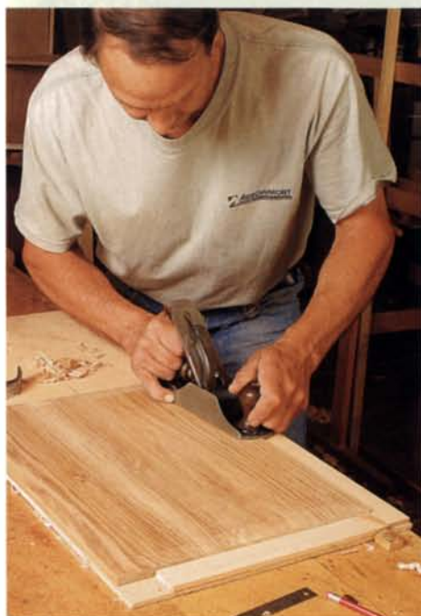
Raised door panels. The delicate bevel on the front of the door panels can be cut with handplanes. A block plane works best on the end-grain bevels.
