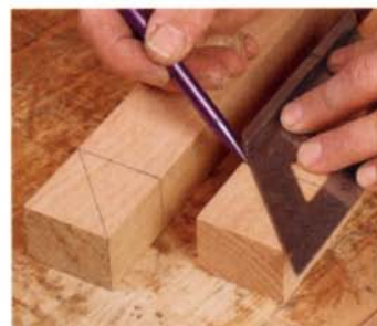
Lay out the miters. Draw the 45° miter and then scribe a baseline around the workpiece.
