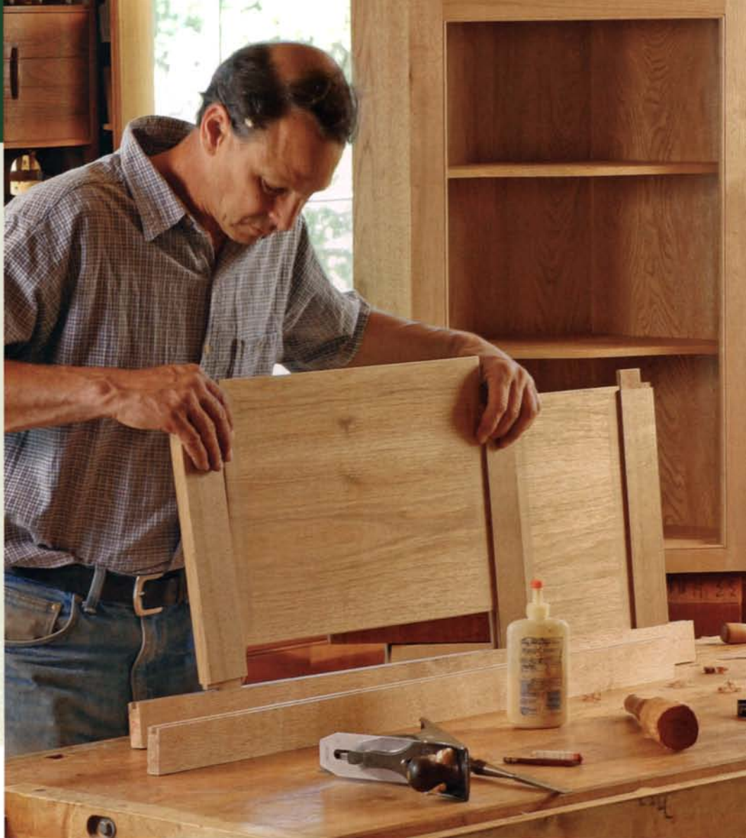
Assemble the door. The cabinet door is a frame-and-panel design with mortise-and-tenon joinery. The extra length on the ends of the stiles is sawn away after the door has been glued.
