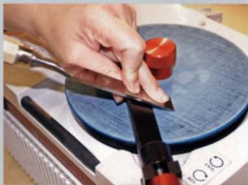
Tool-guide bar is adjustable. For sharpening bevels, the guide bar supports chisels and plane irons at the correct angle (bottom). The bar can be removed for grinding flat surfaces (top).
