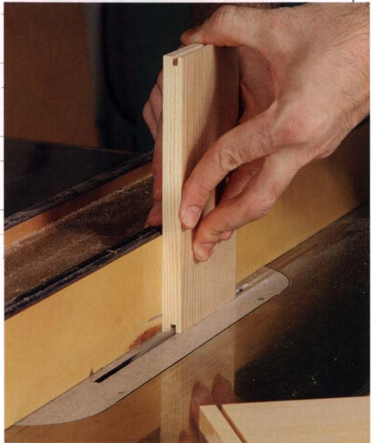
Rabbet the front and rear pieces in two steps. Move the front and rear drawer pieces vertically across the blade (above) to make the first part of the rabbet. Use a zero-clearance insert plate around the blade to support the workpiece. With the piece flat on the table (left), make the second cut, leaving a tongue that will connect with the side pieces.
