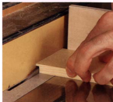
Rabbet the front and rear pieces in two steps. Move the front and rear drawer pieces vertically across the blade (above) to make the first part of the rabbet. Use a zero-clearance insert plate around the blade to support the workpiece. With the piece flat on the table (left), make the second cut, leaving a tongue that will connect with the side pieces.
