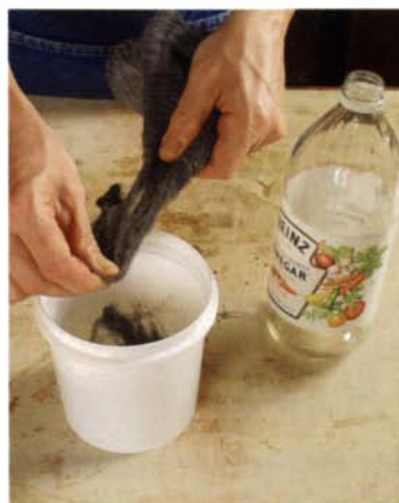
Iron buff. Shred a pad of steel wool into a pint of white vinegar. The solution turns some woods black.
