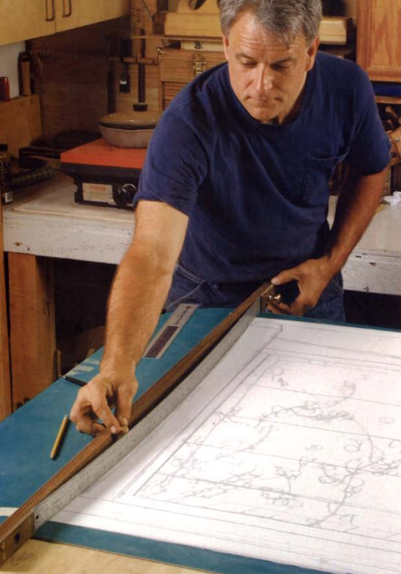
Adjustable jig for fair curves. Schürch designed this pinch fairing jig to create fair curves when drawing full-size furniture plans.
