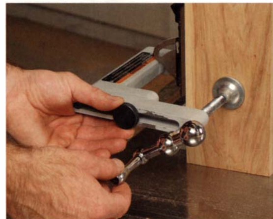
Knob makes adjustments easier. When wide stock dictates that the clamp arm has to be slid forward, Purdy preferred the jigs that locked the arm with a knob (shown) over those that called for an Allen wrench.
