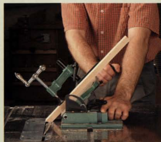
Side-tilt adjustment. The jigs have a main fence that can be tilted left up to 18°, 24°, or 45°, depending on the manufacturer.
