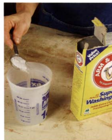
Sodium carbonate. Available as washing soda, this chemical mimics the effects of age.
