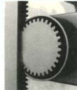
Rack & Pinion Drive
