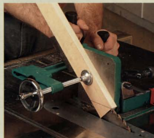
Front-to-back tilt adjustment. Using the secondary fence, each jig allows the workpiece to tilt backward up to 45°.
