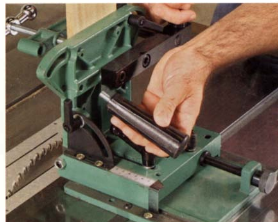
Adjustable handle. Most of the jigs offer at least one alternate handle position.
