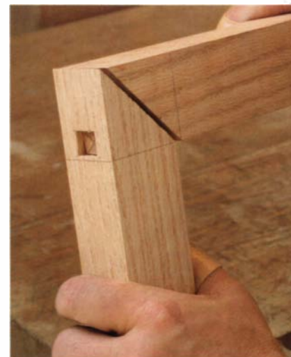
Finish the mitered faces with a chisel. Pare away the small step left behind from sawing.
