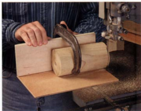
Solid support for round stock. For a safe cut, clamp round stock in an L-shaped sled that's screwed to a miter gauge. For stability, be sure the clamp sits below the stock's centerline.
