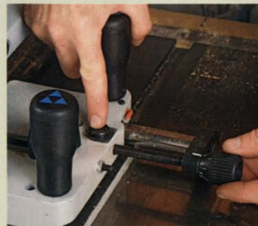
Side-to-side adjustment. When it came to establishing the tenon width, the Delta proved easiest to use—just push a release button, slide the main fence sideways, and then fine-tune the location with the micro-adjustment dial.
