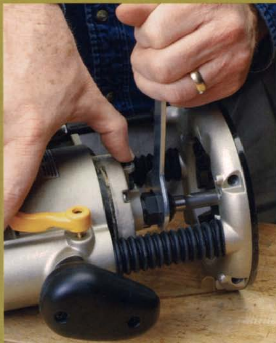
Best for bit changing. Lots of open space around the collet and a one-wrench changing system made the Ryobi a favorite when it came to removing or replacing a bit in either plunge or fixed mode.
