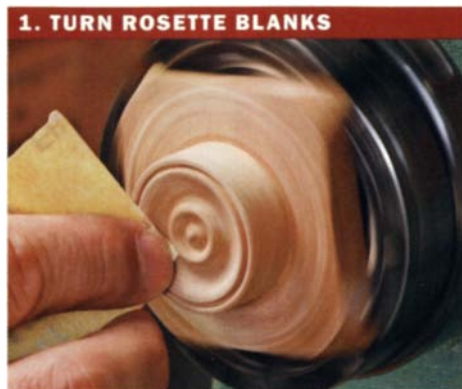
1. TURN ROSETTE BLANKS Rosette blanks turned on a lathe have a limitless number of profile and size possibilities.
