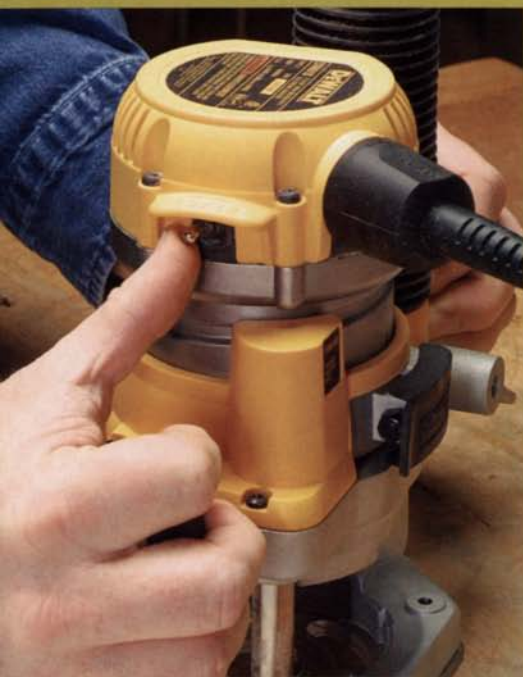
Sweet switch. A conveniently located toggle switch on the DeWalt allows you to keep both hands on the handles when turning the router on or off in plunge or fixed mode.
