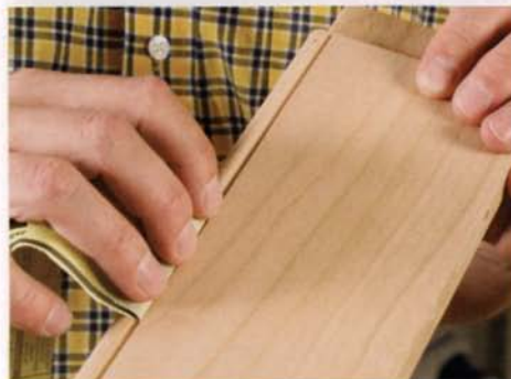
Sanding curves by hand. Contour the paper to fit curves in the wood.
