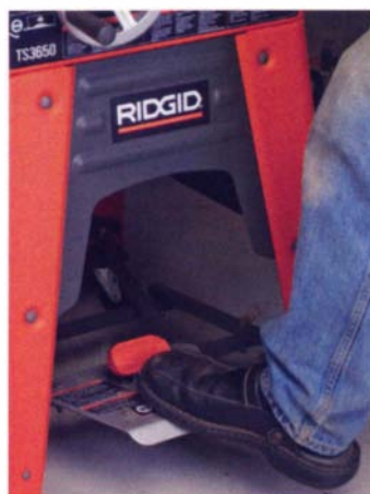
Retractable casters. A foot pedal controls a scissors lift that activates four retractable rubber wheels.
