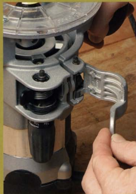
A lock for the bases. The oversize lever on Porter-Cable's fixed and plunge bases helped make it easy to lock the motor in each base.
