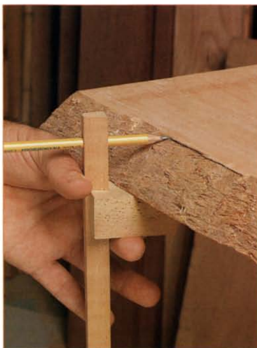
Scribe \frac{1}{16} in. over final thickness. Pick a show face and scribe from the bottom of the plank for your final passes with the power planer. Hare uses a shopmade marking gauge to work around live edges.
