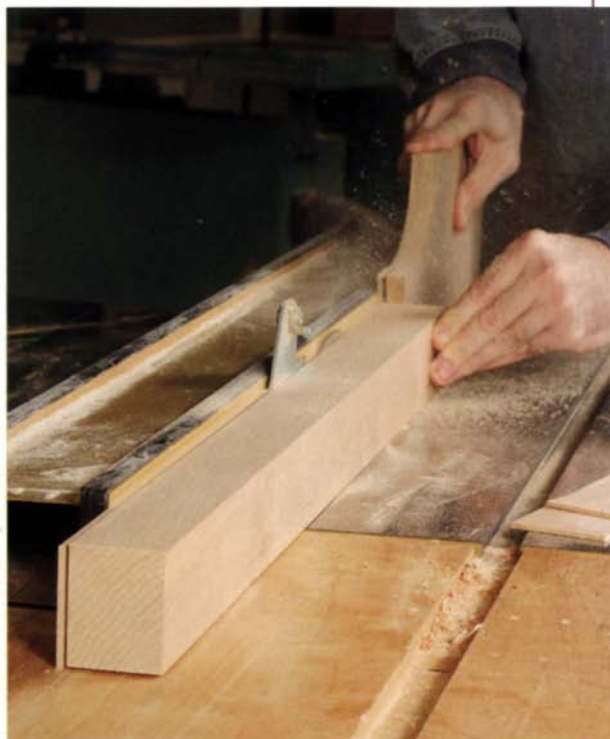
A push stick for ripping thin stock. A beveled front end on this push stick keeps the back end of the workpiece from rising up during the cut.
