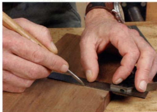
Thin marking lines yield accurate measurements. A marking knife can offer a precise line to measure to and from. Avoid thick pencil lines.
