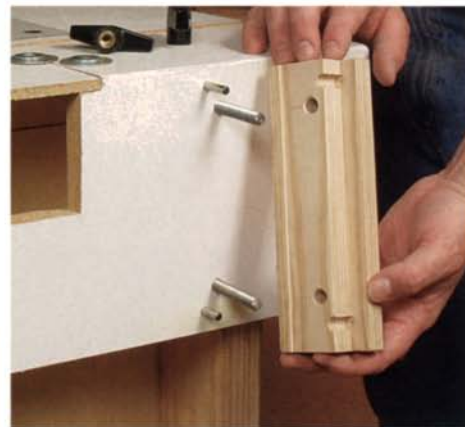
Clamp blocks secure the adjustable carriage. The clamp blocks fit over the carriage bolts and steel dowels and are tightened in place with threaded handles.
