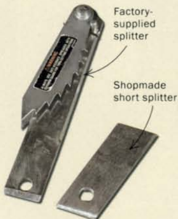
Make your own splitters for special tasks. Cut steel bar stock, drill a hole for the fastening bolt, and file the leading edge of the splitter to a bevel.
