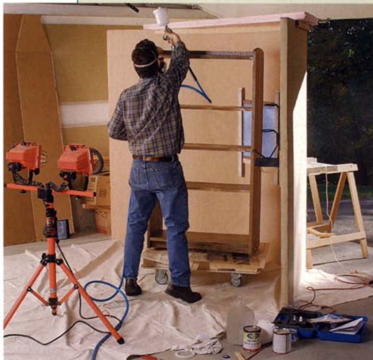
Garage spray booth. The spray booth fits into a garage-door opening, and a box fan draws some of the overspray into the filter and fumes into the open air.
