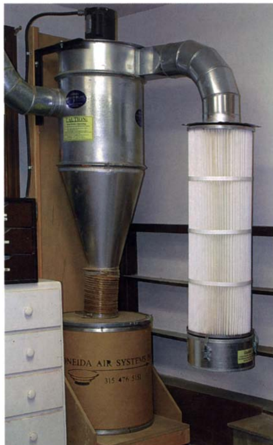
No disassembly required. The exposed filter on the Oneida Air Systems cyclone is cleaned with a blast of compressed air. Dust settles into a removable dustpan.
