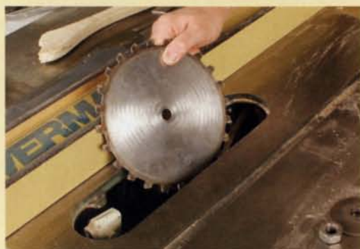
Use a dado blade for the first cut. For 10-in. tablesaws, an 8-in. dado blade sits far enough below the new uncut insert that it won't contact the insert when the saw is turned on.
