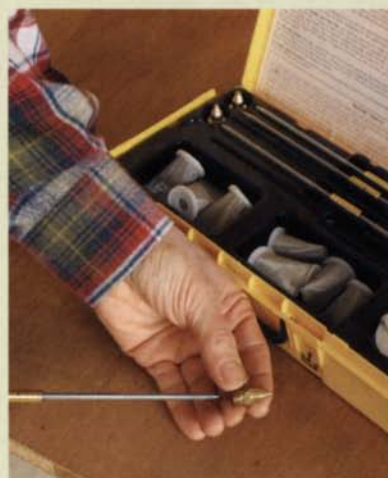
Choose the right-size needle/ nozzle. The higher the viscosity of the finish, the larger the needle/ nozzle to achieve good atomization.
