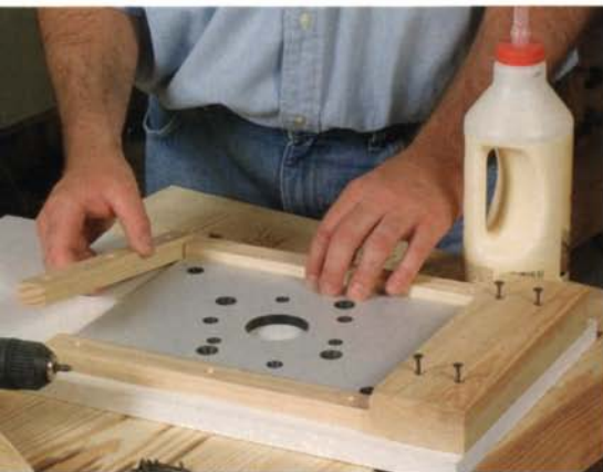
A frame on the back of the adjustable carriage holds a router baseplate. The frame supports a horizontally mounted router. The upper rail also supports overhead attachments.
