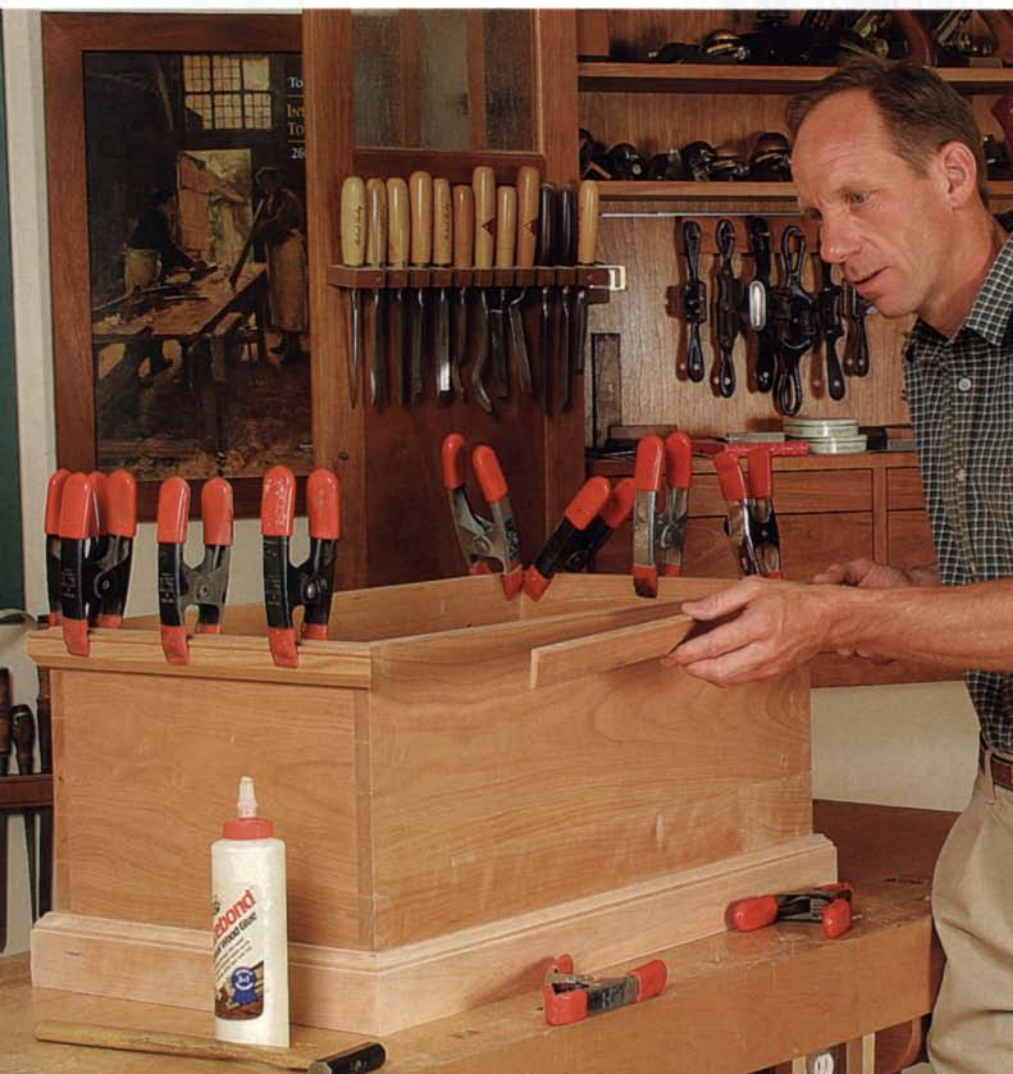
Glue the top molding. Later, after the hardware has been installed, nail the molding with finish nails to add additional holding power.
