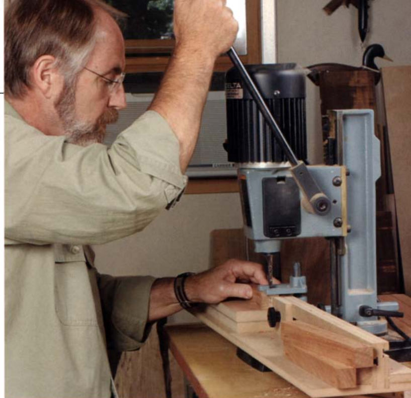
Accurate mortises with one setup. Take your time when setting up the hollow-chisel mortiser. One fence setting can be used to cut all of the mortises in the table.
