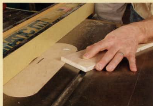
Clamp the insert in place with the saw fence. Position the fence over one edge of the insert and clamp it in place. Hold a piece of scrap over the other edge as you raise the blade into the new insert.
