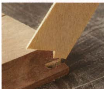
A push stick that locks in place. Although he usually prefers larger, paddle-style push sticks, Latta occasionally uses a thin one shaped on the bottom to lock in place with a matching kerf.
