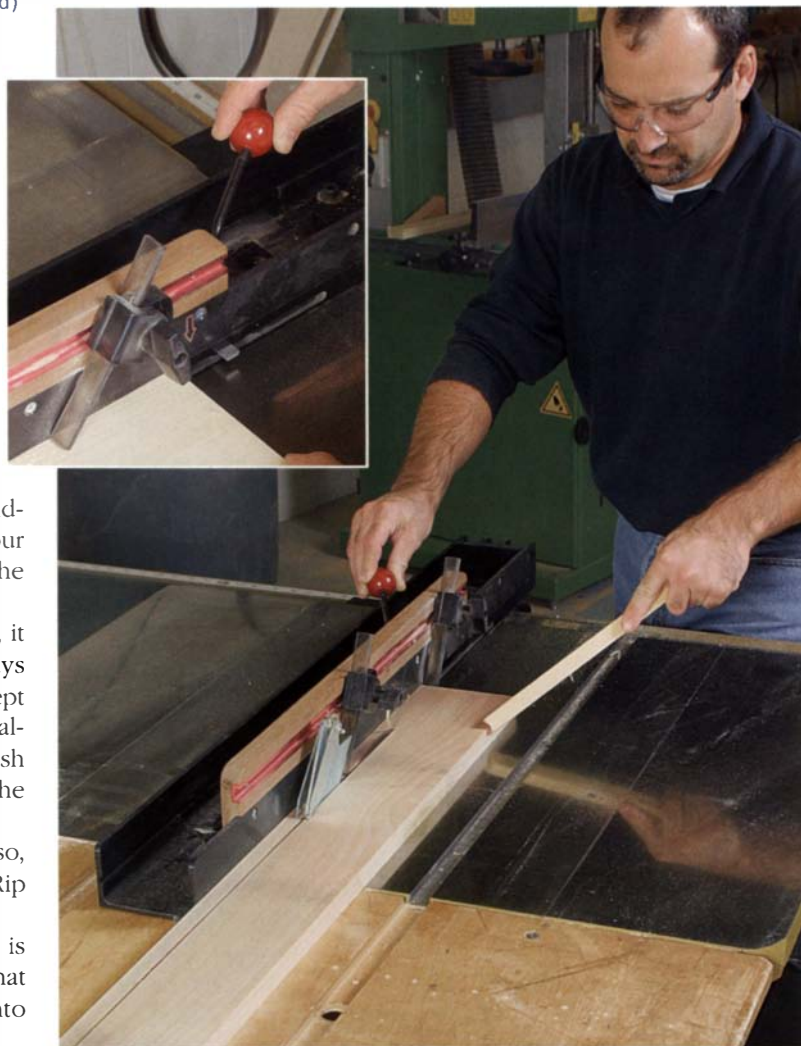
Rip fence helps keep fingers away from the blade. The WondeRip uses a lever attached to an aluminum finger to push narrow parts through the blade. The operator's notched stick helps hold the stock against the fence.
