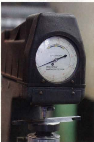
Tempering improves toughness. After quenching, the O1 steel is reheated to a temperature below the red-hot stage, which decreases hardness and increases toughness. The hardness of the blade, destined for a spokeshave made by Woodjoy Tools, is checked on a Rockwell-hardness tester (right).
