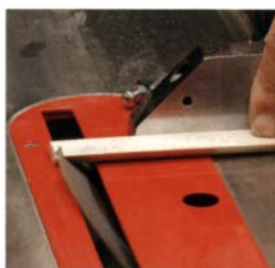
Cut the tenons from a long strip of material. Cut a bevel along one edge of the tenon stock. Then bevel one end and crosscut to length.
