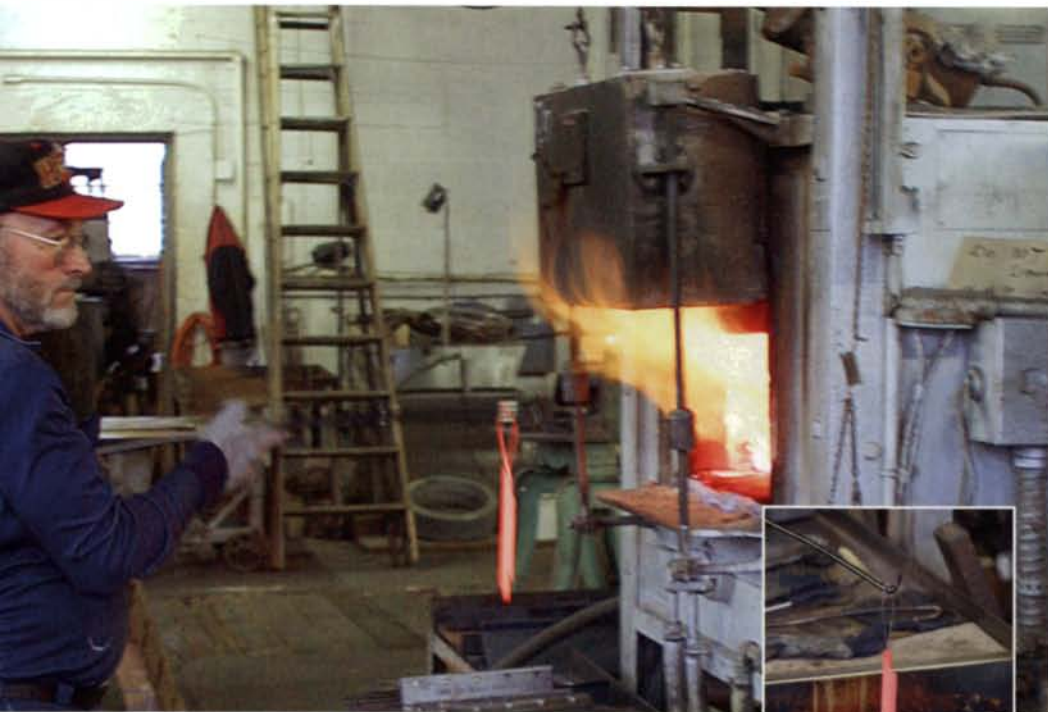
The hardening process. At Rhode Island Heat Treating in Providence, a glowing, red-hot O1 steel spokeshave blade is removed from a furnace, then quickly quenched (cooled) by dipping the steel in a bath of oil (inset).
