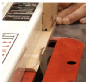
Cut the tenons from a long strip of material. Cut a bevel along one edge of the tenon stock. Then bevel one end and crosscut to length.
