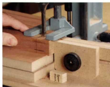
Remove the spacer block to cut the other end of the mortise. Once both ends of the mortise have been cut, nibble away at the remaining material.
