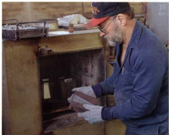
Tempering improves toughness. After quenching, the O1 steel is reheated to a temperature below the red-hot stage, which decreases hardness and increases toughness. The hardness of the blade, destined for a spokeshave made by Woodjoy Tools, is checked on a Rockwell-hardness tester (right).
