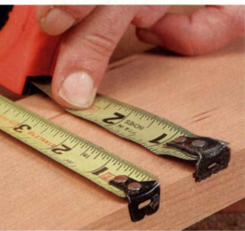
Start with a good tape measure. A bent hook or a twisted tape can cause measuring mistakes.
