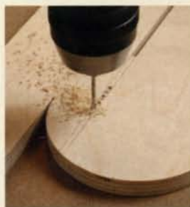
Drill the mortise. Using a fence on a drill press, drill \frac{3}{32} -in. holes in line with the blade kerf. Clean up the mortise with a chisel, and glue in the splitter.
