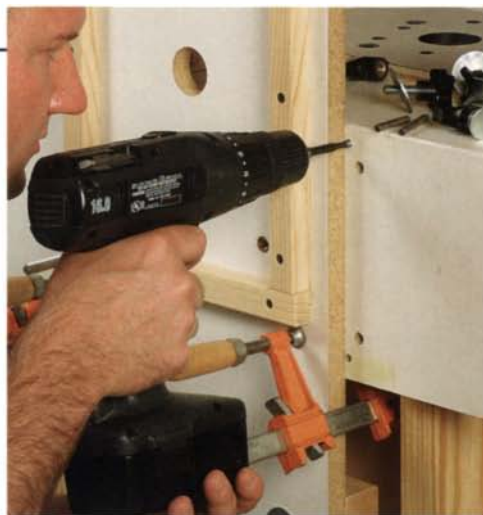
Mount the adjustable carriage to the table. Clamp the carriage in place so that it sits perpendicular to the tabletop. Drill holes for carriage bolts and steel dowels.
