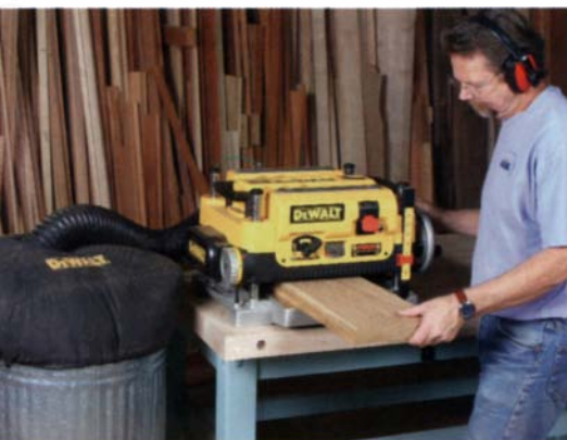
Built-in chip collection. The optional system, consisting of a hose and a trash-can fabric collar, did a good job collecting chips.
