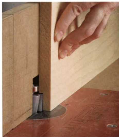
Rabbeting-bit set has extra cutting length. With an uncommonly long 1-in. cutter, plus seven different bearings, this set can make rabbets of varying lengths and widths.
