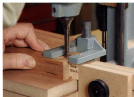
Accurate mortises with one setup. Take your time when setting up the hollow-chisel mortiser. One fence setting can be used to cut all of the mortises in the table.
