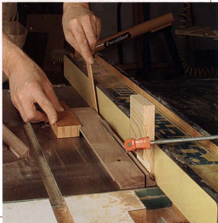
A push stick that locks in place. Although he usually prefers larger, paddle-style push sticks, Latta occasionally uses a thin one shaped on the bottom to lock in place with a matching kerf.
