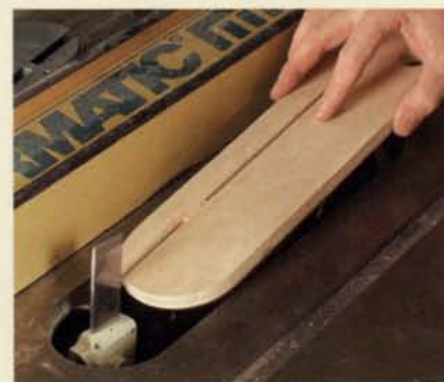
Make your own splitters for special tasks. Cut steel bar stock, drill a hole for the fastening bolt, and file the leading edge of the splitter to a bevel.
