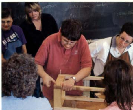
Hands-on instruction. Albert demonstrates how to pin a mortise-and-tenon.
