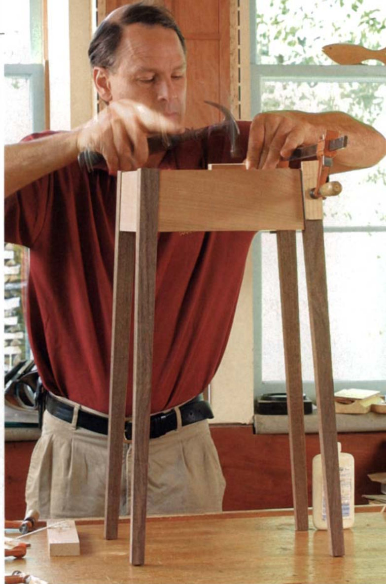
Glue in the front and rear aprons. Tap the aprons into their mortises with a hammer and block.
