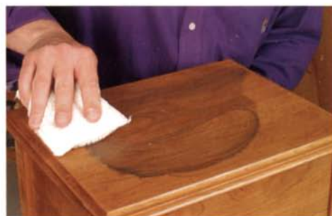
Rottenstone makes it glossy. Use a toweling sponge, available at auto stores, to rub the rottenstone in random patterns, bringing the whole surface to a uniform high gloss.
