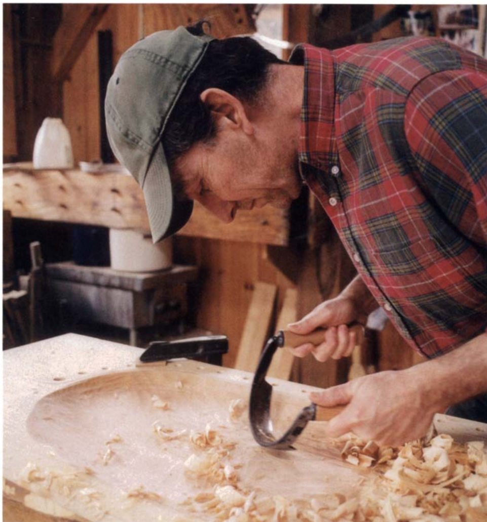
Big scorp does the job. With its added size and weight, plus good-quality steel, this new scorp from Barr Tools was a solid performer.
