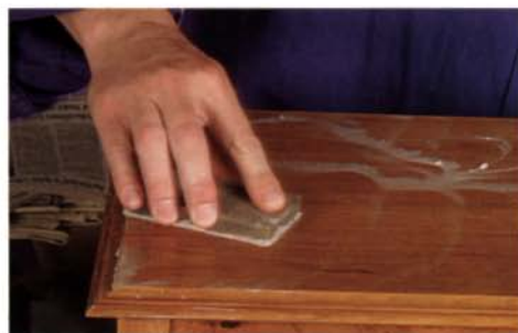
Random rubbing. Unlike the earlier sanding that was done with the grain, rub the pumice in random circles with a felt block.
