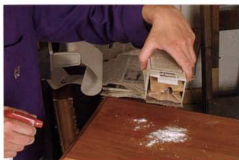
Pumice and water. Sprinkle pumice on the surface and spray it lightly with water in preparation for rubbing out the finish.
