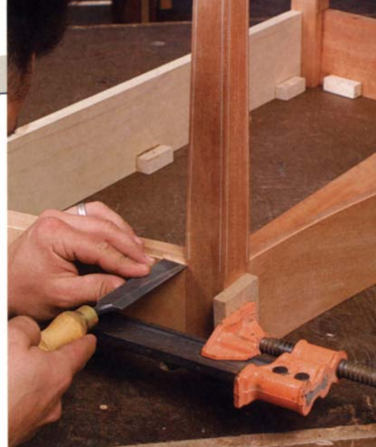
Transfer the banding locations from aprons to legs. Dry-fit the table, then use a wide chisel to carry over the layout marks.
