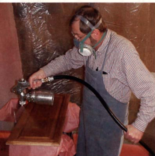
Turbine power. The HVLP sprayer from Turbinaire has plenty of power to spray any finish a woodworker is likely to use.
