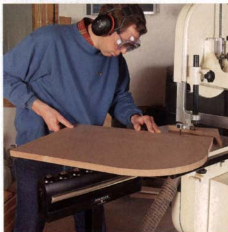
Moving around. Ball-bearing supports allow the workpiece to be moved in any direction, as when cutting curves on the bandsaw.
