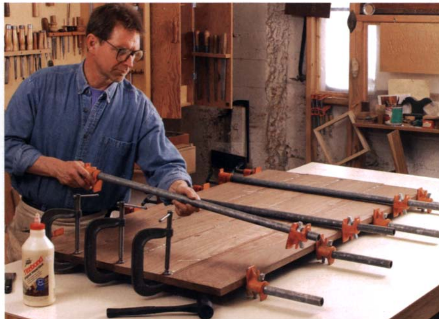
Add the top clamps. Placing clamps on top helps balance the clamping forces applied by the bottom clamps. If all of the clamps were mounted on only one side, the panel likely would buckle when the clamps were tightened.
