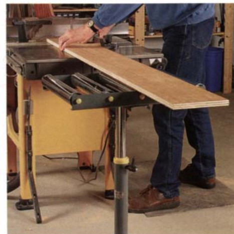
Rolling crosscut. Multiroller stands with their wide surfaces offer the best support when crosscutting on the table-saw.
