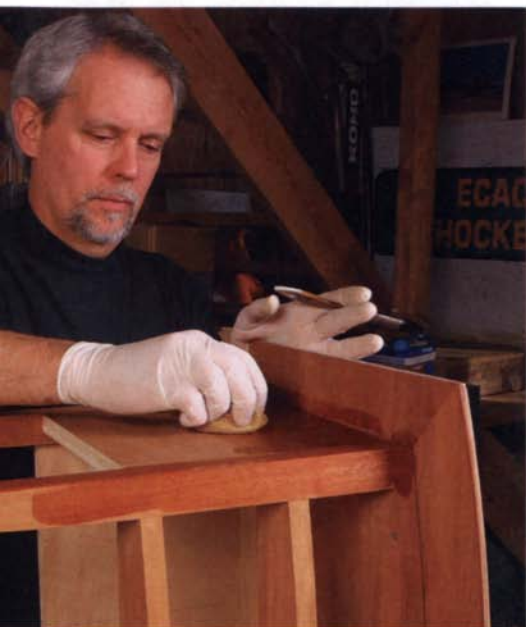
Padding prevents sags and runs. Gedrys applies shellac with a pad but uses a small brush to get finish into crevices and corners.
