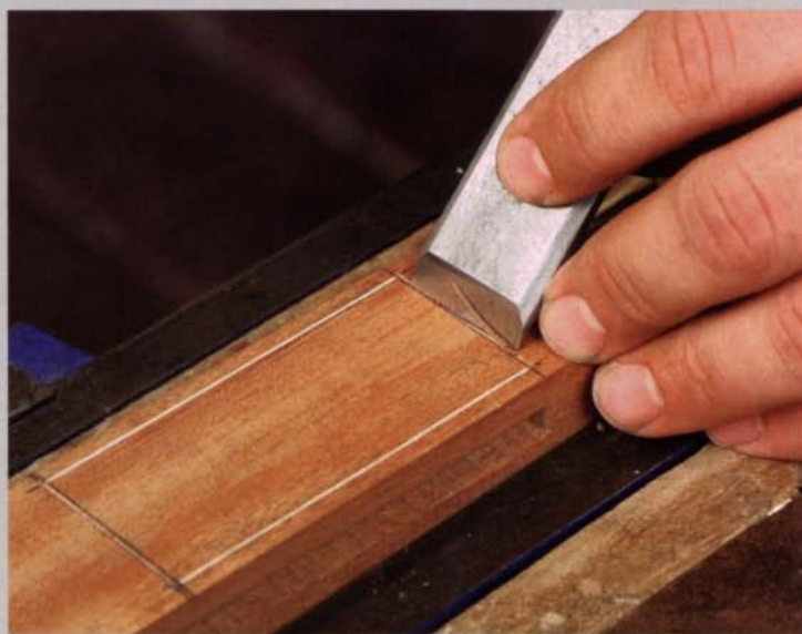
Cut the waste. Use a chisel to work from the center of the groove toward the scribed edges to remove most of the waste, a technique called ramp-cutting.
