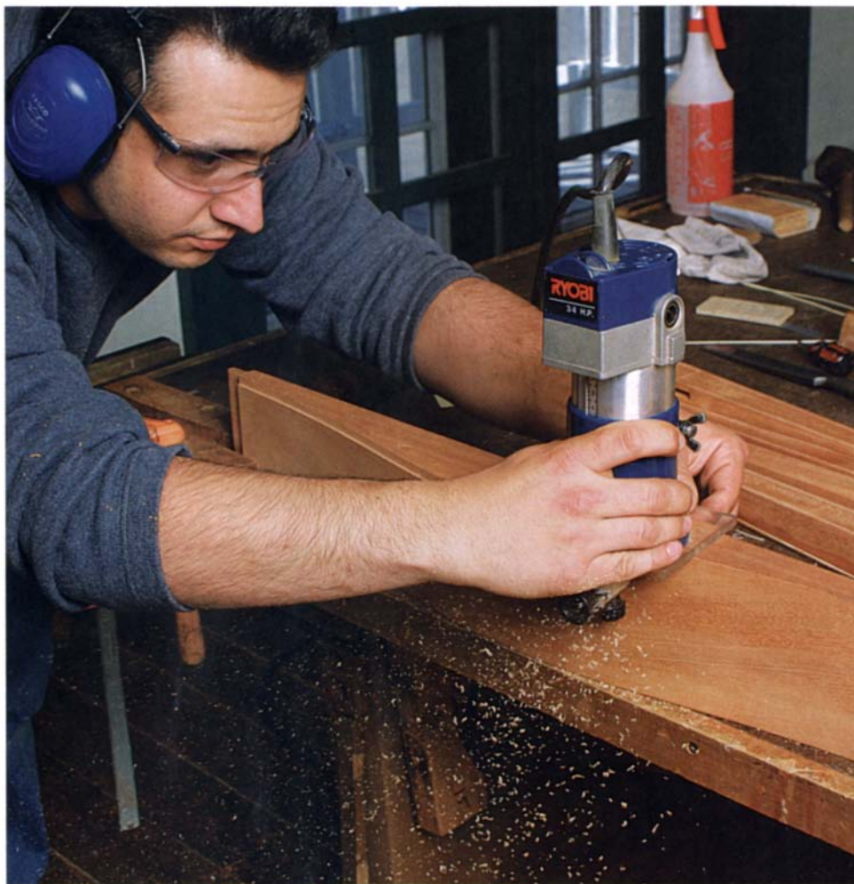
Cut the rabbets in the aprons. First, scribe the bottom edges of the rabbets to prevent router tearout. Then use a small router (above) with a single-bearing edge guide to follow the curve. Make test cuts in scrap to ensure that the banding will end up just proud of the surface.
