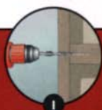
1 DRILL STEPPED PILOT HOLE
