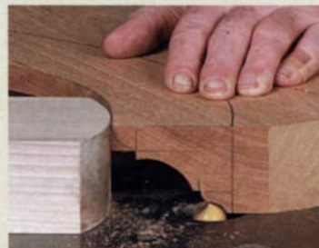
Cut the cyma recta. Start with a \frac{1}{4} -in.-radius roundover bit. Finish with a \frac{3}{4} -in. half-round (core-box) bit.
