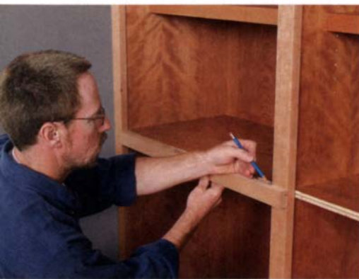
Fit the rails. Starting at the outside cabinets, mark and fit the upper and lower rails and the edging for the fixed shelf. Then move to the inside cabinets.
