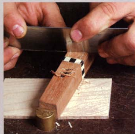
Level the cuff banding. Pare away most of the waste with a chisel, then scrape and sand the surfaces flush.
