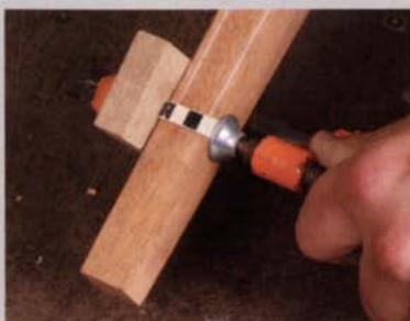
Glue in the last piece. Use masking tape or a small clamp to hold the banding in place. No banding is necessary on the back face.
