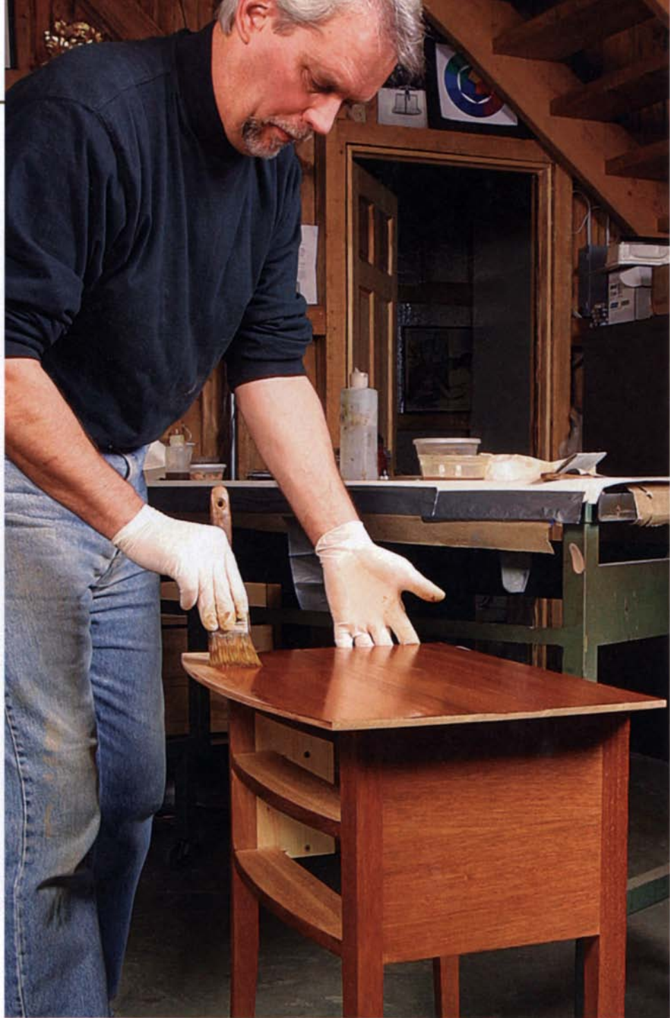
Brushing it on. Larger areas are easiest to finish with a brush. The larger capacity of a brush allows you to build up the thickness of a finish more quickly than using a pad.
