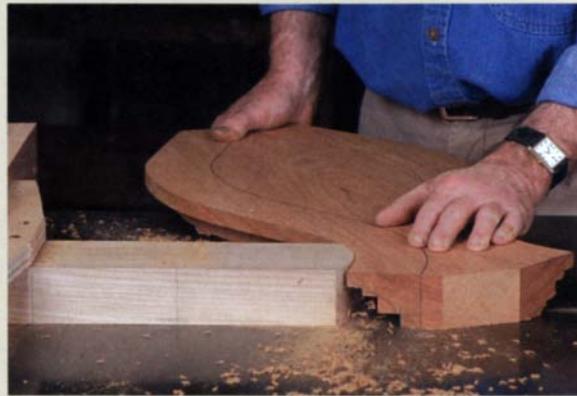
Start with a large 8/4 slab. Bandsaw the lower edges of both moldings from one slab, which provides a stable platform during routing.
