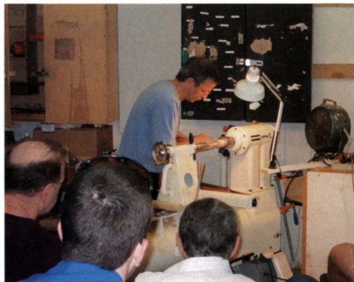
Down-to-earth demos. The exchange of ideas at the conference included many technical presentations. Here, Jean-Francois Escoulen demonstrates efficient spindle turning using a bedan.
