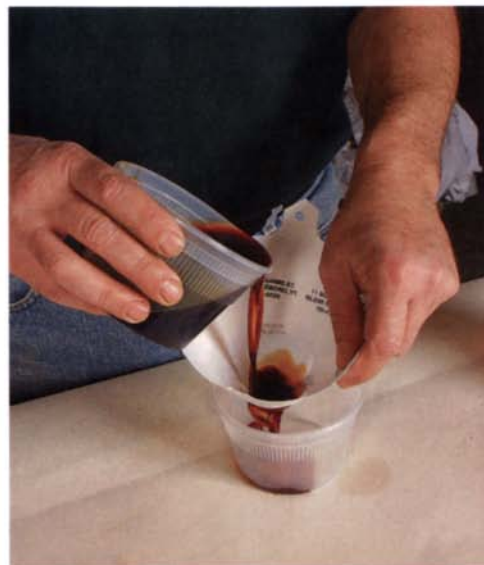
4 Strain the finish. After the shellac has dissolved, pour the fluid through a paint strainer to remove any impurities.
