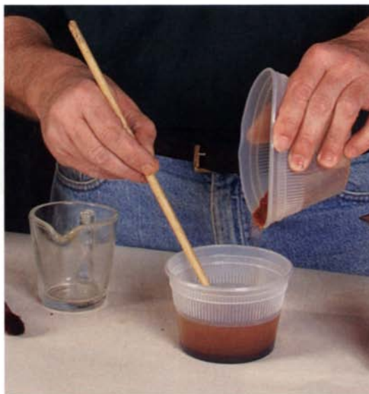
3 Dissolve the shellac. Stir the dry shellac into 8 liquid oz. of alcohol.
