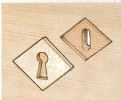
VENEER ESCUTCHEON Diamond or oval patterns can be cut from veneer and let into a mortise surrounding the keyhole.
