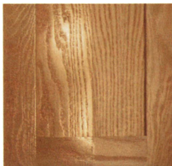
Spray gun vs. spray can. The left half of the panel received two coats of lacquer from a spray gun. The right half received two coats of lacquer from an aerosol can. The aerosol finish is only half as thick as the spray-gun finish.
