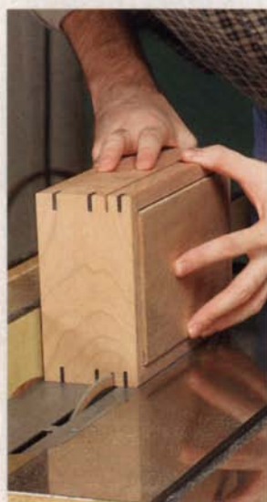
1. Through-cut. Set the tablesaw blade slightly higher than the thickness of the sides to cut through the two long sides.
