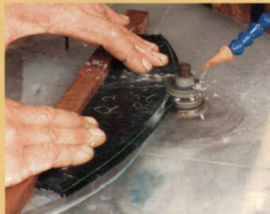
The stoneworker’s turn. Anderson mounted each template on a rough-cut stone blank and used a bearing-guided diamond bit in a router-table setup to create the bead. A jet of water kept the cutter cool.
