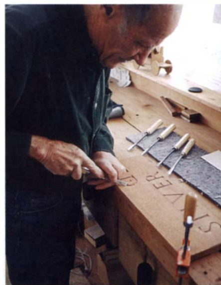
High-end carving tools. Lamp-brand carving tools take a nice edge, cut well and won't roll off the workbench.
