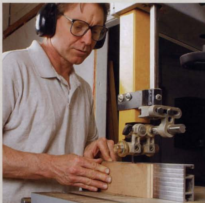
Sides resawn from thick stock on the bandsaw will produce a box with four matching corners.
