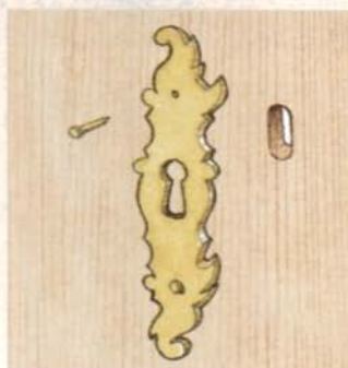
PLATE ESCUTCHEON Simple or intricate pieces of hardware simply can be nailed into place over the keyhole.
