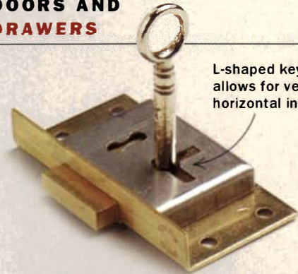
The lockset installed on this door is typical of those found on most 18th-century doors and drawers. It is mortised into the back of the door. A mortise in the opposing door or case captures the bolt.
