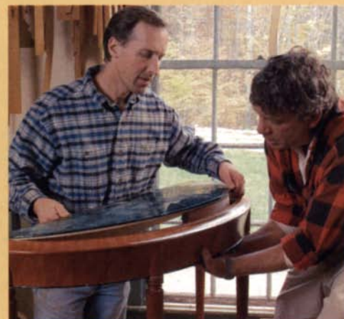
Attaching a stone tabletop. After laying on a coat of auto-body filler and running the tabletop slab through a wide-belt sander to create uniform thickness, Lamb and Anderson glued the blocks to the bottom of the slab with epoxy. The blocks, in turn, were screwed to the apron.
