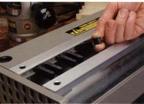
Locking fingers. The finger templates on the Akeda lock onto the jig's back rail, allowing for easy and precise adjustments.
