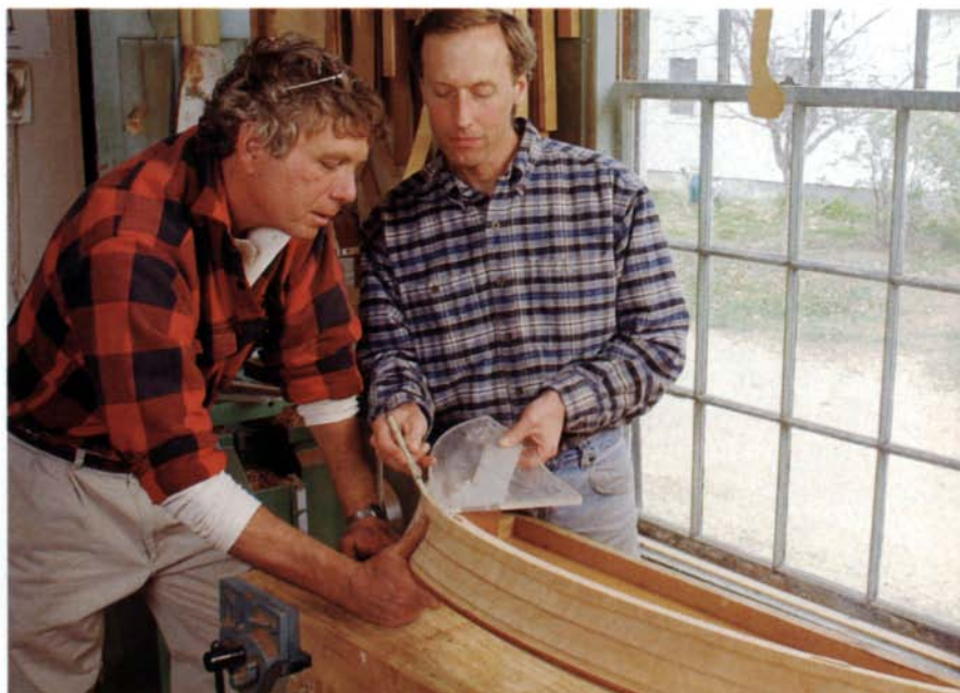
Templates are the key. For each section of beading, Lamb (right) made a plastic template directly from the elliptical table apron, and passed it on to Anderson (left).
