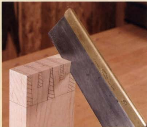
Cut the dovetails. Use a fine-toothed backsaw to cut the sides of the dovetails.
