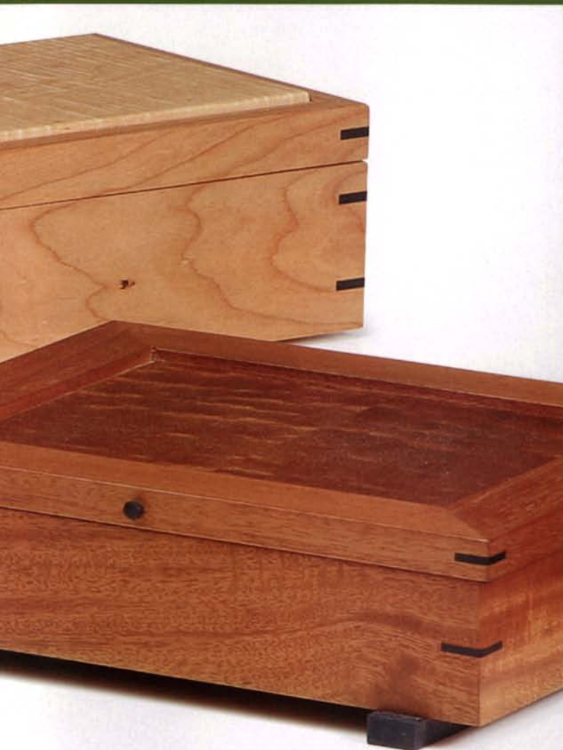
Sides resawn from thick stock on the bandsaw will produce a box with four matching corners.
