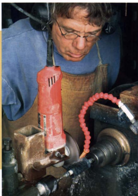
Precise pattern for the feet. Anderson used a turned wooden mock-up of a foot as a template. By mounting a right-angle grinder (armed with a diamond wheel) in the tool post of an old metal lathe, Anderson created a stone-turning machine.
