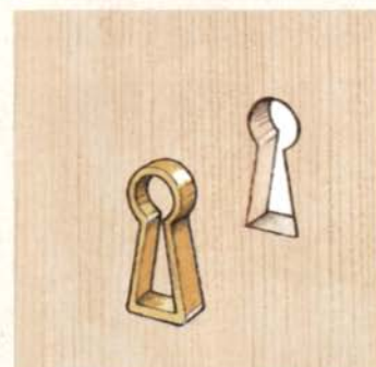
INSET ESCUTCHEON Another classic option is to inset a brass keyhole into the cutout for the key.
