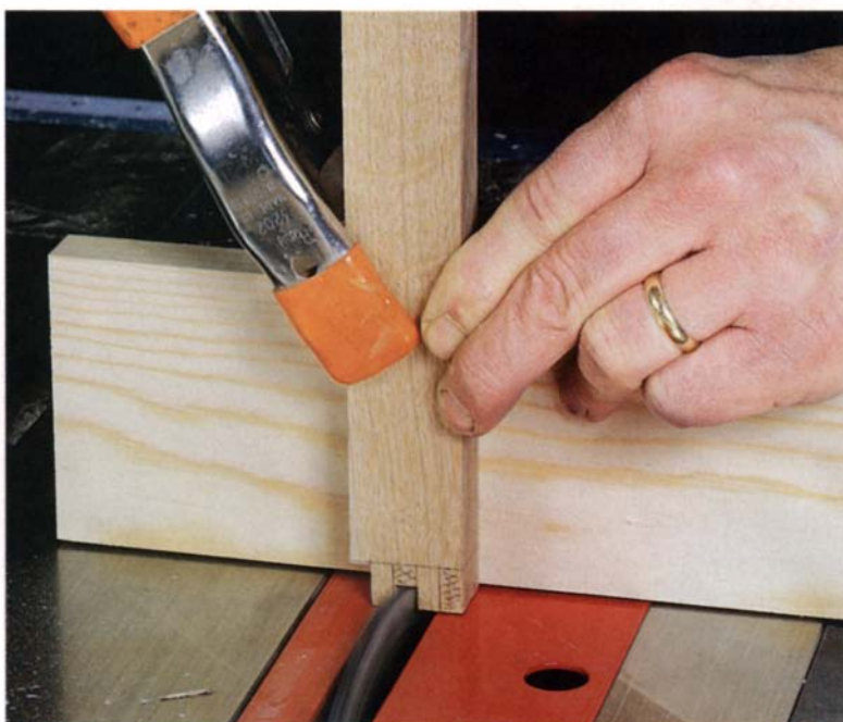
Use the mortises to lay out the tenons. Place the rail on the mortised leg and mark the locations of the tenons.
