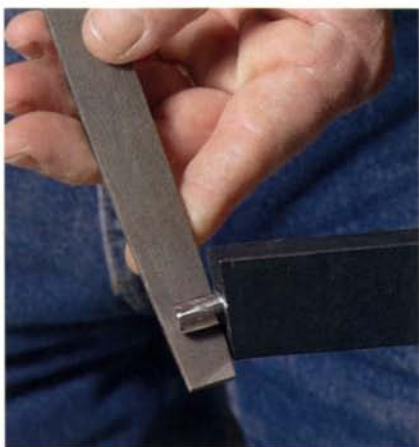
Steel tenons filed to fit. Gibson uses a mill file to shape the stretcher tenons to their final thickness.
