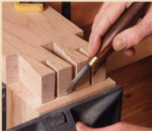
Mark the pin locations on the outside and inside ends. With the end cap clamped in a vise, the front piece is used as a template to mark the pin locations.
