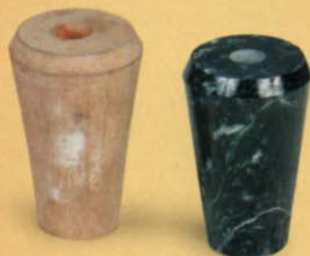
Precise pattern for the feet. Anderson used a turned wooden mock-up of a foot as a template. By mounting a right-angle grinder (armed with a diamond wheel) in the tool post of an old metal lathe, Anderson created a stone-turning machine.
