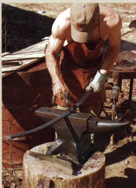
Texturing the stretcher. Blacksmith Ben Gibson uses a ball-peen hammer to create a dimpled texture in the stretcher.
