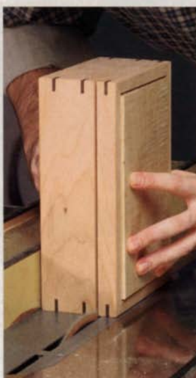
2. Partial cut. Lower the blade to leave \frac{1}{16} in. of wood on the short sides. This alleviates clamping or supporting the lid with shims during the final cut.
