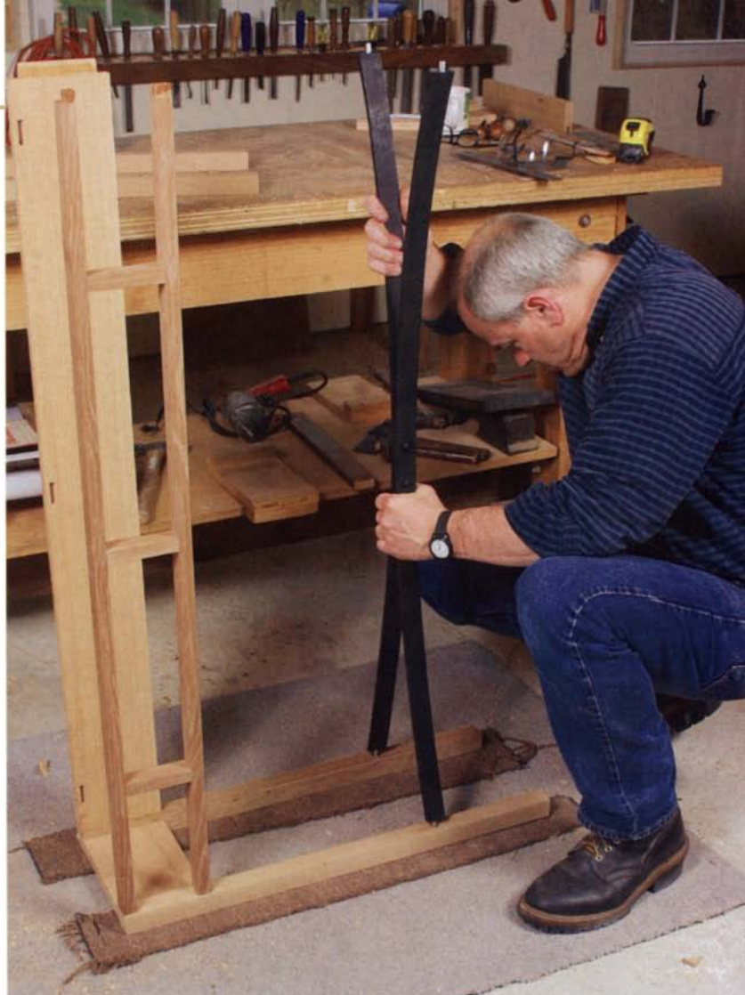
Steel tenons filed to fit. Gibson uses a mill file to shape the stretcher tenons to their final thickness.
