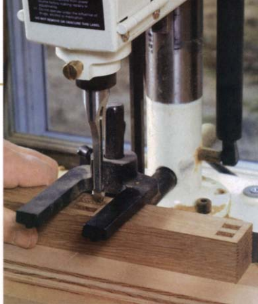
Mortise for double tenons. Using double tenons creates a stronger joint. To ensure consistency, cut all of the mortises at the same time.
