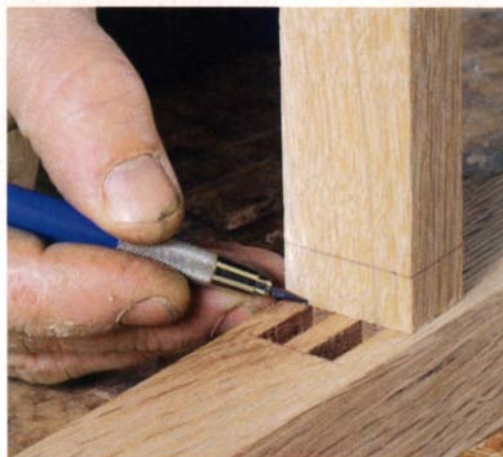
Use the mortises to lay out the tenons. Place the rail on the mortised leg and mark the locations of the tenons.
