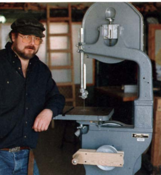
Hand-cranked bandsaw. Woodshop teacher Rocky Steirs converted a bandsaw from electric-powered to hand-powered to comply with school liability restraints.
