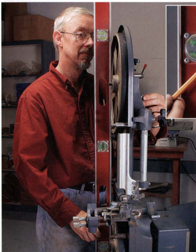
Check the alignment. Begin by placing a long straightedge (White uses a 4-ft. level) across both wheels. Then adjust the tracking mechanism to bring the upper wheel parallel to the straightedge.
