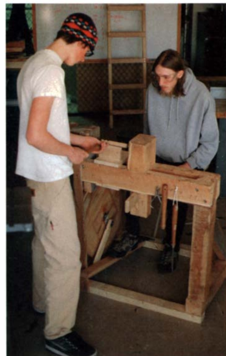
Back to the future. Two students operate a treadle lathe built by Steirs using his knowledge of Colonial-era metalworking.
