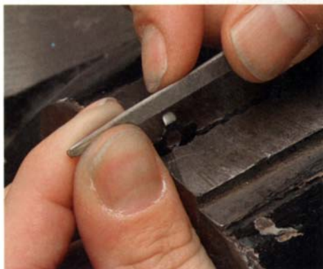
File a thumbnail. If the nicker edge is worn, refile it into a thumbnail shape.
