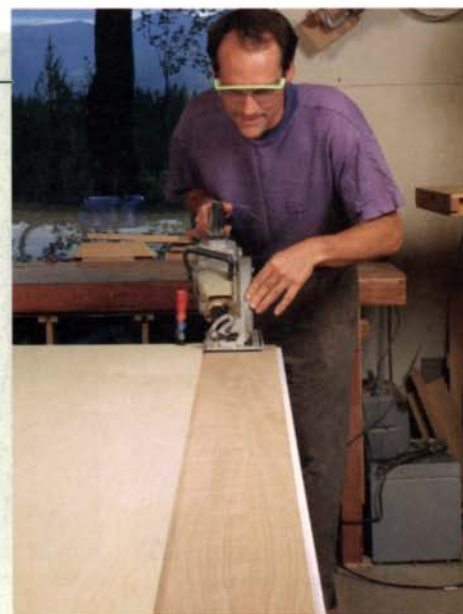
Cutting a plywood sheet. A second sheet of plywood (top) makes a serviceable edge guide for rough-cutting large sheets.
