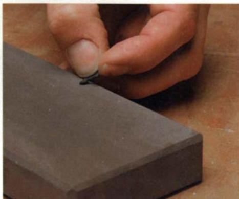
Hone until it's sharp. Using a sweeping motion with your hand, hone the nicker on a fine-grit stone or 220-grit sandpaper.
