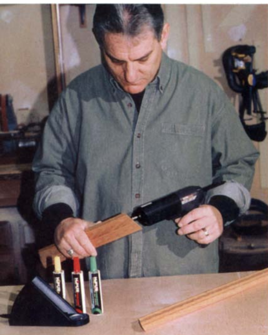
Hot glue is hot stuff. Titebond's quick-setting system is handy for gluing small, hard-to-clamp parts, such as moldings and miters.
