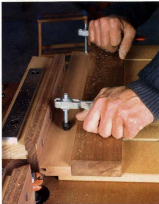
Cutting profiles. Warner uses this long-grain sled when routing profiles on long, narrow boards. The toggle clamps are safer and more effective than using fingers to guide the work this close to a cutter.
