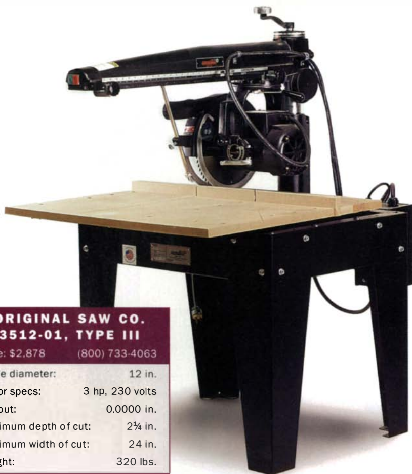
Two handles find the angle and keep it there. The lower handle keys into a notched collar, providing factory-set adjustments for square cuts and 45° miters. The handle at the top tightens the overhead arm onto the column.
