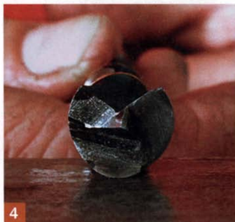
Hone the tip. Rotate the tip of the bit clockwise on the flat stone to hone the outside surfaces. Use a light touch here.
