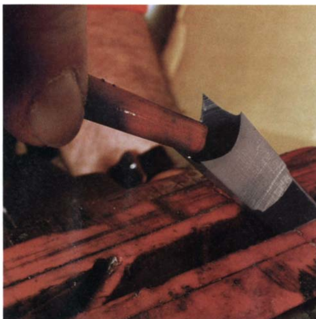
Sharpen the chisel bevel. To hone the beveled surfaces, use a fine-grit, round, tapered stone, rotating the stone as you work.
