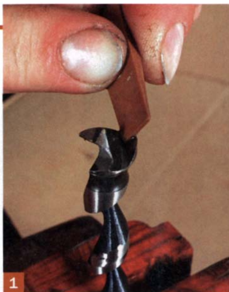
Start with the wing. A few short strokes with a fine-grit auger-bit stone sharpens the wing of the bit.
