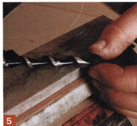
Hone the flutes. The flutes of the bit can be smoothed by rotating the bit counterclockwise on a flat stone.
