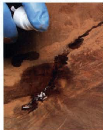
Pack, fill, spray. Fill the gap with sawdust using a wedge of wood to pack it down (left). Add several drops of cyanoacrylate glue (middle), then spray accelerant on top of that (right). The accelerant hardens the glue instantly, making it ready to be worked.
