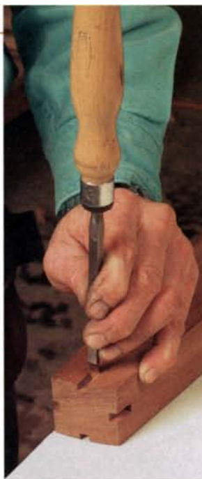
When routing the grooves, use a stop block. The tip of the post is angled, so you must reset the stop for each groove. Square the ends of the grooves with a mortising chisel (right).
