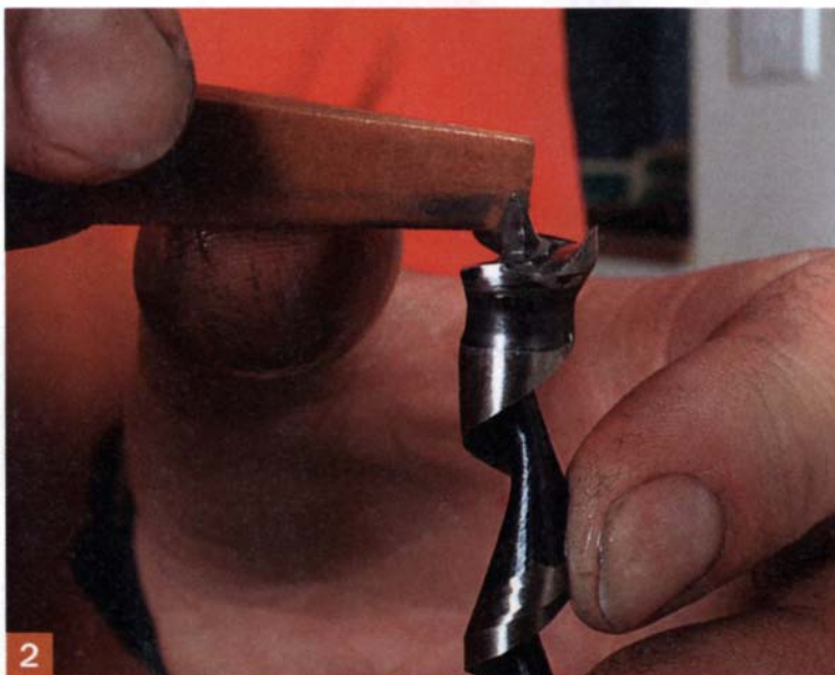
Start with the wing. A few short strokes with a fine-grit auger-bit stone sharpens the wing of the bit.
