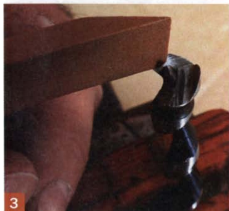
On the edge. When sharpening the cutting edge, pull the stone in one direction, working from the leading edge to the trailing edge.
