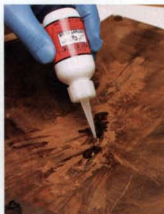
Pack, fill, spray. Fill the gap with sawdust using a wedge of wood to pack it down (left). Add several drops of cyanoacrylate glue (middle), then spray accelerant on top of that (right). The accelerant hardens the glue instantly, making it ready to be worked.
