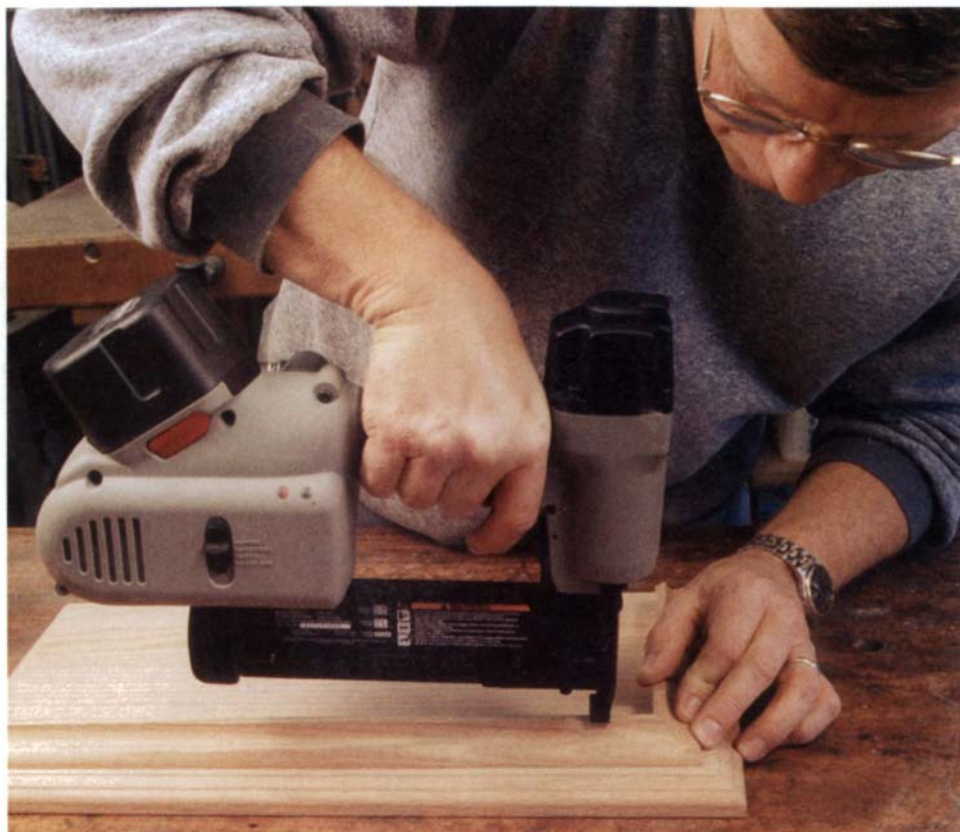
Minicompressor maximizes convenience. Equipped with a rechargeable battery that powers a small, built-in compressor, this brad nailer is truly portable. But it's not for 98-lb. weaklings.
