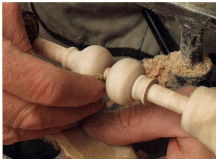
Don't be ashamed to sand your work. Particularly with curly wood, some tearout is inevitable and is easily removed by sanding.
