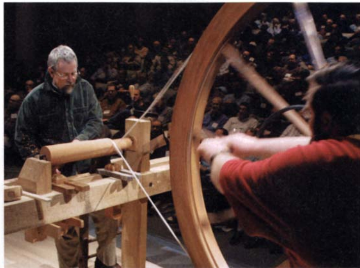
Human power. A member of the audience supplied the power to the lathe (above) while Phil Lowe turned the pedestal of a tea table.
