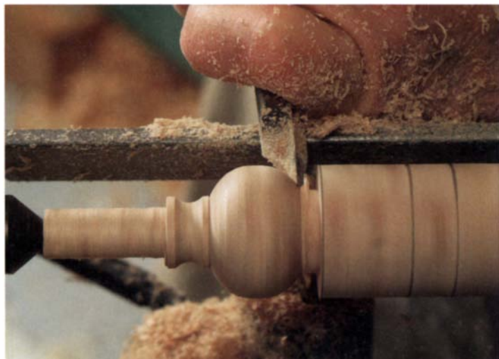
Worry-free beads. With the depth of the bead already defined on both sides by the V-parting tool, round over the sides of the bead with a series of light cuts.
