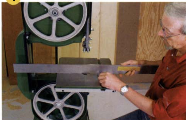
Using a straightedge and feeler gauge, we were able to check each of the tables for flatness.
