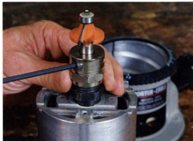
Quick bit switch. Bit changes are easy with the Eliminator RC collet, which requires only one Allen wrench to release the cutter.
