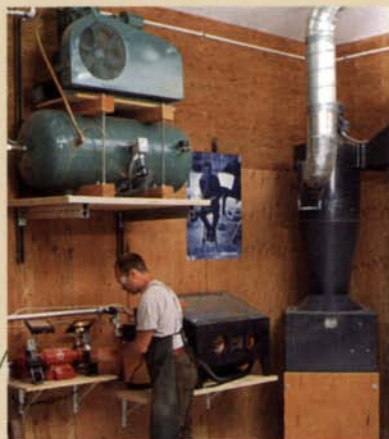
The air compressor rests on an industrial-strength shelf along one wall. Below, the floor space is utilized for a more practical application, in this case a sharpening station.
