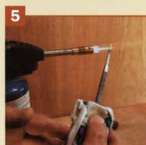
Attach a handle. Drill a stepped hole in the handle and heat the tang. The hot metal will burn its way into the hole for a tight fit.
