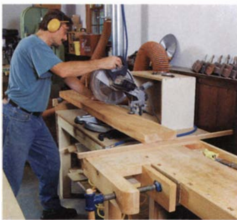
Sawdust is captured by a box, which is connected to the dust collector. A roller bolted to the left of the table provides stock support. The workbench (with the aid of a piece of scrap) provides support to the right of the chopsaw.
