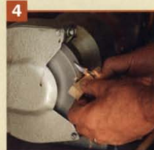
Grind the chisel tip. A tool rest helps at this point to establish an even bevel. Use a light touch when grinding, and cool the tool often.
