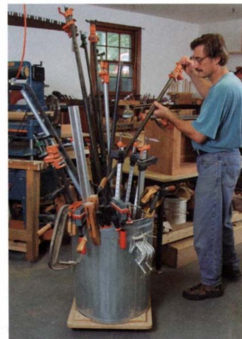
Clamps to go. Stored in a metal trash can, clamps can be wheeled to the assembly area, then rolled into an out-of-the way corner when not needed.
