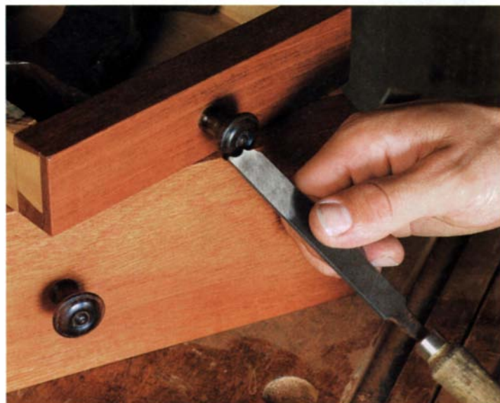
Philip C. Lowe teaches his students to make this custom scraper for decorating the knobs on a tool chest.
