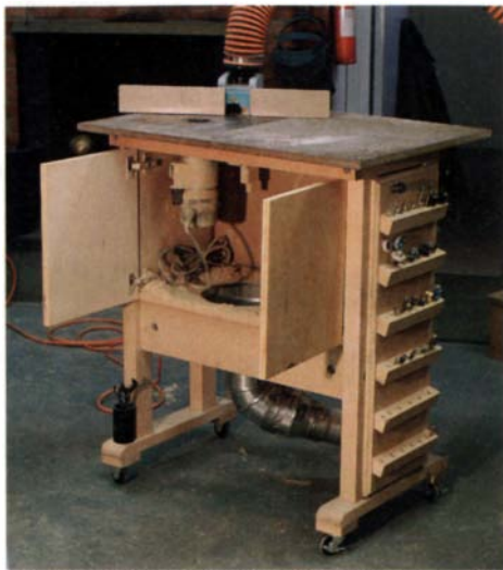
Traveling router cabinet. Dust collection is provided below, via a 10-in. to 5-in. reducer, and above, via a 2½-in.-dia. hose connected to the fence. The table is big enough to add another router if needed.
