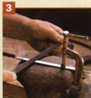
Smooth the surfaces with a file. A normal file will cut your tool blank, which has been softened slightly.
