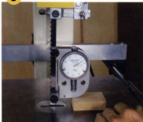
A tension gauge was used to measure the tension on the blades when the scale on the saw was set to the \frac{3}{4} -in. mark.
