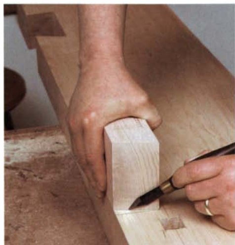
After angling the sides of the threaded blocks, lay out their recesses. The trapezoidal shape gives mechanical strength to this joint, which is also glued.
