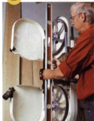
A long straightedge helped us find out if the wheels were in the same plane.
