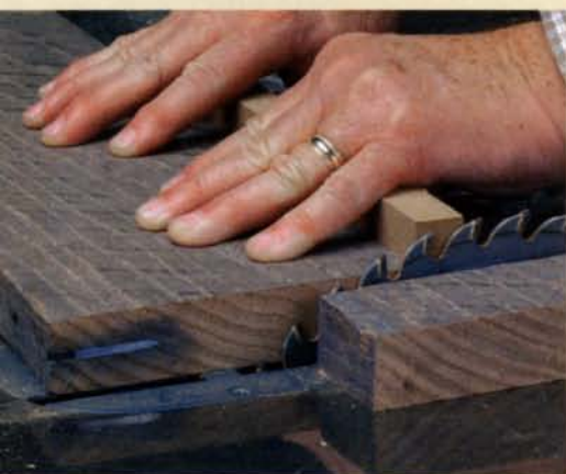
Cutting a nail. Not only does this damage a blade, but it can also send a very hot piece of metal into your saw cabinet.
