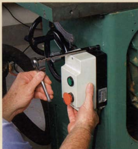
Remove the electrical box and clean out the dust. Also, remove all arbor adjustments and knobs to eliminate the possibility of someone picking up the machine by one of these elements.
