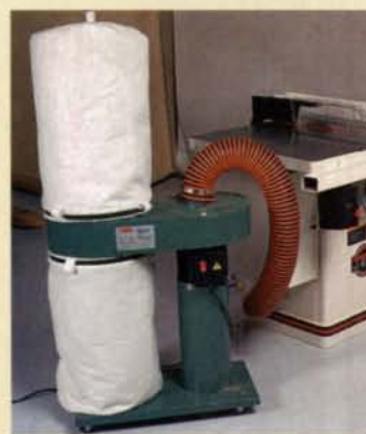
Sparks in the bag. Metal sucked into the dust collector's fan blade may cause a spark and ignite sawdust in the filter bag.
