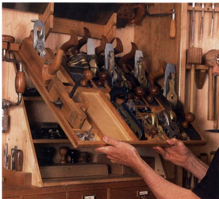
Planes within easy reach. Ledge strips locate planes on the shelf, and small pieces of leather are used to protect the blades.
