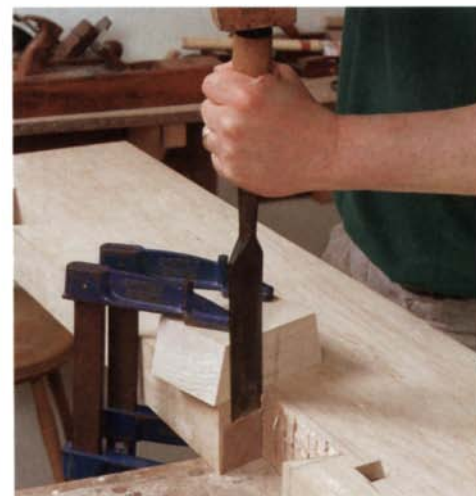
After chopping out the waste, pare the sides. Use one of the threaded blocks to guide your chisel.
