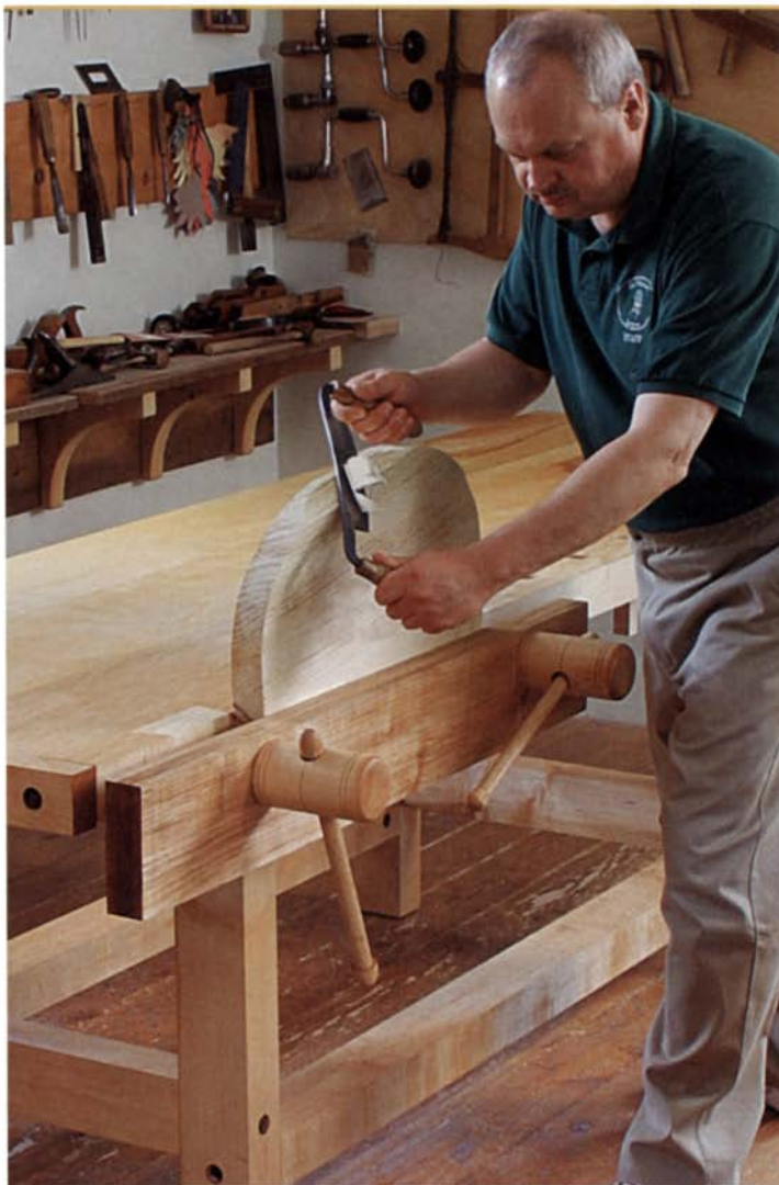
Size and strength. The thick wooden screws are far enough apart to accommodate a wide workpiece, and the jaw is long enough to support a 6-ft. board for edge-jointing.
