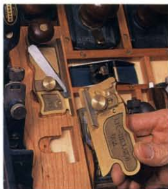
Fitting a tool. Odd-shaped tools, such as this side rabbet plane, fit into french cutouts in the shelf.
