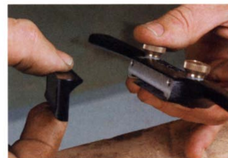
Removable toe piece. Removing a pair of machine screws separates the toe piece from the body of the spokeshave.
