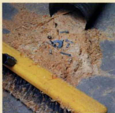
Metal in the dust pile. When cleaning shop, it's easy to sweep up screws, washers and nails. Dust from the floor should be sifted by hand, before it's introduced into a dust-collection system.
