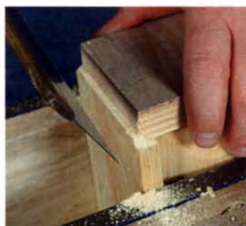
Saw a cutout for the bead strip. All four sides of the drawer fronts must be cut back to fit the cock beading. Cut each end of the drawer with a backsaw and plane the top and bottom to size.
