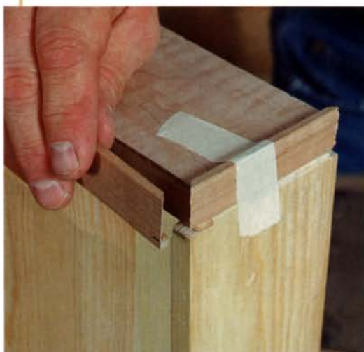
Tape clamps. Cock beading sits proud of the veneer by \frac{1}{8} in. Masking tape works like another set of hands to hold the cock beading in place while fitting the final pieces. After all of the pieces have been fitted, glue and clamp the cock beading in place.
