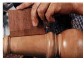
A custom straightedge. The knife-edge of a mitered block of scrap will reveal high and low spots that need to be evened out. Backlighting helps.
