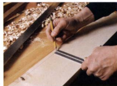
Use a straightedge to mark a parallel edge. Hold a pencil against the blade of a combination square, set to the desired width, and mark a line on the opposite side.
