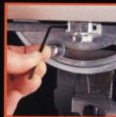
Fine tune micro-adjust trunnion.
