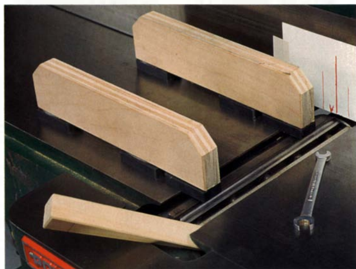
Bar magnets (available from hardware or electronics stores) glued to a block of wood (do this on a level surface) with silicone adhesive make a decent knife holder/straightedge. Tighten the bolts on the locking bar so that each knife (at top dead center) is level with the outfeed table.
