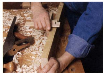
Marking gauge determines thickness. After one face of the board has been planed flat and smooth, run a marking-gauge fence along the finished side to mark the board's final thickness. Repeat the three-plane process on the rough, unfinished side.
