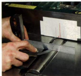
On many jointers, the outfeed table should be about 0.015 in. above the cutterhead.
