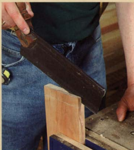
Saw both corners, then connect the cuts. Cutting through a tenon's long grain can be a problem unless you ease into it by making
