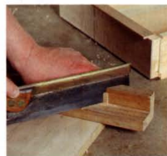
Miniature miter box for cock beading. Once the edges of the drawer front have been cut back, cut the cock beading with a backsaw and a small miter box.
