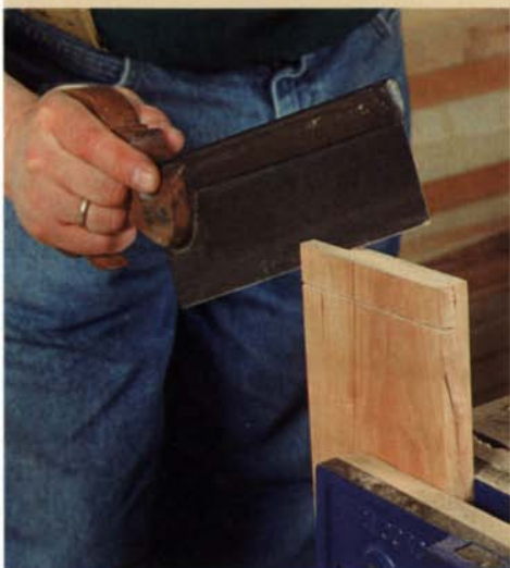
Saw both corners, then connect the cuts. Cutting through a tenon's long grain can be a problem unless you ease into it by making
