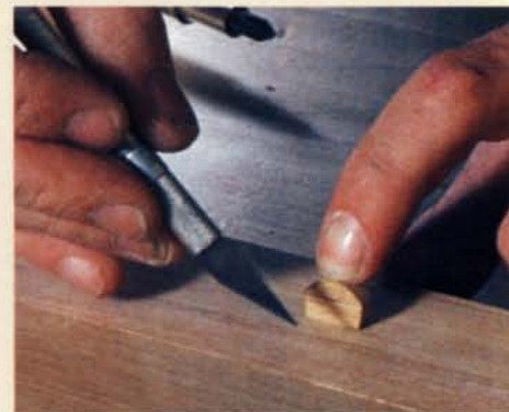
Doors with latches and elbow catches require a doorstop. Mortise the stop into the base of the case, keeping it centered.
