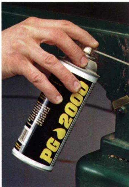
PG 2000 for sticky machines. The dry lubricant doesn't attract a lot of sawdust.
