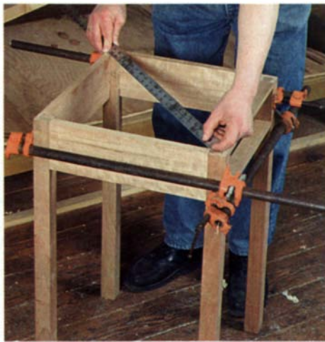
Ruler and square are invaluable. After the joints have been cut, dry-fit the table with clamps and take diagonal measurements across the top of the frame (left). Equal diagonal measurements indicate it is square. Check the rail-to-leg joints for square while the table is clamped but before the legs are tapered (below).
