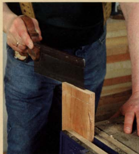
a diagonal cut through both corners and then connecting those cuts across the middle. Use the same process when cutting the shoulder.
