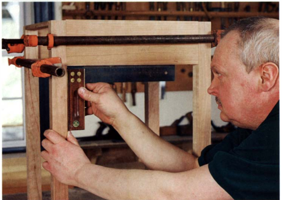
Ruler and square are invaluable. After the joints have been cut, dry-fit the table with clamps and take diagonal measurements across the top of the frame (left). Equal diagonal measurements indicate it is square. Check the rail-to-leg joints for square while the table is clamped but before the legs are tapered (below).
