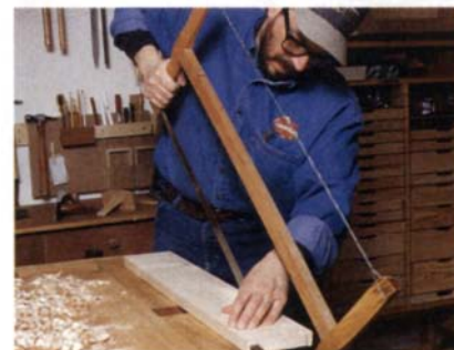
Bowsaw for ripping to final width. The saw's long blade makes it easy to take long strokes. Cut to within \frac{1}{16} in. of the marked line. Finish the sawn edge with a jointer plane.
