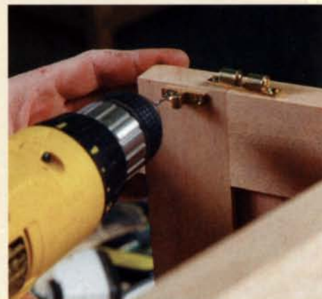
Temporary fastener. Double-sided tape on the male half will hold it in place on the door so that accurate pilot holes may be drilled.
