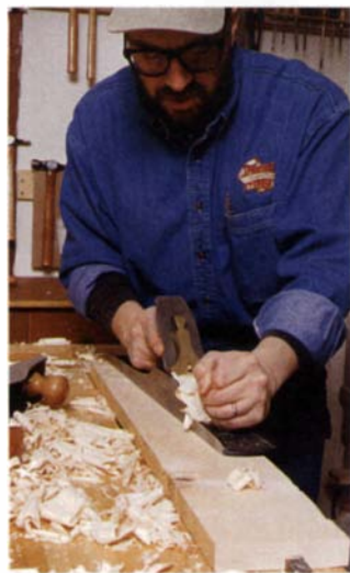
Jointer plane is the last one to use. With a long jointer plane, work the board with the grain, removing the marks left by the jack plane.
