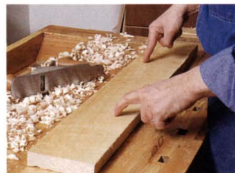
Check a board's flatness. Place your fingers on diagonal corners of the board. If the board rocks on the bench, move your fingers toward the center. When the board rocks no more, the high spot is between your hands.
