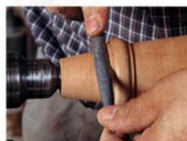
A fine rasp for delicate cuts. Truing a tapered foot to fit into a brass caster is a good job for this tool.
