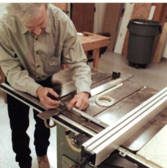
Measuring for parallelism. John White measured each fence at 1-ft. increments to check whether the fence was parallel to the saw blade. He clamped a straightedge to the table, locked the fence and then used a razor knife to mark the fence-to-straightedge distance on a piece of masking tape on a smaller straightedge. After measuring at the front and the rear of the fence, he used an inspection microscope to measure the distance between marks in thousandths of an inch (.000 in.).
