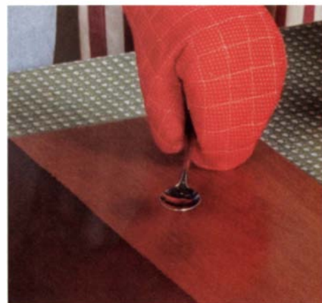
Hot-spoon test. Several finishes were marred when a hot spoon was allowed to cool on the panel.
