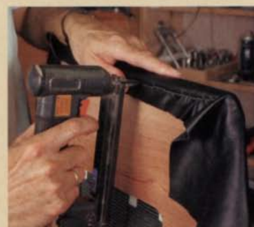
Fill in the border with staples. Stretch and staple the cover between corners and middle edges. The author is not stingy with staples and tacks.
