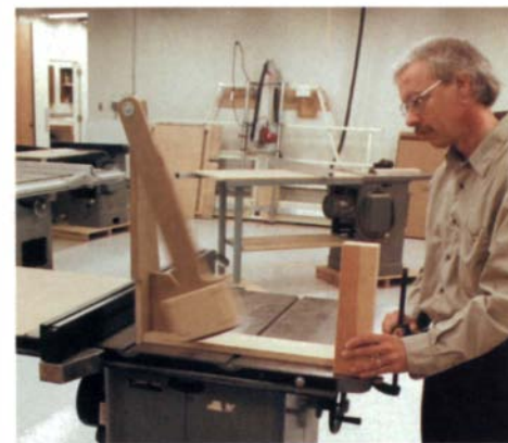
Getting whacked. Swinging a 2-ft.-long, 3-lb. pendulum at the outfeed end of each fence approximates what happens in a shop when a fence gets knocked by heavy sheet goods. After whacking the fences, they were checked for parallelism. All but one fared well.
