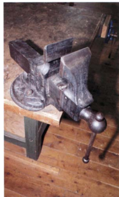
Smooth operator. This antique Prentise vise (right) has smooth faces that won't mar wood.
