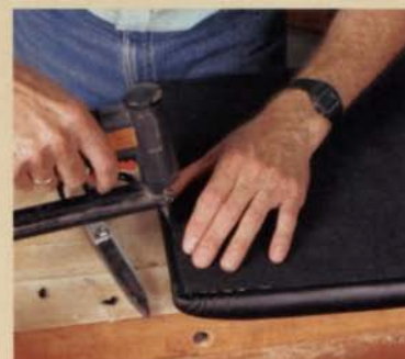
Black fabric finishes the bottom of the seat. Fabric for the underside of the seat is folded and tucked under itself before being tacked into place. Afterward, the author found the holes for T-nut fasteners and snipped cutouts in the fabric as clearance for the machine screws that hold the seat to the chair frame.
