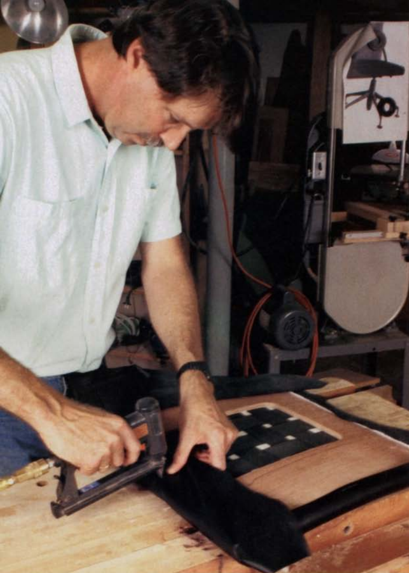
Start in the middle. The author stretches and staples the finish cover (in this case, leather) along the middle of each edge.
