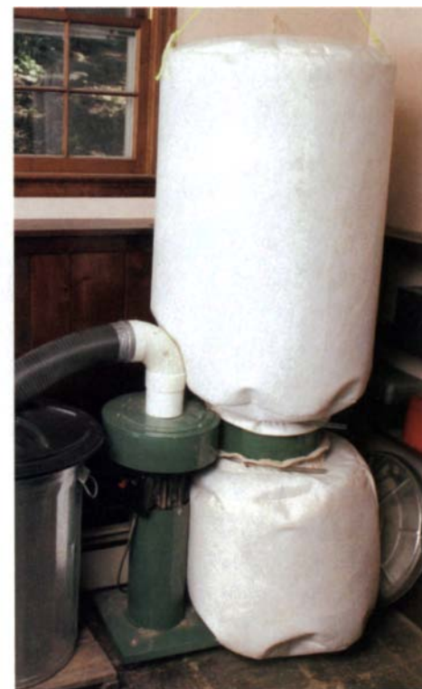
Big bags improve airflow. High-efficiency dust bags from Oneida Air Systems will keep you and your collector breathing easier.
