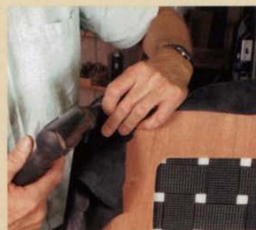
Next pull and tack each corner. Depending on the thickness of the cover material, you may need to fold in a visible pleat at the corners.
