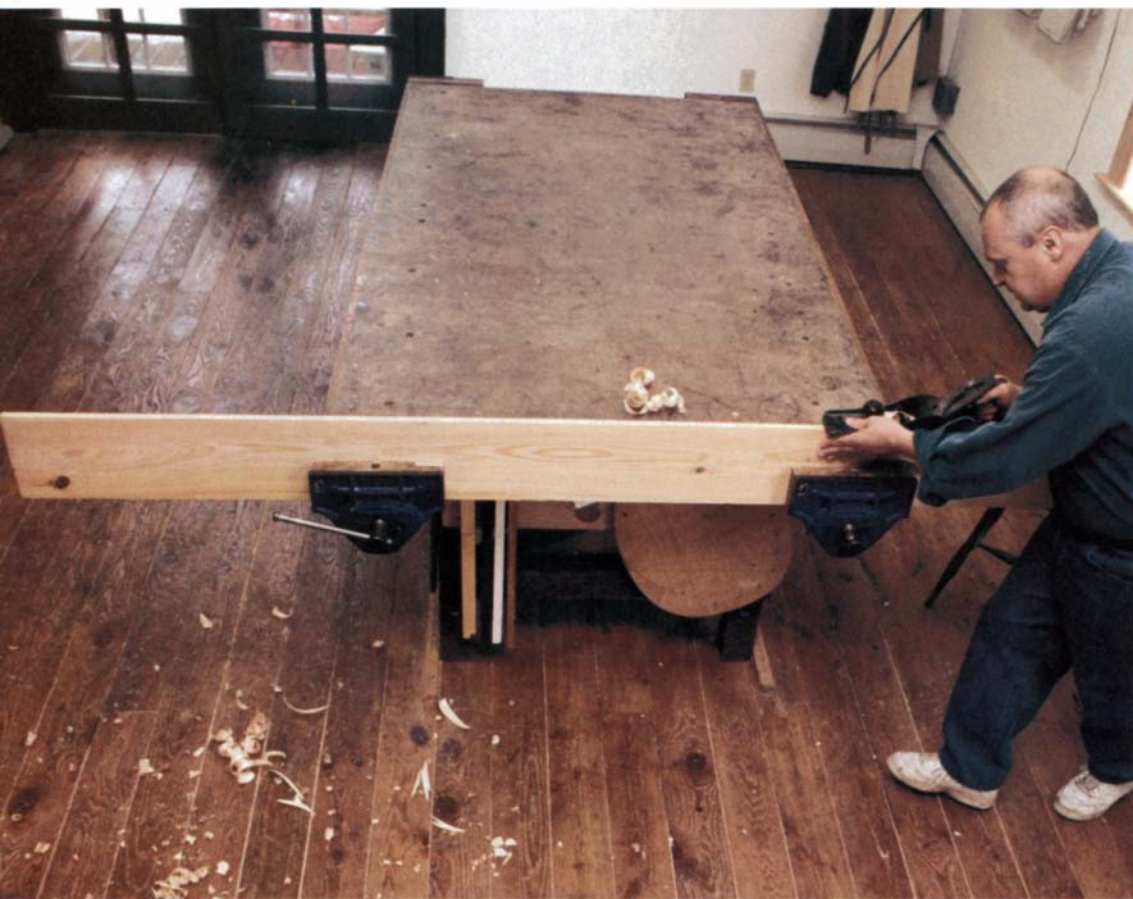
Smooth operator. This antique Prentise vise (right) has smooth faces that won't mar wood.
