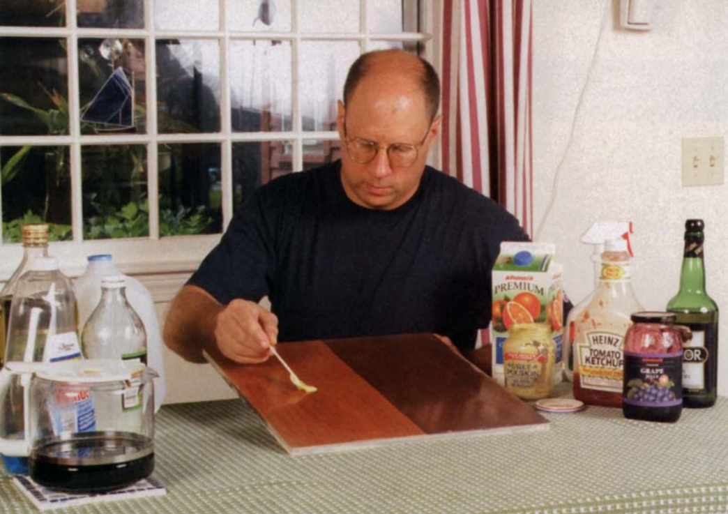
Food-stain test. Finishes were subjected to a variety of common foods and cleaners. Most finishes held up very well. Cleaning products, however, were hardest on the finishes.
