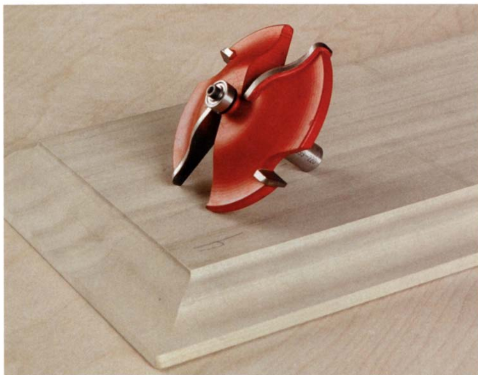
Clean-cutting bits. Freud's 2+2 panel-raising bits, which have four cutting wings instead of the usual two, leave a tearout-free edge where the ramp meets the field.
