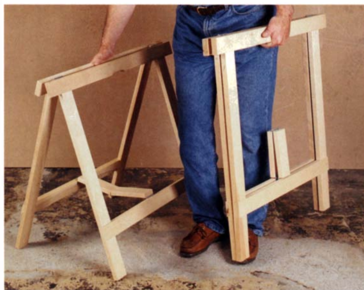
Sturdy folding sawhorses. Quick-Fold sawhorses flatten to 2¼ in. when stowed.
