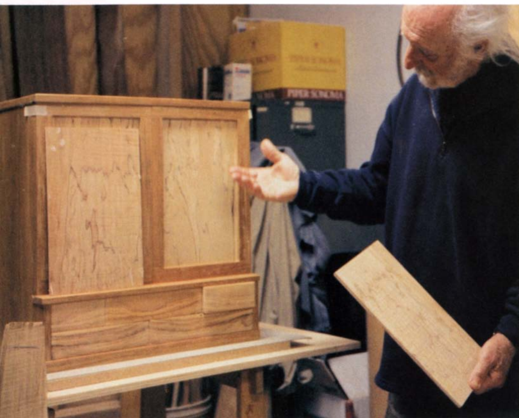
Panel discussion. Krenov liked the pattern of spalting in another pair of panels he cut for the doors, but as he demonstrates in the photo above, the color was too pink for the cabinet. The finished cabinet (right), with its harmony of colors and patterns, proves again that when it comes to reading grain, Krenov wrote the book.
