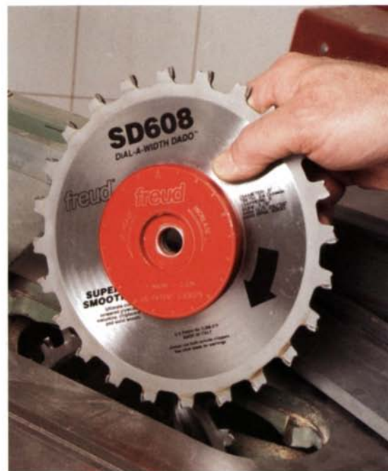
Dial Freud for a dado. Freud's Dial-a-Width dado does away with the nuisance of shims.
