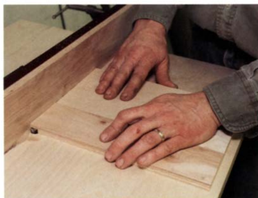
Gang several pieces together. Cutting two or three pieces at once improves stability against the fence and reduces tearout.
