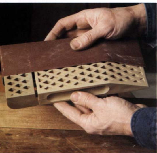
Hand-sanding block. The SandDevil uses 3-in. by 21-in. abrasive sanding belts.
