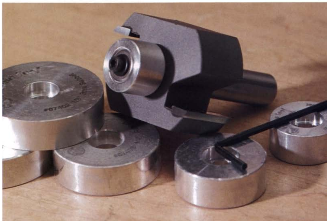
Heavy-duty rabbeting bit. Amana's Superabbet router bit uses rub collars of different sizes that fit over the bit's bearing.
