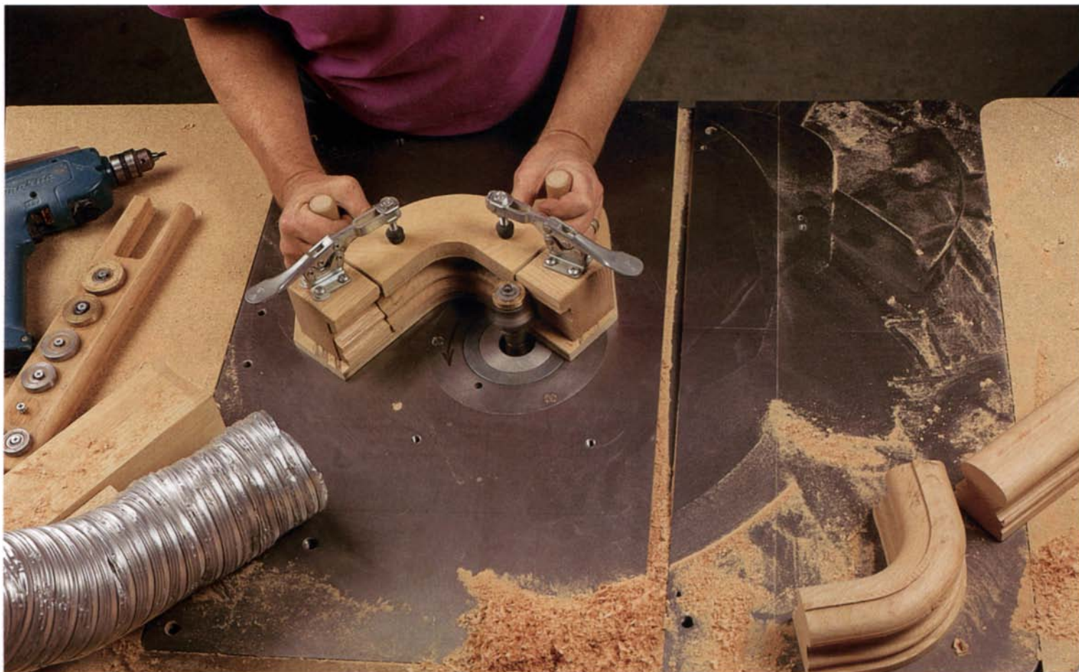
Pattern cutting is a shaper's strong suit —To pattern-shape small parts, the author uses jigs with handles and clamps. Pattern cutting is one of four jobs where the author says a shaper outperforms a router and router table.
