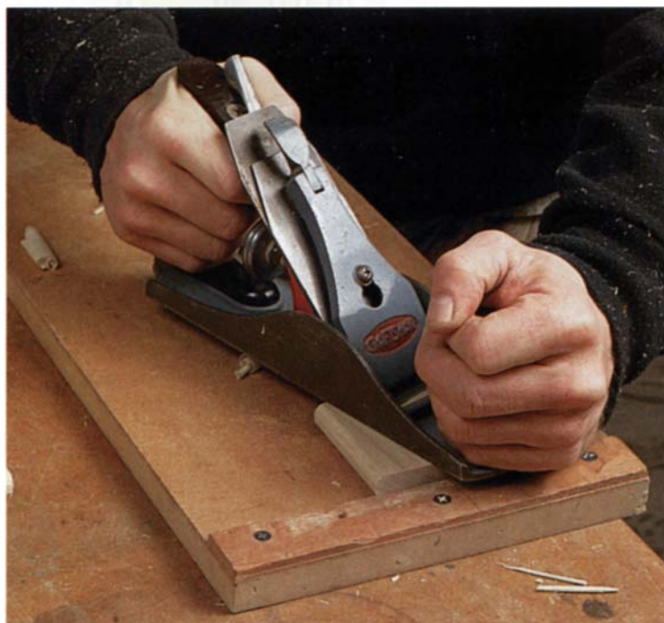
A couple of passes with a handplane take the tenon stock down to size. The author mills the tenon stock a hair thick, so he can get a precise fit for each joint with a plane.
