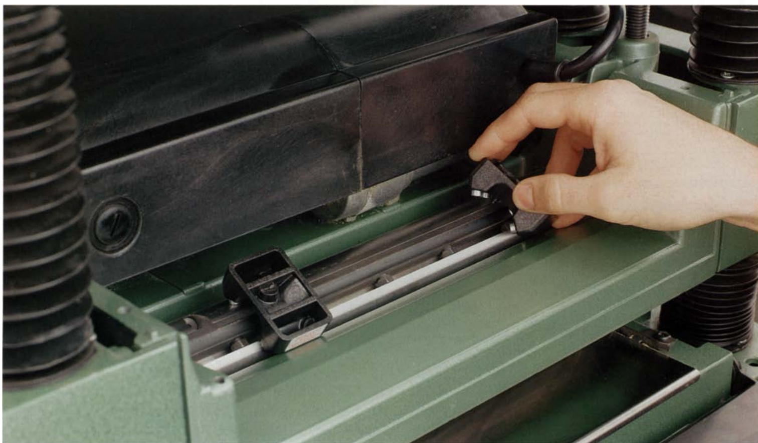
Quick, accurate knife changes on portable planers. Planer Pals, a pair of polycarbonate castings with embedded magnets, take the hassle out of setting knives on many portable planers. It takes no more than five minutes to use Planer Pals.
