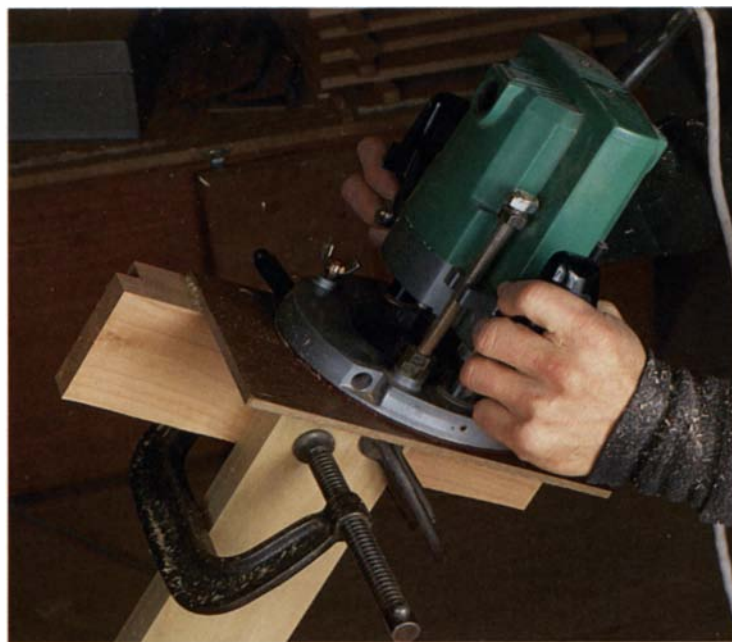
Simple router mortising fixture works for leg and rail. A slotted piece of hardboard screwed to a hardwood block provides all the guidance you'll need for routing accurate mortises. A spacer inserted between fence and rail correctly positions the template for the rail mortises.
