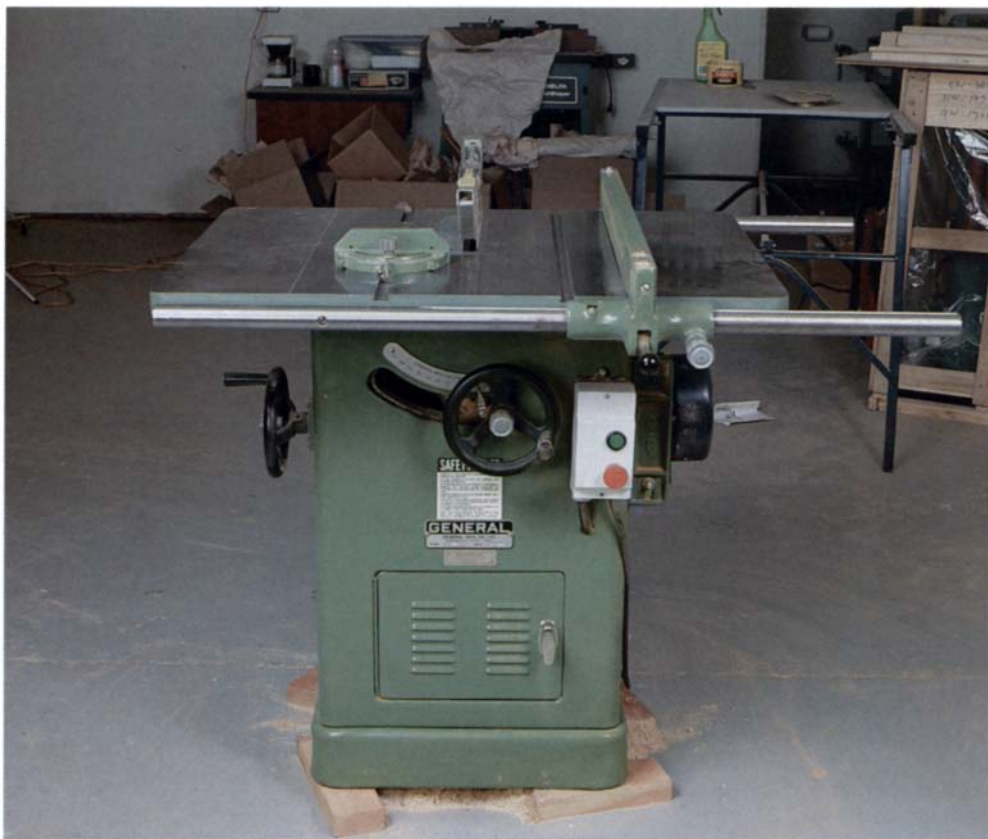
Top-quality saws cost between $1,500 and $2,000. These saws, what the author describes as Class A machines, have solid cast-iron tables and extension wings and a full-length fence. These heavy-duty, smooth-running machines form the backbone of many small professional and serious amateur woodworking shops.
