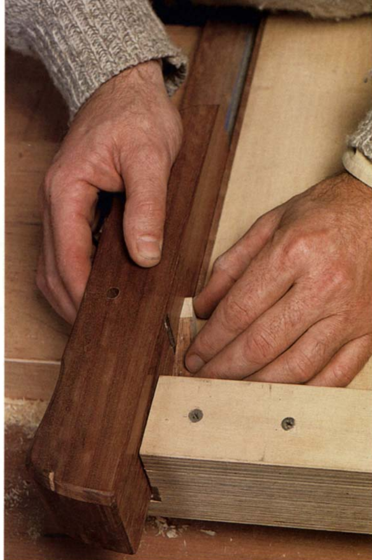
Fine adjustment for fit. A plane and a shooting board helped the author trim pieces, so they conformed exactly to the elliptical plan he worked from.
