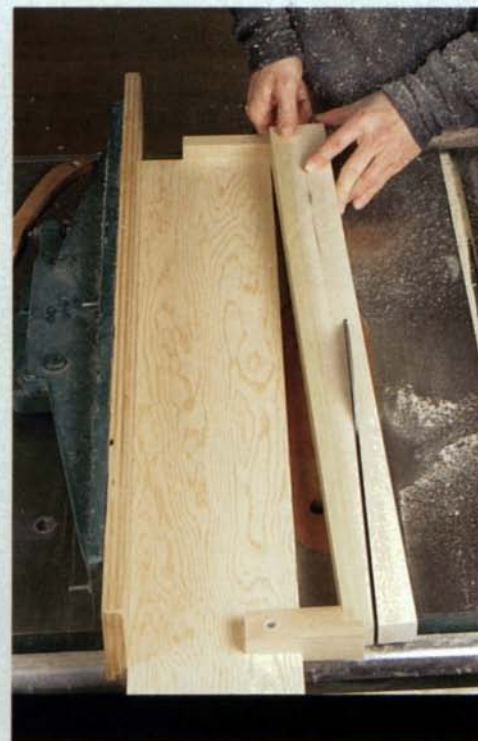
After the first taper cut, turn the leg so the cut faces up. This keeps a jointed face on the saw table and a square end against each stop for the second cut.
