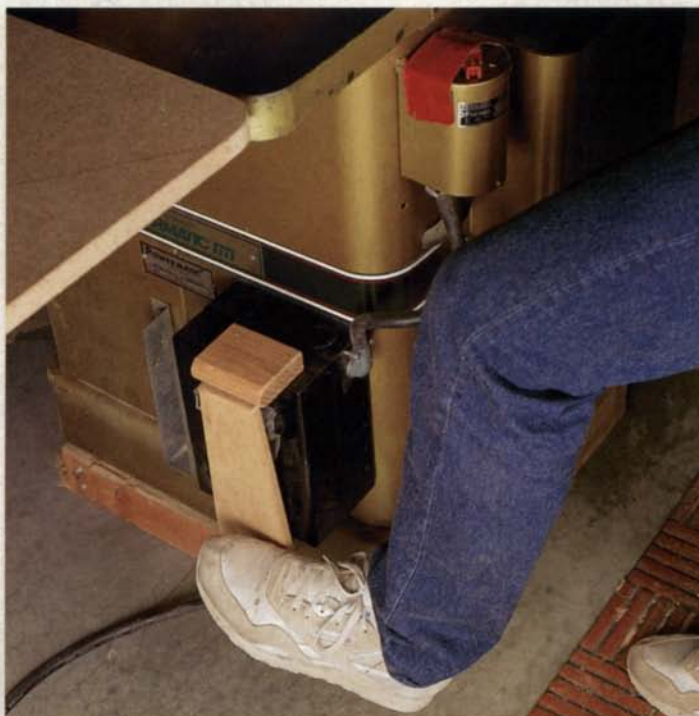
A kill switch offers security, so the author built this foot-controlled off switch. He also keeps the spindle-reversing switch taped, so he doesn't change the cutter rotation inadvertently.
