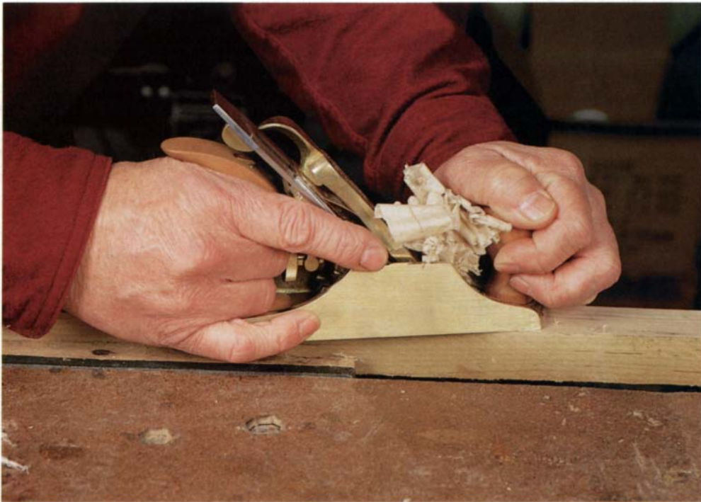
Bronze bench plane by Lie-Nielsen is better than Stanley original. Lie-Nielsen's first bench plane, a No. 2 Bedrock, is heavier and more precisely milled than its Stanley forebear. And the plane offers better seating between the frog and the plane body.
