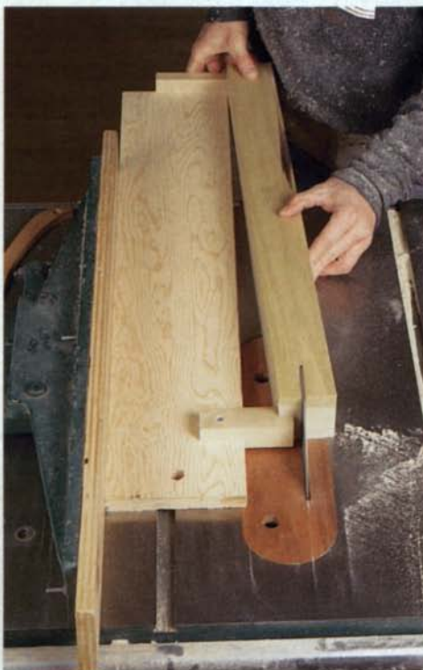
Dedicated taper jig ensures safe, consistent results. With stops both front and back, this jig captures the leg snugly, keeping it from vibrating or moving as it's cut.
