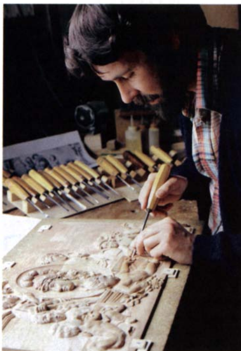
Cast panels start with a wooden pattern. A Daïdé craftsman, one of 20 specialists who worked on the desk, carves a panel used to fabricate a finished part.
