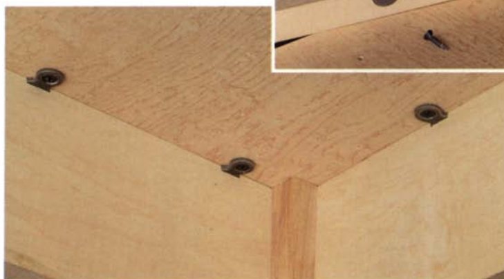
Figure-eight clips can be installed after the base is complete. With these clips, you drill only one shallow, flat-bottomed hole in the rail. Screw the other half of the "8" into the underside of the tabletop.
