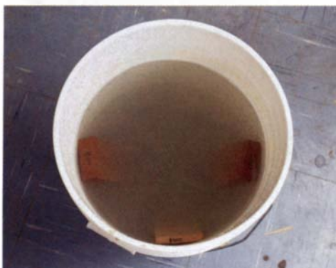
Salvaged 5-gal. bucket makes a good storage bin for waterstones because it contains plenty of water to keep the stones clean. Place a section of perforated rubber mat at the bottom of the bucket to cushion the stones and to keep them from sitting in a slurry of mud.
