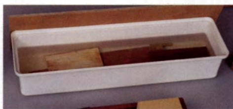
Keeping slip stones in a separate smaller bin keeps them safe. Otherwise, the big stones in a bucket would stand a good chance of breaking the slip stones.
