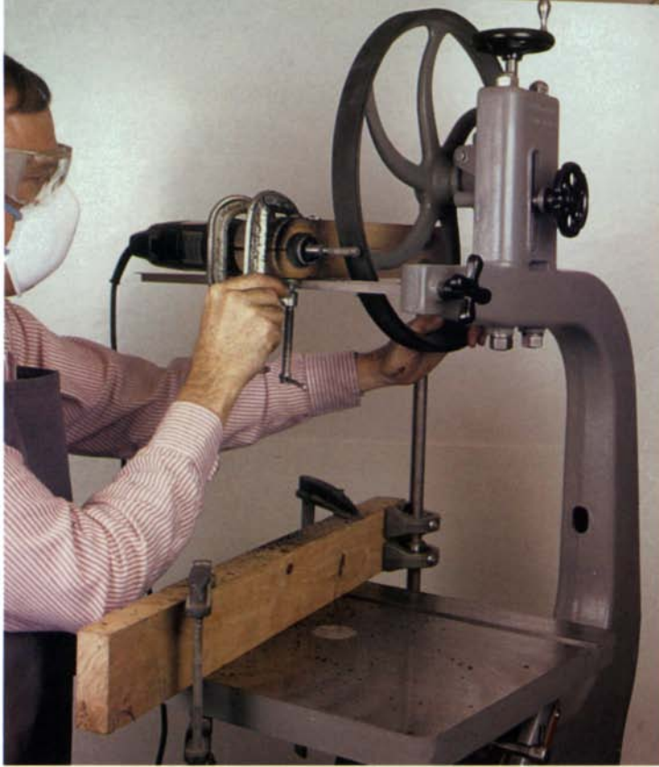
Vaughan's jig for trimming and crowning the tire holds an electric die grinder fitted with a flush-trimming router bit clamped in a pivoting bracket. He clamps the jig to the bandsaw with the
