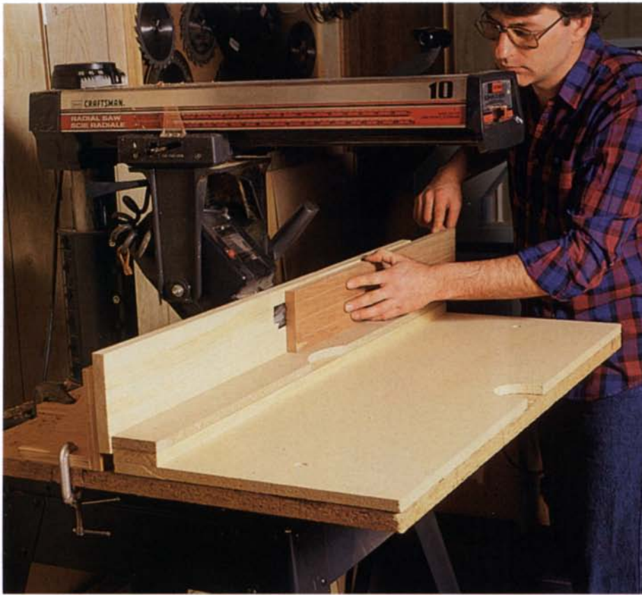
An auxiliary table and fence make shaping on the radial-arm saw a safe process. Because the motor can be tilted to almost any position, an infinite variety of shapes can be cut using just a molding head and a basic set of knives.
