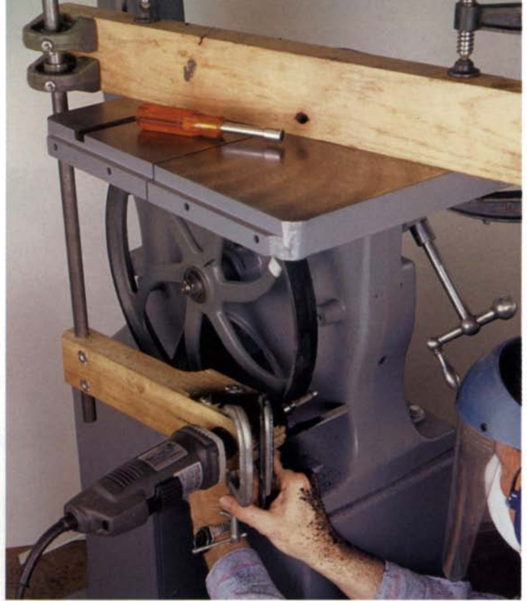
pivot shaft extending up for working on the top wheel (left) or down for the bottom wheel (right). Each tire is trimmed twice at a slight angle from each outer edge to form a V-shaped crown.
