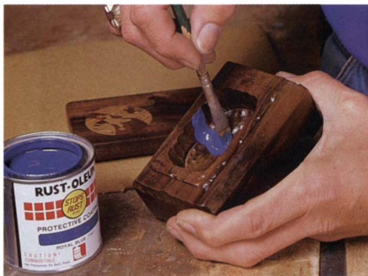
Seal the routed-out interior of a box with a coat of lacquer, and then apply an enamel paint to act as an adhesive for the flock. Using the same color paint as flock produces a rich, uniform appearance, even on irregular surfaces.
