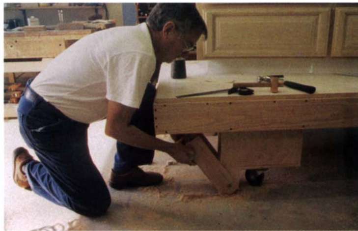
Shopmade cam brakes hold the table immobile. A little wax on the fulcrum screw keeps the cam working smoothly.
