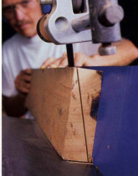
The author resaws a 2x8 with his bandsaw table tilted 15° to rough out the wedge-shaped segments that form the column. To ensure a good grain match, all 24 segments are cut from two long boards milled from a single tree.
