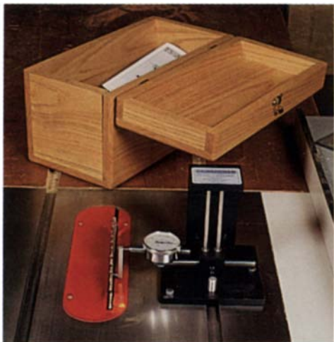
TS-Aligner consists of a dial indicator mounted on an arm that travels vertically on linear bearings. The cam-follower bearings that fit in the miter-gauge slot allow horizontal movement.
