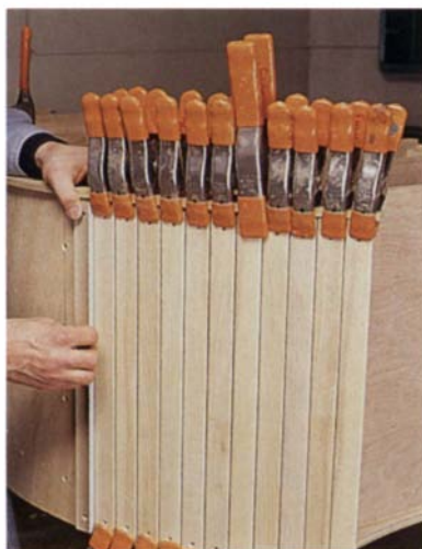
Solid-wood edgebanding that's laminated together from thin strips covers the edges of the bent-plywood carcass. The carcass itself acts as the bending form, and spring clamps hold the glued laminae in place.
