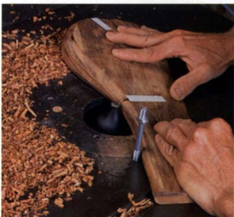
After bandsawing the outer edge to the pedestal's profile, the author rounds over each segment's edge on a router table. He uses two different bits: a ⅜-in. radius bit for the narrow upper portion and a ¾-in. radius bit for the wide lower portion (above). Masking tape designates where to stop each cut.
