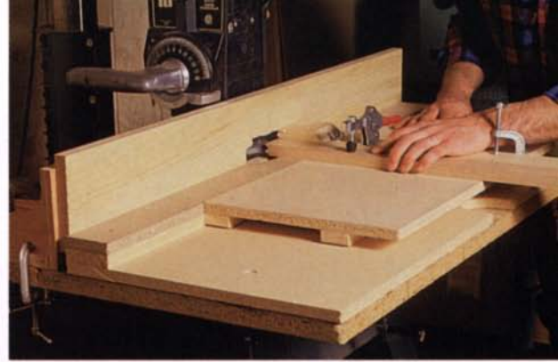
A sliding carriage, with an adjustable fence and a toggle clamp to secure the stock, makes shaping ends for cope-and-stick frames simple and safe.
