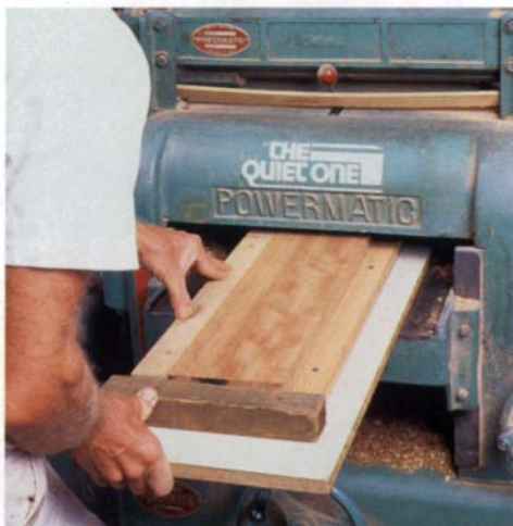
To clean up the bandsaw marks and to provide a good surface for gluing, Carr runs the segments through the planer on a carrier. The carrier holds the beveled segment's surface parallel with the planer table.
