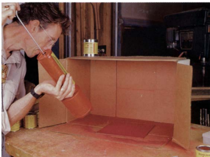
The best way to flock larger surfaces is with a pump-action flocking gun. The author shoots an even coat onto a painted drawer bottom. A cardboard box traps the overblown flock, allowing it to be scooped up and reused.
