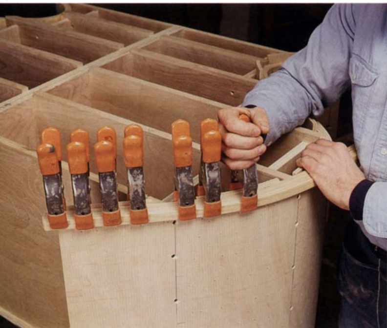
Solid-wood edgebanding that's laminated together from thin strips covers the edges of the bent-plywood carcass. The carcass itself acts as the bending form, and spring clamps hold the glued laminae in place.
