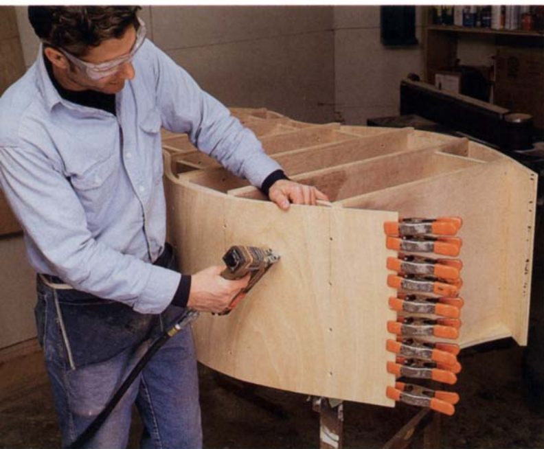
The author glues and nails a second layer of thin bending plywood over the first, which was screwed to the end of each divider as the ply was bent into place. Byers uses spring clamps temporarily to keep the ply in place while a pneumatic nail gun drives dozens of brads to secure the layer.
