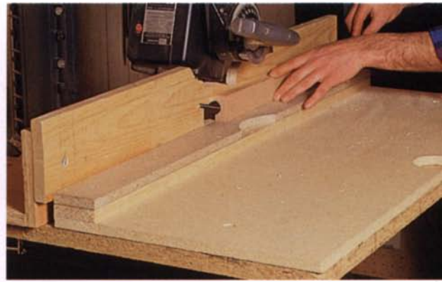
An auxiliary table and fence make shaping on the radial-arm saw a safe process. Because the motor can be tilted to almost any position, an infinite variety of shapes can be cut using just a molding head and a basic set of knives.
