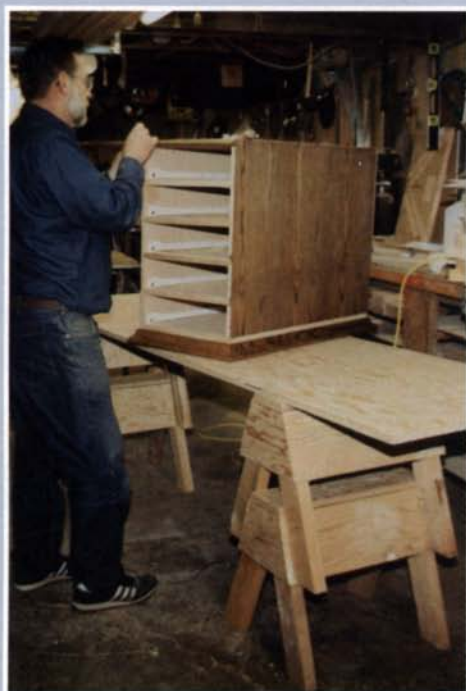
A combination mini-sawhorse and toolbox, these saw ponies are extremely versatile. Their rugged construction and low stature make them very stable.
