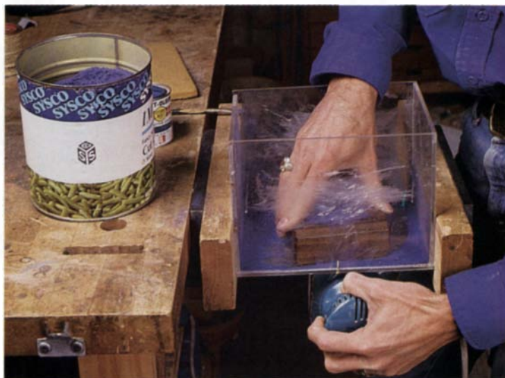
After sprinkling the box with flock, hold it against the bottom of a thin-walled box vibrated by an orbital sander. The vibration causes the flock fibers to stand on end, producing an evenly coated, plush surface. Pour out the loose flock, and set the box aside to dry.
