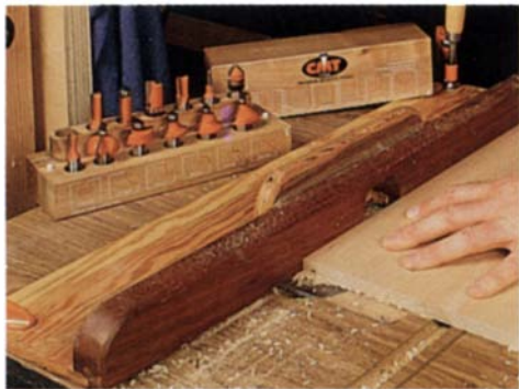
Even in rock maple, CMT bits met little resistance. Proprietary micrograin carbide provides a fine cutting edge, and baked-on Teflon all but eliminates drag. The bits are available individually or in sets.
