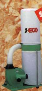
UFO-101 2HP/1Phase 1182CFM two 4" collection inlets
