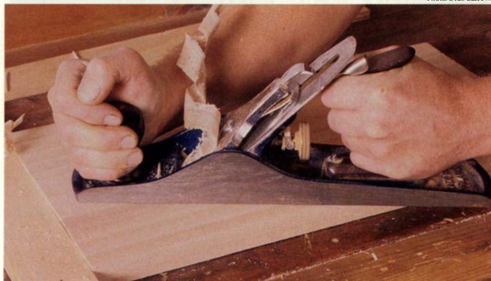
Paulownia can be easily worked with sharp tools, and can be planed to a satiny surface that needs little or no sanding before finish is applied.
