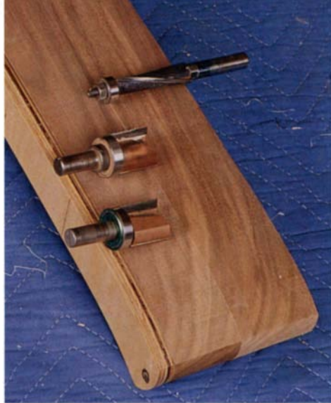
Routing thick frame members, such as the crest rail shown here, requires multiple passes with standard straight bits and pilot bearings, both above and below the cutter.
