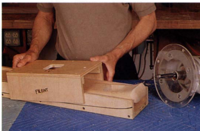
Through mortising frame parts is done by routing from two sides using a box jig with a template cutout for the first cut and a removable platform to support the router for the finish cut.
