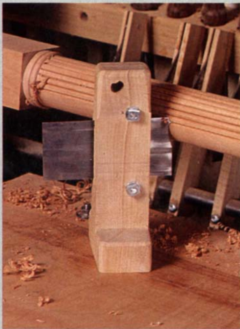
Campbell cuts reeds with a scratch stock made from a scraper blade that's bolted in a saw kerf in a T-shaped tool post. The tool post slides on a plywood platform attached to the lathe bed.
