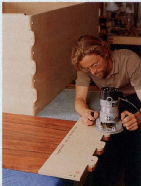
To rout the carcass's strong finger-joint corners, Dale uses a large finger template made from \frac{1}{2} -in. plywood. He saws out the waste first, routs using the template and a flush-trimming bit and squares up the corners with a sabersaw and chisel.
