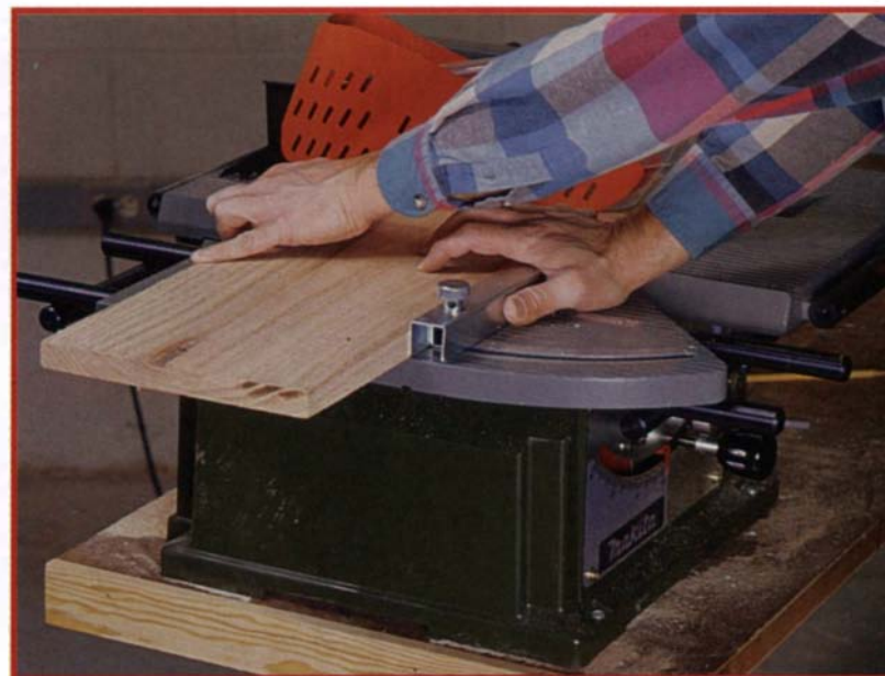
The Shopsmith's miter gauge (left), with its hand-triggered hold-down clamp, secures the stock during a cut. After pulling the blade through the cut, a spring returns the carriage.
