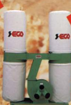
UFO-102B 3HP/1Phase 1883CFM, 4 bags 10.48 CU. FT. of volume Three 4" inlets
