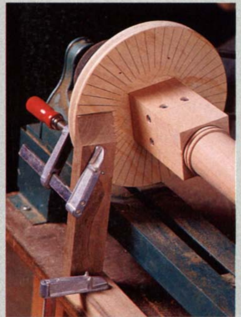
For lathes without indexing rings, a shop-made indexing plate can be attached to the headstock end of a spindle, independent from the lathe itself. A rigid pointer arm is needed to use the indexer.
