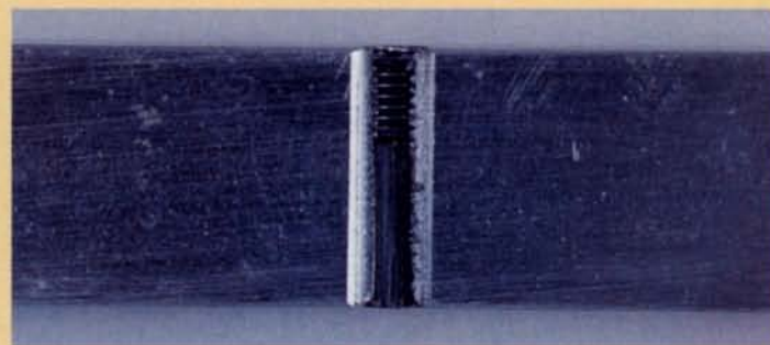
A Cool Block and a setscrew inserted into a threaded hole machined in the miter-gauge bar, as shown in this cutaway view, can eliminate play between the bar and the tablesaw slot, thus improving the performance of any miter gauge.
