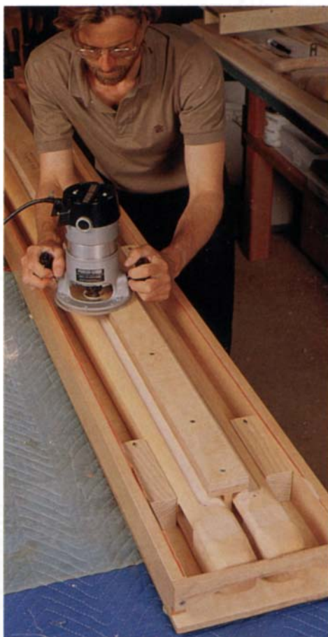
The box jig, used for shaping the edges of the armoire's frame members, is also used for routing dadoes in the front posts for attaching the solid-wood carcase.
