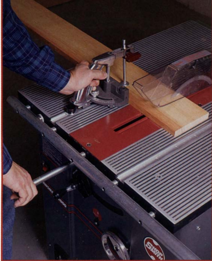
The Shopsmith's miter gauge (left), with its hand-triggered hold-down clamp, secures the stock during a cut. After pulling the blade through the cut, a spring returns the carriage.
