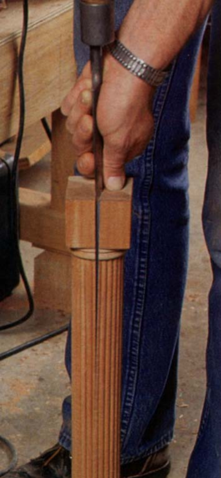
Campbell's quartering method resembles firewood splitting. The glue line is cleaved easily due to the layer of newspaper between.
