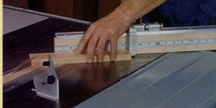
A miter gauge is essential to safely crosscut and miter on the tablesaw. Here the author uses a FasTTrack miter gauge, with adjustable fence and micro-adjustable flip stop.
