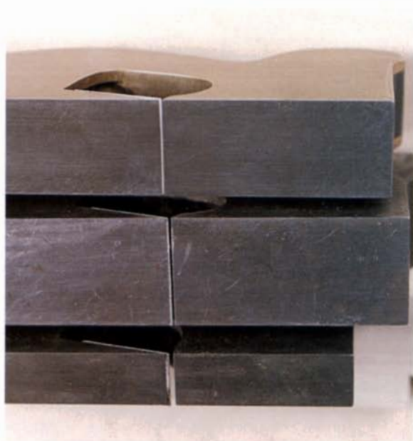
A fine mouth opening is a sign of quality. The Norris (top) has a minute cutting aperture of .010 in.; the Mathieson (middle), an acceptable .025 in.; and the Record #042 (bottom), a marginal .051 in.
