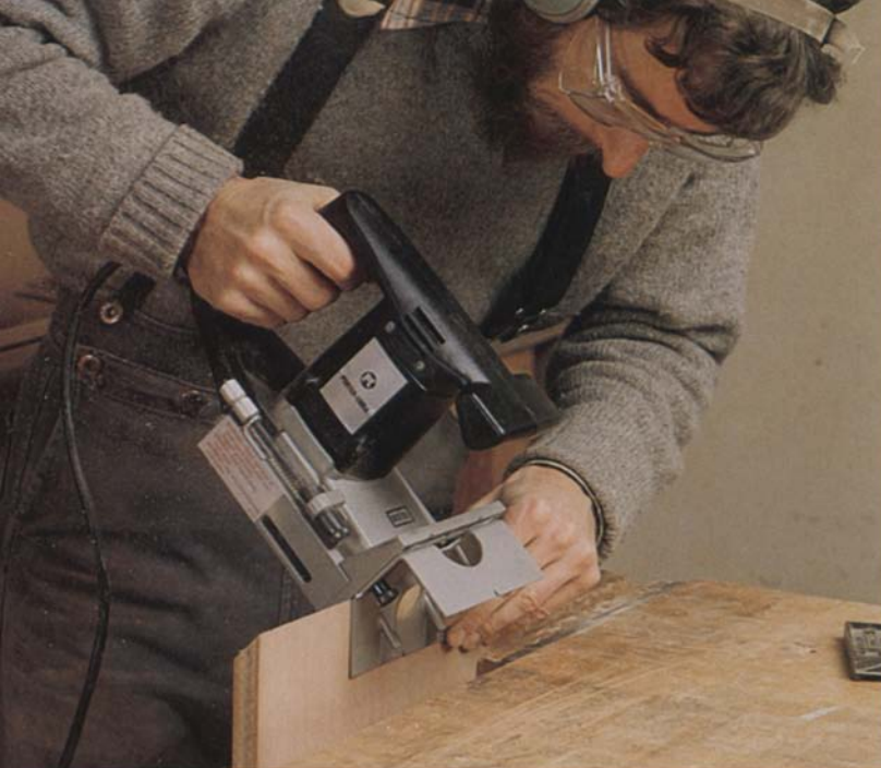
The adjustable fence on the Porter-Cable Model 555 flips over and positions the machine for cutting slots on a mitered panel's edge. Its 'D' handle design distinguishes it from other plate joiners, which must be grasped by the motor housing for plunge-cutting slots.
