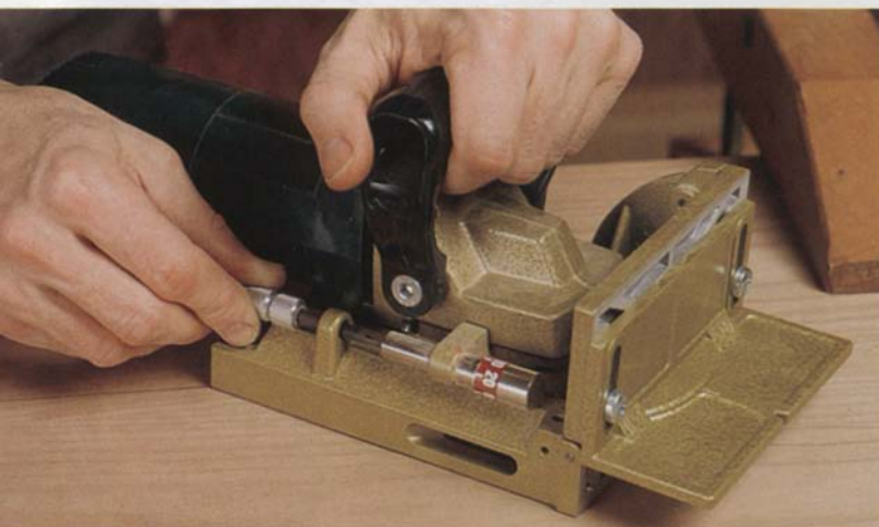
The stepped depth-stop on the Lamello Standard quickly sets to three positions that adjust the machine's depth of cut to make slots for different-size plate-joinery biscuits. Similar depth stops are found on most other models.
