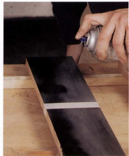
Deft spray lacquer makes a good finish. Just make gentle overlapping passes with the spray, as shown, then sand lightly between coats.
