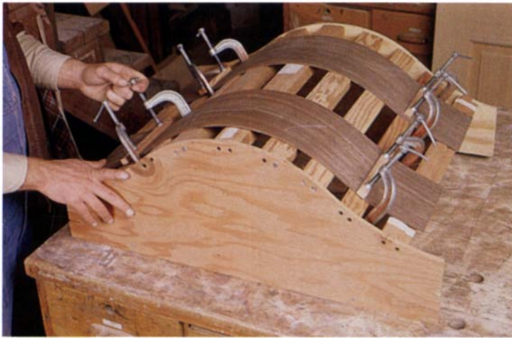
A bending form, screwed together from scraps of 1/2-in. plywood, lends shape to the two 1/8-in.-thick walnut pieces that will form the cabinet's arched top. The radii of the jig are slightly tighter than the final shape of the top, to allow for springback when the steam-bent pieces cool.
