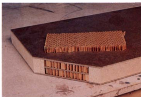
Surrounding a corrugated-paper honeycomb material with a particleboard frame and sandwiching it between layers of MDF, smooth hardboard or particleboard creates a strong, rigid and lightweight panel.
