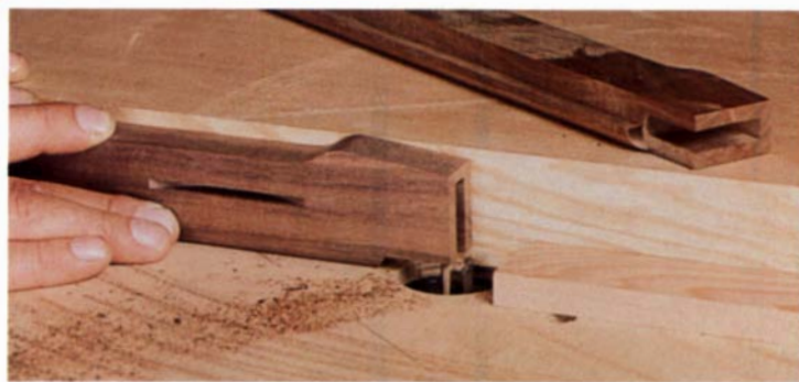
A \frac{1}{2} -in. straight bit in the router table cuts the cope in the ends of the stiles and removes the sticking where the rail and stile will mate. Here the stop block is set for cutting one end of each stile; the other ends are cut with the block left of the bit.
