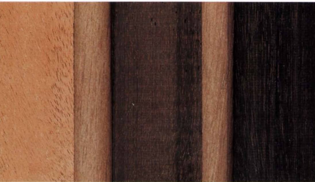
A strip of mahogany, above, illustrates how each coat of stain darkens the wood. The left side is plain; the center has one coat of the steel wool/vinegar mixture; and the right, three coats. Each coat is sanded with fine paper before the next coat is applied. Applying a coat of aniline dye on top of the stain darkens the wood even further (see p. 50 for more on aniline dyes).
