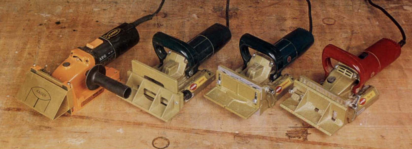
Plate joiners are plunge-cutting circular saws that create slots for football-shape biscuits, glued into the slots like splines. The machines above, from left to right, are the Kaiser Mini 3-D and the Lamello Junior, Standard and Top 10.
