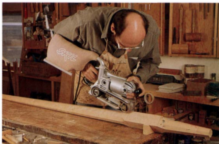
With the shaped post supported by a simple V-block, Becksvoort beltsands the machining marks from the tapered bevels of the octagon. A smooth, continuous motion and a light touch with the nose of the belt sander are requirements for sanding the curving transition from bevel to square.
