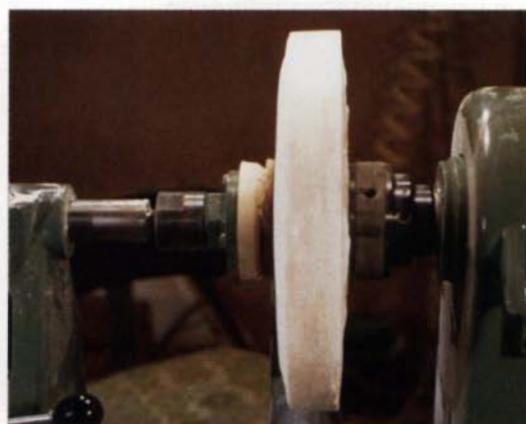
Above: To center and clamp the preturned wood base to the piece, the author uses a stub with the proper Morse taper for the tailstock on one end and threads for a faceplate on the other. The base is then
