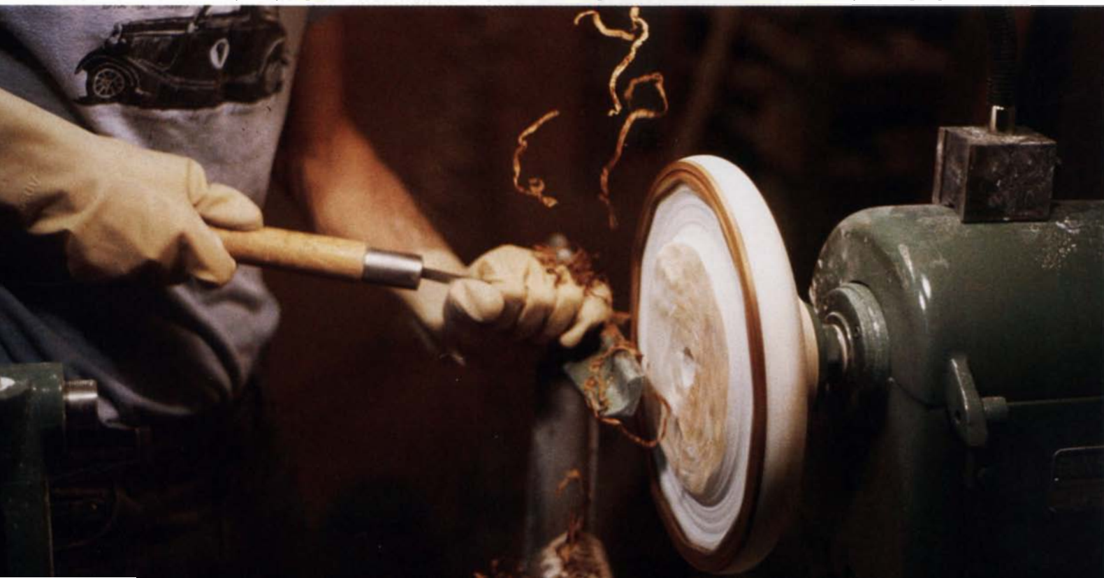
Above: To center and clamp the preturned wood base to the piece, the author uses a stub with the proper Morse taper for the tailstock on one end and threads for a faceplate on the other. The base is then
