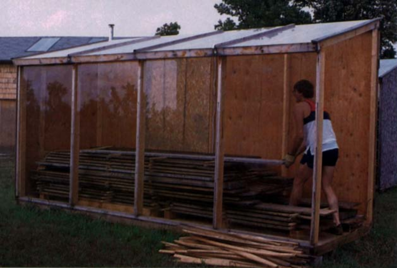
The simplicity of the solar-kiln construction is evident in the above photo. The plywood panel from one end is removed to allow access for unloading a dry batch of lumber.
