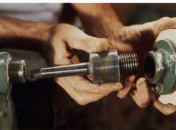
Above: To center and clamp the preturned wood base to the piece, the author uses a stub with the proper Morse taper for the tailstock on one end and threads for a faceplate on the other. The base is then
