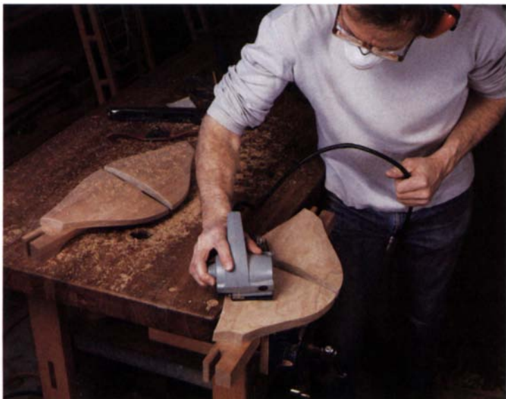
Once the backrest plaques are joined to the back rail and clamped to the bench, they are roughed to shape with a small motorized block plane. The author then uses spokeshaves and scrapers to refine and smooth the forms.
