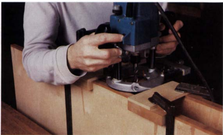
With a 1/2-in. spiral-fluted straight bit in a plunge router, the author cuts through mortises in the chair's armrests and legs. The chair parts are clamped inside a plywood jig, which guides the router base as it cuts the mortises. Two adjustable stops clamped to the top of the jig's sides act as stops to determine mortise length.
