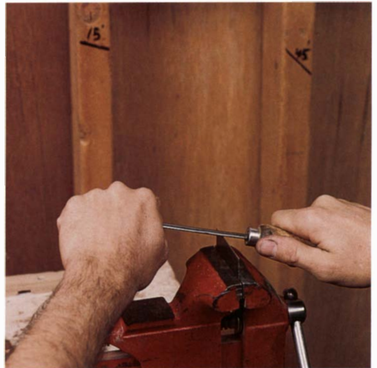
The final step in tuning the scraper is to form the cutting hook on the edge of the blade. The author is shown here burnishing the scraper's edge using a 15° line marked on the wall as a guide. Earlier, in preparation for forming the hook, the blade is flattened and its edge is made straight and filed to form a 45° bevel.
