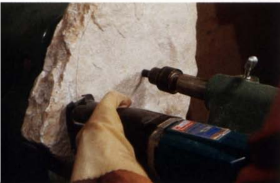
The blank can be rough-cut round with a reciprocating saw.
