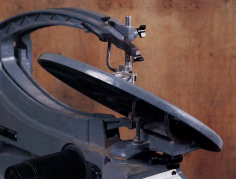
The tables on most scroll saws tilt, allowing beveled cuts to be made. Here, the table on the Delta is tilted to 45°, revealing the two trunnions that support the table, as well as the stop bolt that accurately references the table when it's returned to square.
