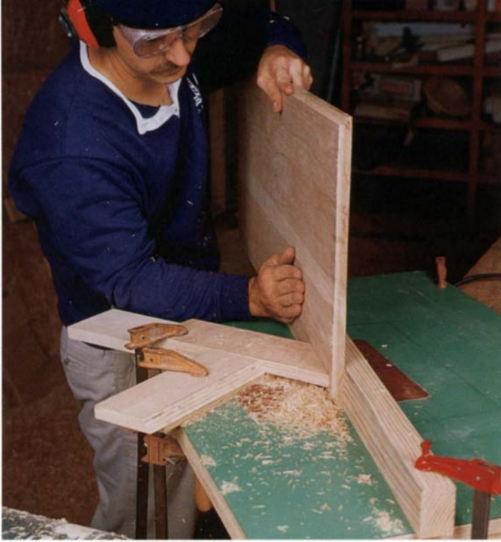
The author makes raised panels for the wardrobe doors on the router table. In the first step, shown above, he reduces the thickness of each panel's edge by running the panel vertically by a straight bit. A fingerboard clamped to a spacer provides the pressure needed to stabilize the panel as it's fed. This fingerboard also prevents the climb-cutting bit from self-feeding the panel.
