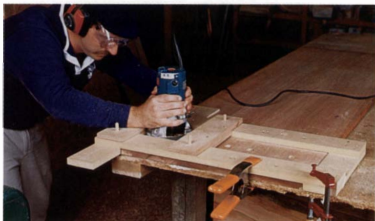
By changing the position of the two movable rails that guide the router, the author works his way across the bottom of the carcass side, chopping mortises for pin tenons that will join the sides to the bottom of his wardrobe cabinet.
