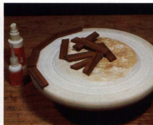
glued to the stone using the tailstock as a centering clamp. Wooden rim segments are applied with cyanoacrylate glue. Below: Turning procedures are much the same as for scraping cuts in wood.
