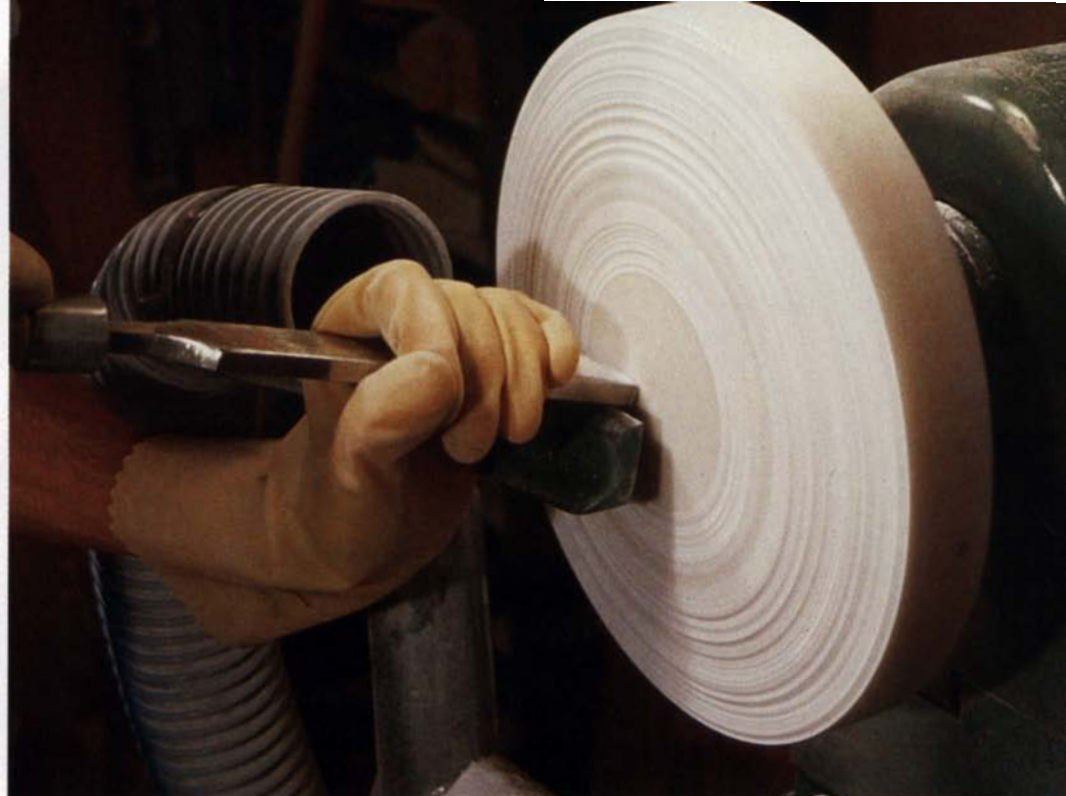
Initial scraping with carbide-tipped tools brings the stone to rough shape. Here, the bottom of the bowl is being trimmed flat with a high-speed steel scraper.
