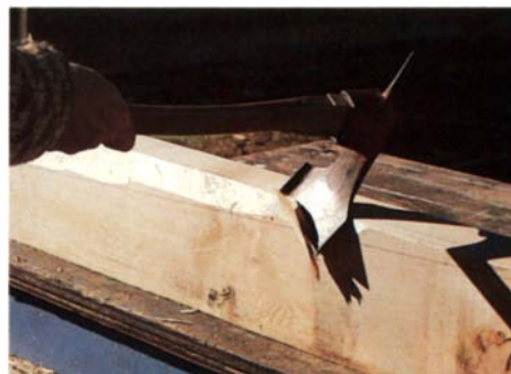
A razor-sharp adze precisely cuts to the line drawn along a Douglas fir beam. The spur shown is often used as a built-in nail set. A worker can quickly sink a nail below the surface, out of harm's way, then continue cutting.
