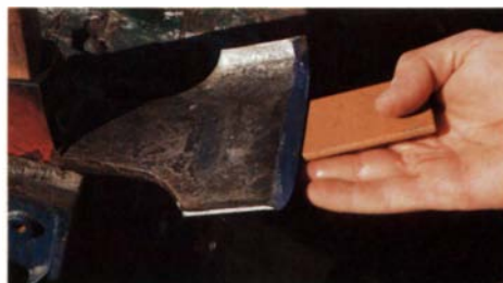
After establishing the 25° bevel and sharpening the edge with a flat mill file, Darr hones the back of the adze with a medium India whetstone, following with a flat, medium Arkansas stone.
