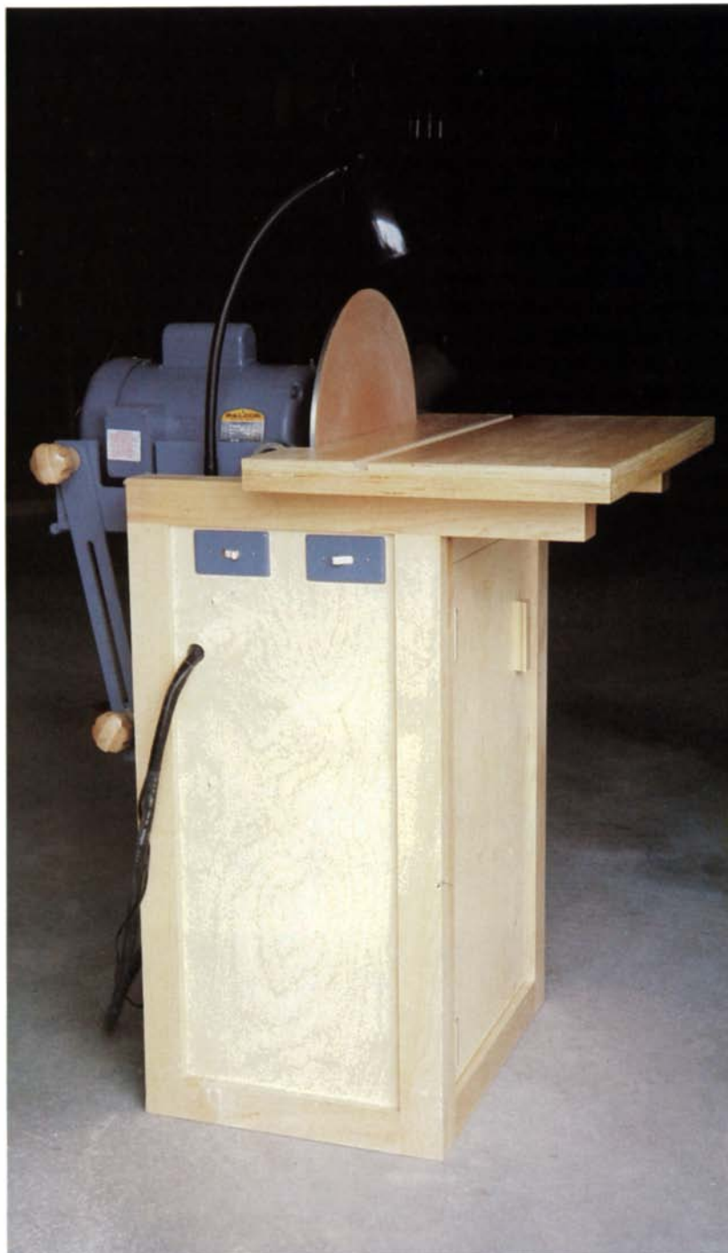
Dwayne Intveld's disc sander features a tilting disc, a reversible motor and straightforward construction.
