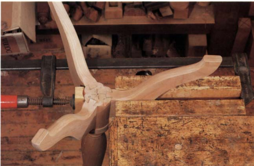
If necessary, you can secure one leg in a bench vise and use a clamp as shown to pull the shoulders tight on the tails.
