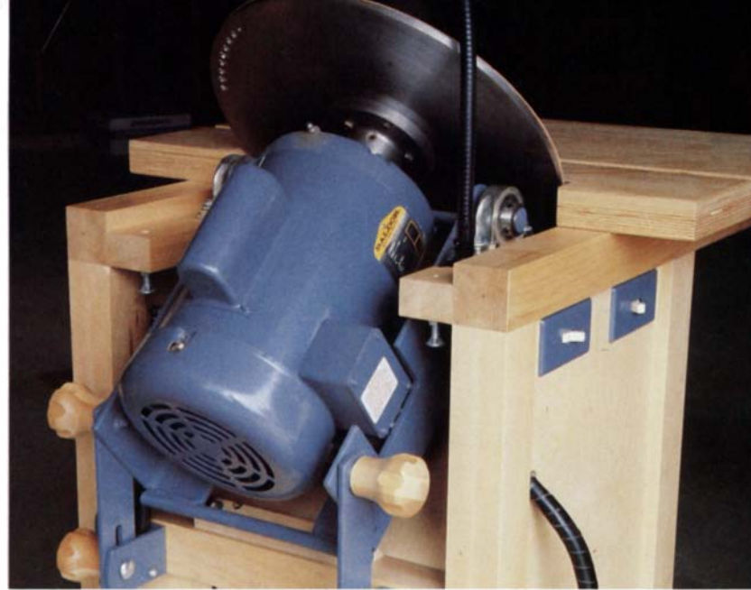
Built of commonly available iron stock, the motor carriage tilts to allow sanding at 45° and 90°, and any angle in between.
