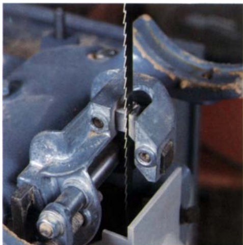
Delta's lower guides are designed with one side at a 45° angle, which allows them to be positioned close to the table for good support, while still allowing the table to tilt 45° to the right. In contrast, the Taiwanese saw's budget version uses the same guides top and bottom. To allow room for tilting, the guides must be positioned low, reducing support.
