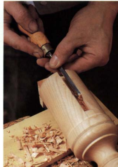
Use a backsaw to cut just inside the layout lines of the dovetail housing, left, then pare to the lines with a sharp chisel. The waste will come out in long strips. Once the leg goes in an inch or so, use the first part of the joint to guide the chisel to the full length of the housing, right.
