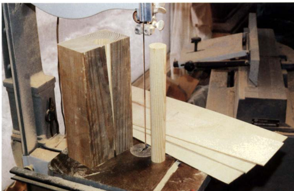
Bimetal blades may do for the bandsaw what carbide did for the tablesaw. This ¼-in. blade, at 25,000 psi tension, can both resaw without bowing and cut tight circles.
