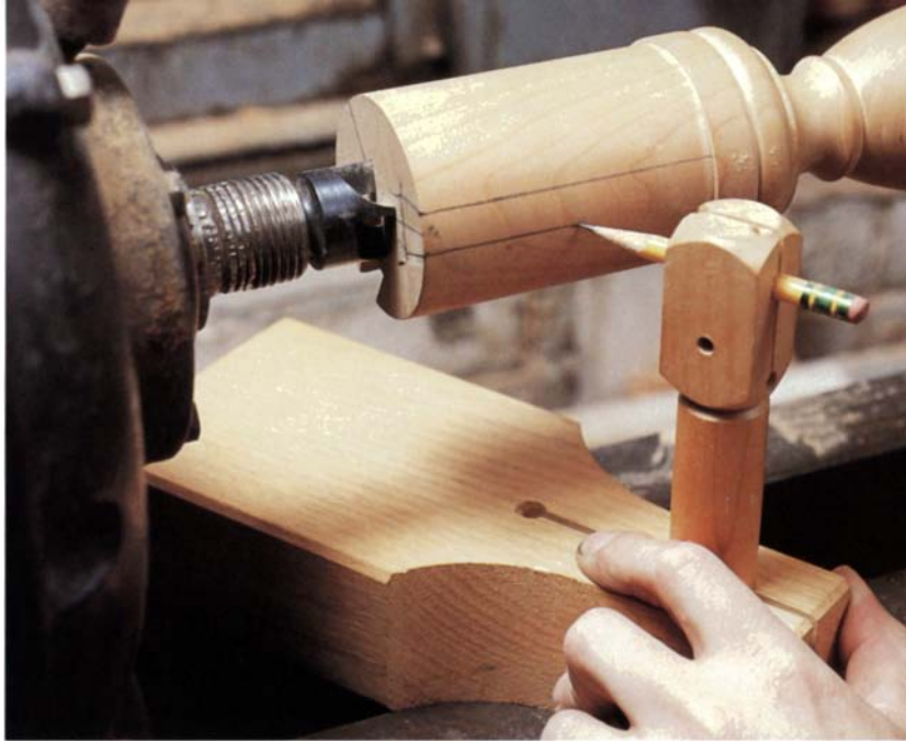
After remounting the column on the lathe, finish laying out the joint with a post scribe. The scribe slides on the lathe bed and draws housing lines parallel to the centerline of the column.
