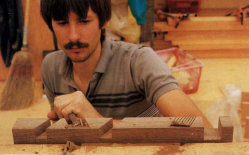
Cutting the tricky angled mortises for the legs (see figure 3) is a matter of sawing and chiseling before the table is glued up.
