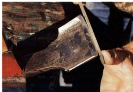
A mill file is used to joint the edge of the adze, and round the corners of the blade slightly so the center cuts into the wood first. The inside corners are sharpened with a round file, rotated slightly on each stroke to prevent grooving.
