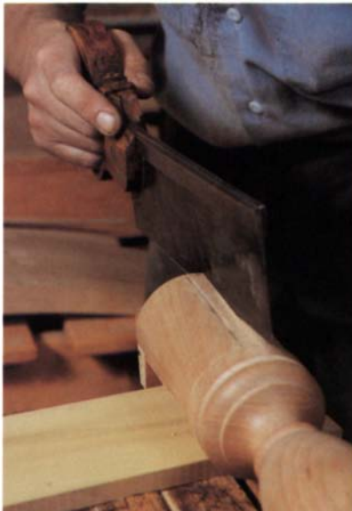
Use a backsaw to cut just inside the layout lines of the dovetail housing, left, then pare to the lines with a sharp chisel. The waste will come out in long strips. Once the leg goes in an inch or so, use the first part of the joint to guide the chisel to the full length of the housing, right.
