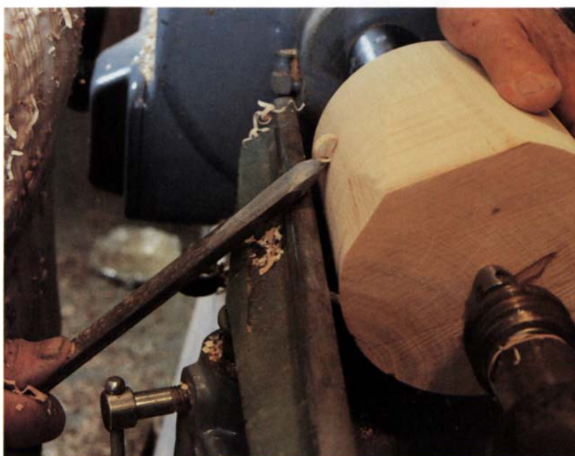
Practice cutting with the lathe off, rotating the wood by hand, until you understand how the tool rides on its bevel as it cuts.
