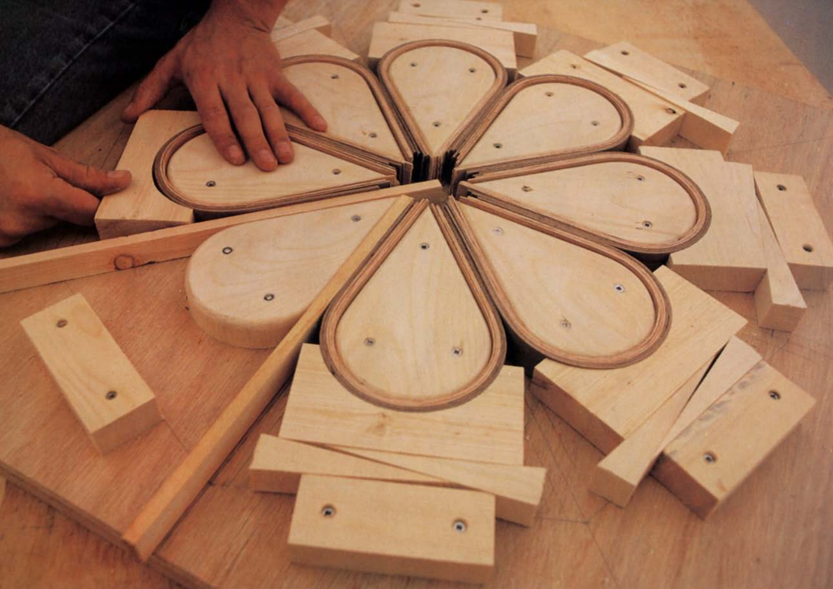
The key to a balanced wheel is an accurate form. Here the author bends steamed laminations into place for drying, after which they will be epoxied together into a rigid framework. The hub and rim are then added to complete the wheel.
