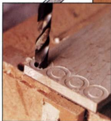
After the coves are laid out with a plug cutter, the pin holes are bored with a twist drill.
