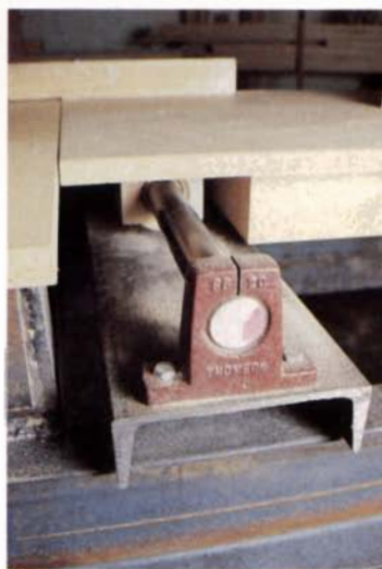
T.H. Ralph's sliding-table crosscut saw has 9-in. travel and will saw stock up to 2¼ in. thick. The Thomson linear-motion bearings, visible in the photo at near right, ride on a 1¼-in. precision-ground shaft mounted in a pair of steel supports. The sliding table's outboard end rolls on a wheel cannibalized from garage-door hardware. Its bearing surface (photo at far right) is a piece of heavy angle iron that can be raised or lowered to square the table to the blade in the horizontal plane.
