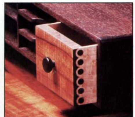
The handcut pin and cove joint shown on this small desk drawer is a captivatingly intricate alternative to dovetails.
