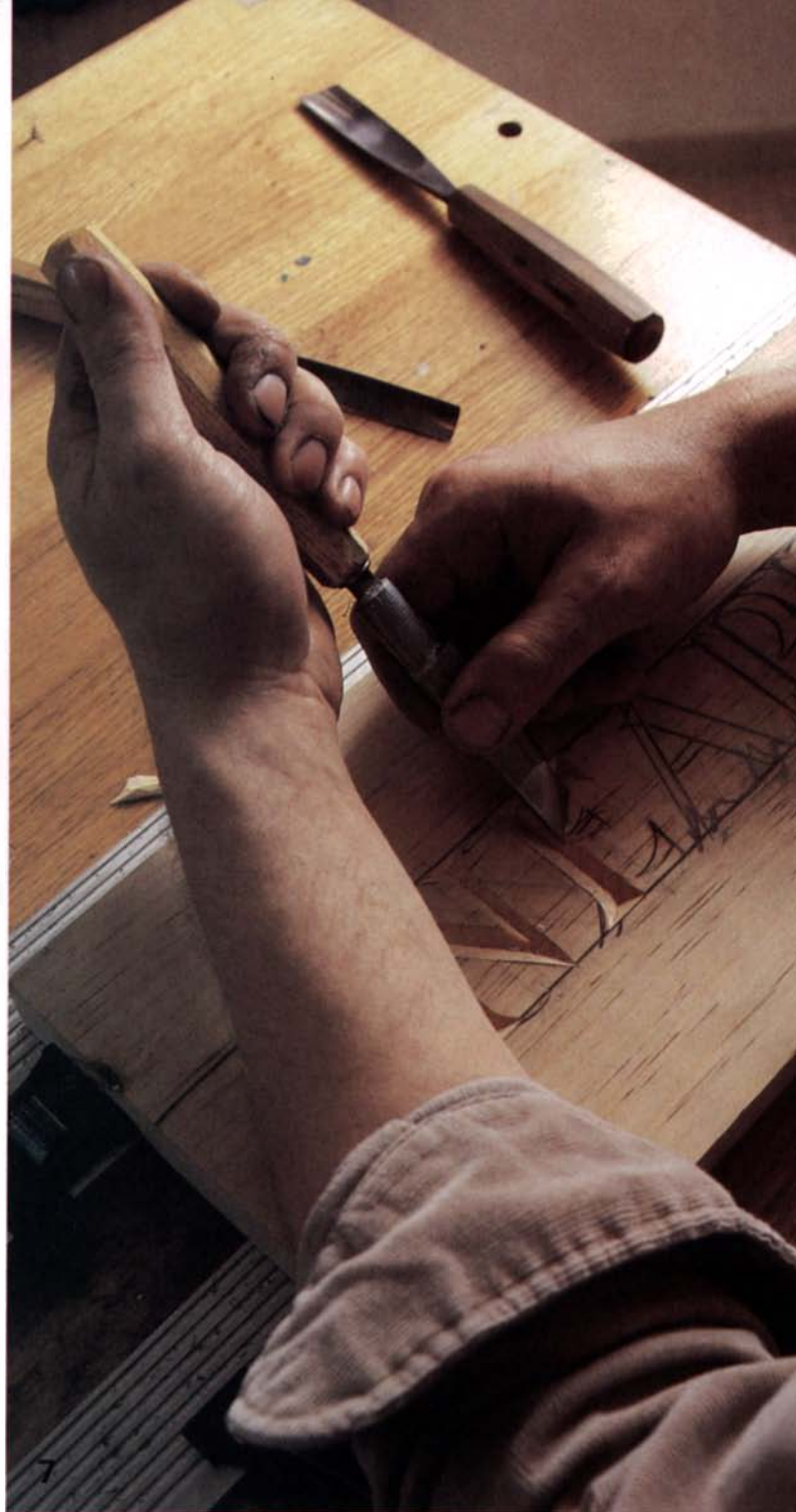
To avoid cutting against the grain on a diagonal cut (above), reverse the skew and push it away from you. Cushwa uses the hand position at right to make the top cut of a horizontal letter stroke.
