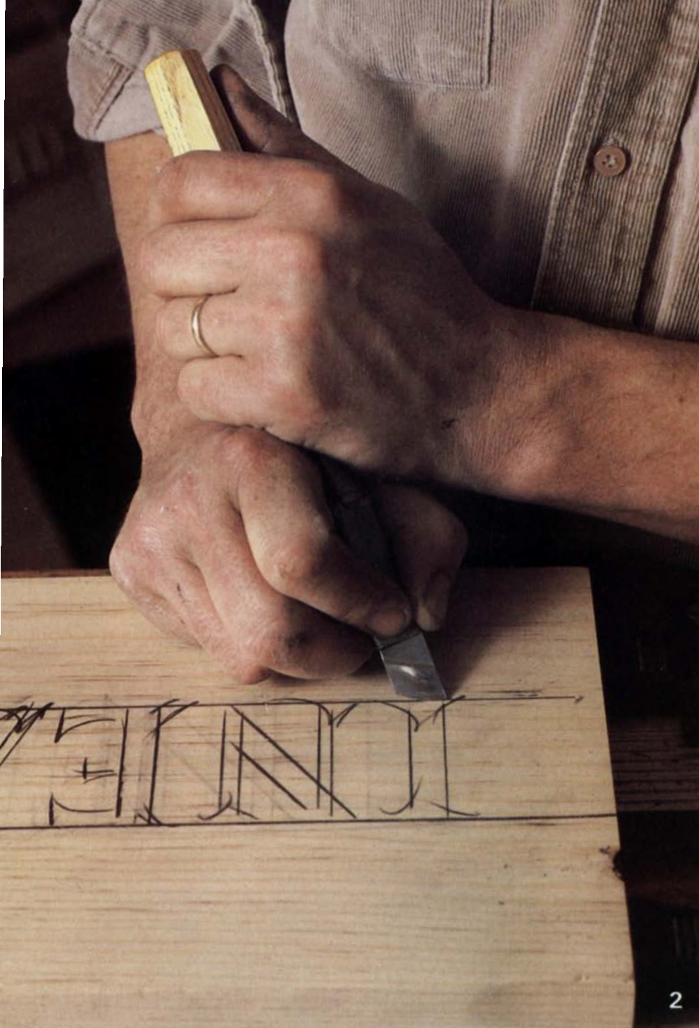
Three basic hand positions are shown here as Cushwa sets in and makes two vertical straight cuts for an I. Some trimming with the skew completes the letter.
