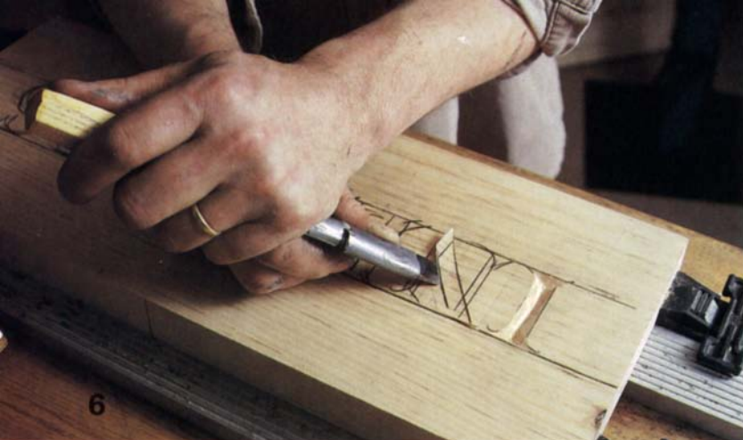
To avoid cutting against the grain on a diagonal cut (above), reverse the skew and push it away from you. Cushwa uses the hand position at right to make the top cut of a horizontal letter stroke.
