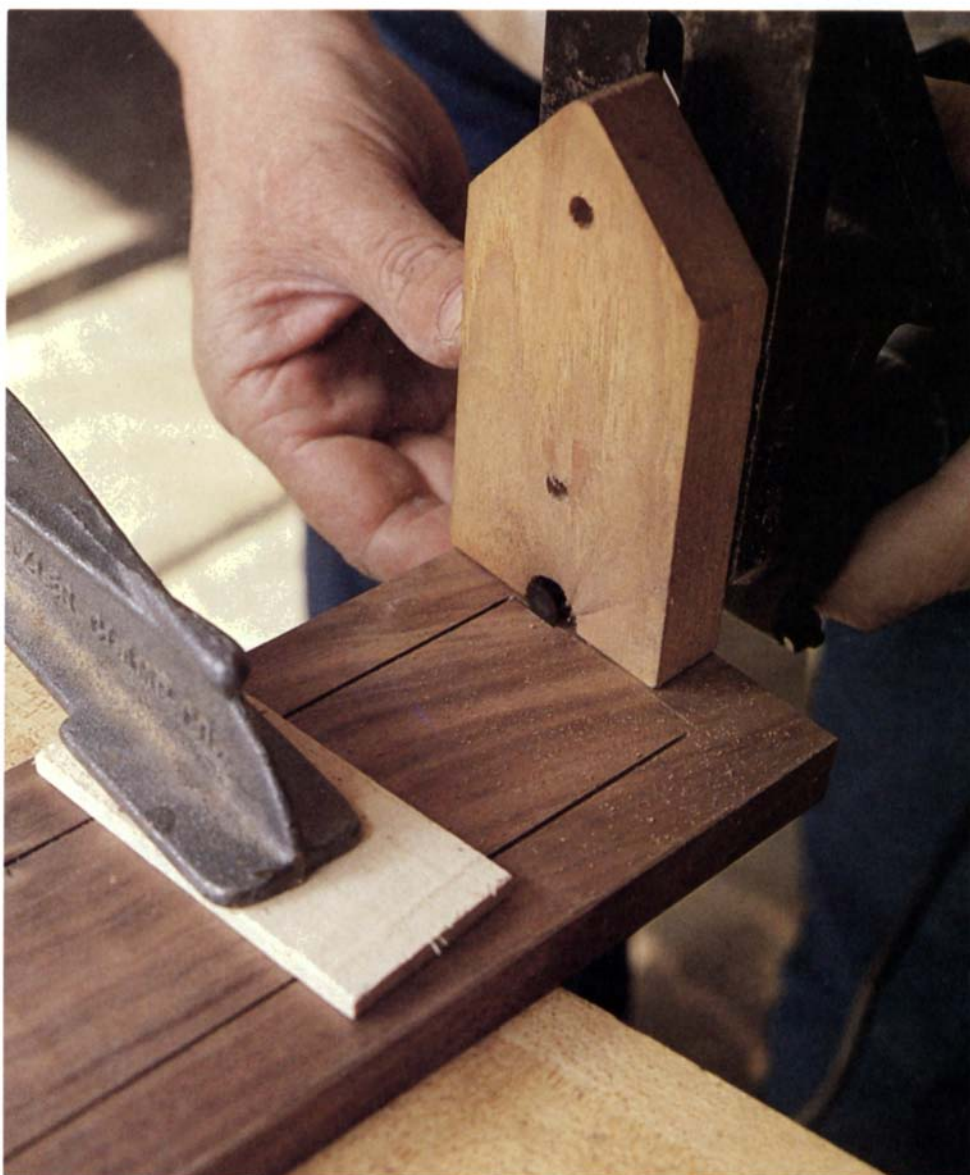
A tool-and-die makers' rotary grinder, left, mounted on shop-built stand cuts the inlay grooves. Shaped blocks can be attached to the 6-in. by 3-in. stand to guide the tool against a fence or curved template. To cut ½-in. slots for inlay, Pine mounts a small Dremel circular saw in the grinder. The wooden block around the blade sets the depth of cut, and the base of the stand bears against the edge of the piece being cut.
