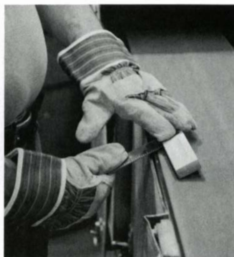
Stanley's best carpenter's squares are hand-hammered to tolerances of 0.005 in. in 15 in. of tongue length. Lew Levine first flattens the tongue on an anvil of end-grain maple, above. Then he trues the square by hammering it as shown in the drawing. A dial-indicator setup similar to Economaki's measures run out. Abrasives (right) play an important role in squaremaking. After the blades are riveted at Stanley, they're sanded flush and sharp metal edges are eased on a large beltsander.
