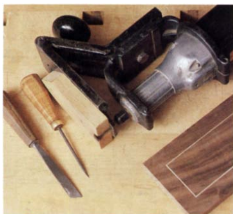
A tool-and-die makers' rotary grinder, left, mounted on shop-built stand cuts the inlay grooves. Shaped blocks can be attached to the 6-in. by 3-in. stand to guide the tool against a fence or curved template. To cut ½-in. slots for inlay, Pine mounts a small Dremel circular saw in the grinder. The wooden block around the blade sets the depth of cut, and the base of the stand bears against the edge of the piece being cut.
