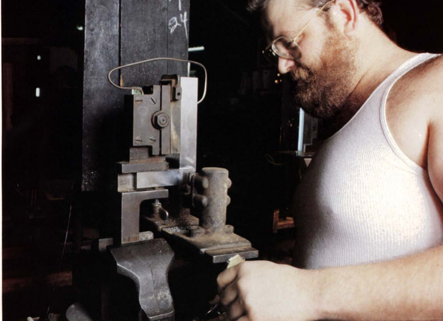
At Starrett, blades are soldered not riveted to the beams. Scott Songer, above, heats both sides of the beam with a dual-tip burner then feeds solder in as the joint warms. Once soldered and quenched, he tests the soundness of the joint by gently tapping the flat of the blade on his vise. A bright, tuning-fork ring indicates a good joint and the square is ready for testing.
