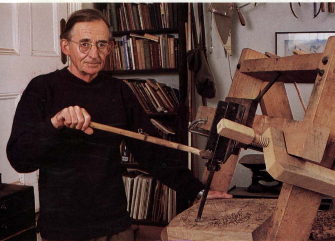
Pye carves bowls and dishes, like the wych-elm dish above, with the fluting engine shown below. The blank is fastened to an indexed turntable; the gouge moves from the edge to the center of the blank.
