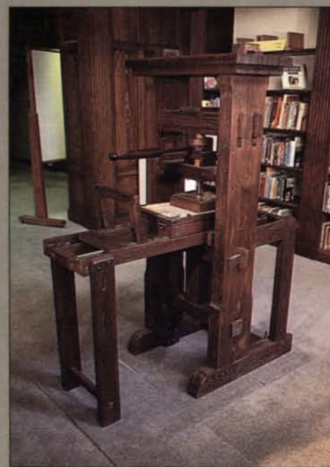
Finding no dies large or coarse enough, Lewis McClure, left, hand-carved the wooden screw for his replica of the Gutenberg printing press.
