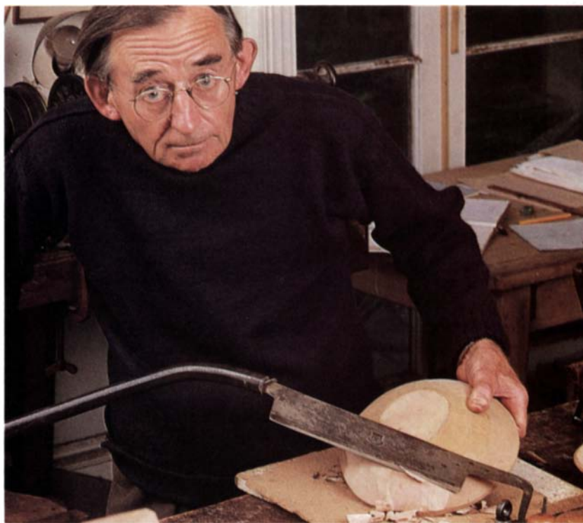
To shape the outside of his bowls, Pye uses his version of a clog-makers' block knife. The 18-in. dia. dish below is made of wild service tree.
