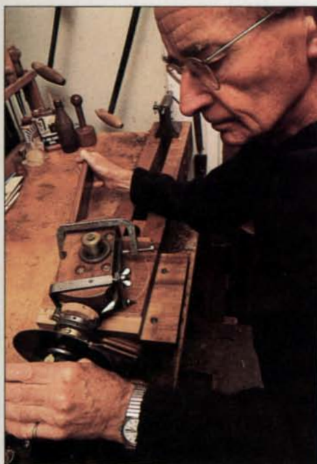
Pye engraves on the lathe with a smaller fluting engine. The pearwood box below is turned inside, carved outside.
