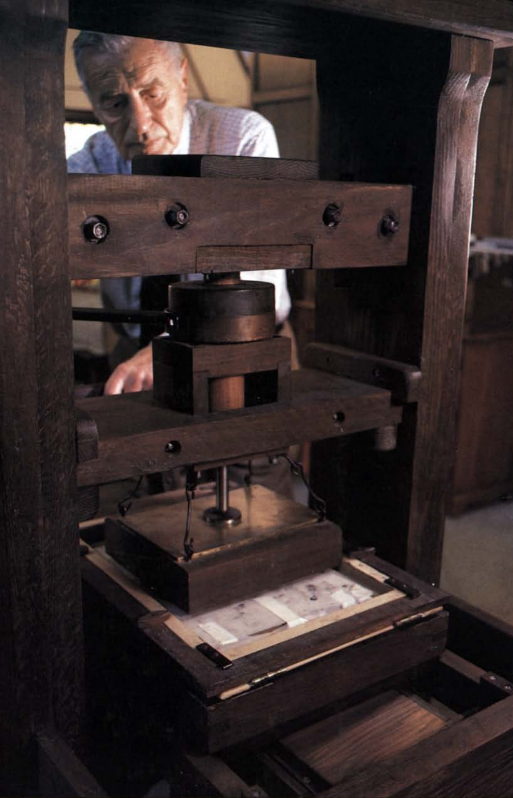
Finding no dies large or coarse enough, Lewis McClure, left, hand-carved the wooden screw for his replica of the Gutenberg printing press.
