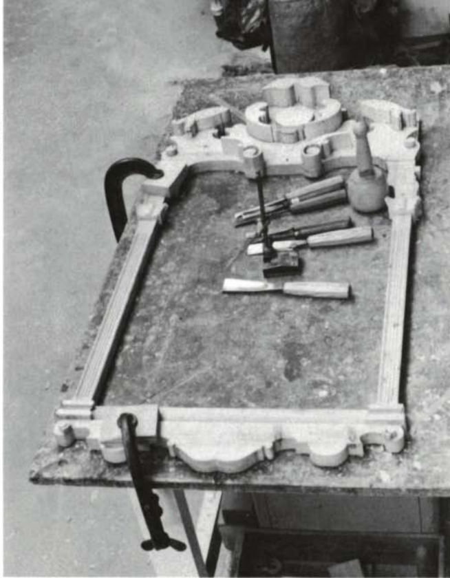
Shaped wooden blocks (above left) make the basic frame thicker in areas where ornamentation will be carved. When the frame is nearly finished, Bacon uses a small veining tool to recut the fine fluting into the gesso (above right).
