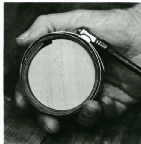
Wrap a strip of 80-grit sandpaper around the outermost strip of wood, then bend three steamed strips around the spiral puck. A hose clamp holds the strips in place while they dry.
