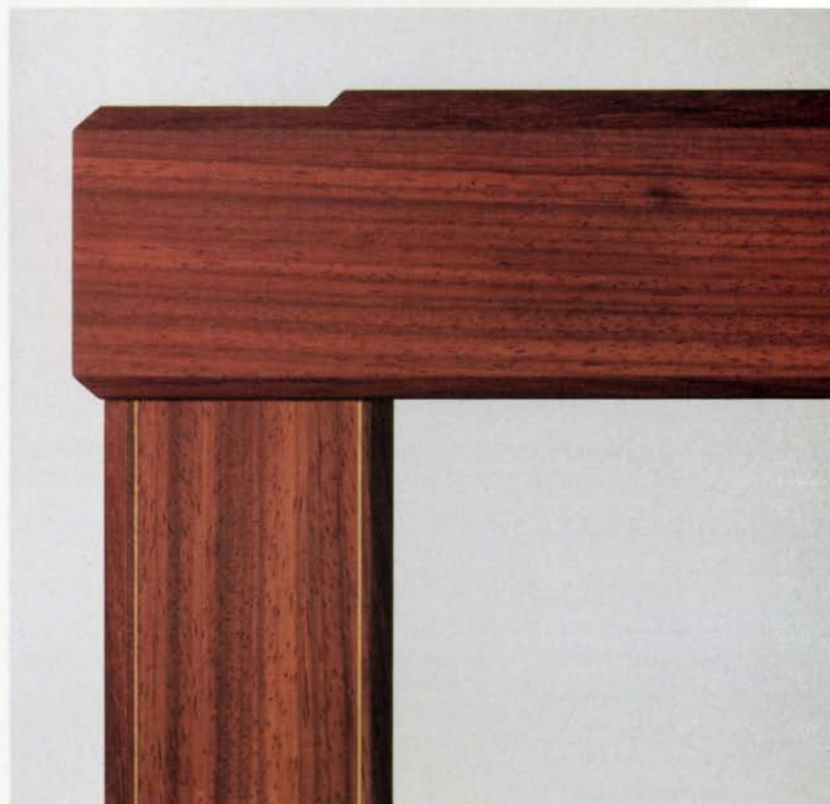
The mitered chamfer on Joe Wilson's padauk buffet is accentuated by satinwood inlay, which joins the chamfer, leg and top. Satinwood is also the primary wood in the raised window-like grid.
