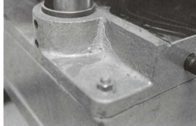
Though generally improving, copycat quality is hit-or-miss, especially in detailing. The photo above shows painted-over sand and dross in the fillets of the Taiwanese planer's table casting. The photo below shows the same detail on the Rockwell original.
