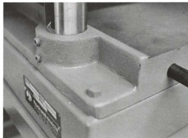
Though generally improving, copycat quality is hit-or-miss, especially in detailing. The photo above shows painted-over sand and dross in the fillets of the Taiwanese planer's table casting. The photo below shows the same detail on the Rockwell original.
