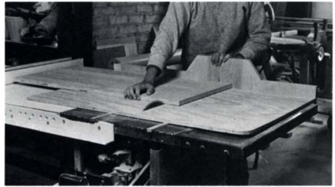
Taylor crosscuts panels on her Sears tablesaw, using a shopmade cutoff box. For larger cuts, she feeds sheets against a Biesemeyer fence, which permits cuts to the center of an 8-ft. sheet.
