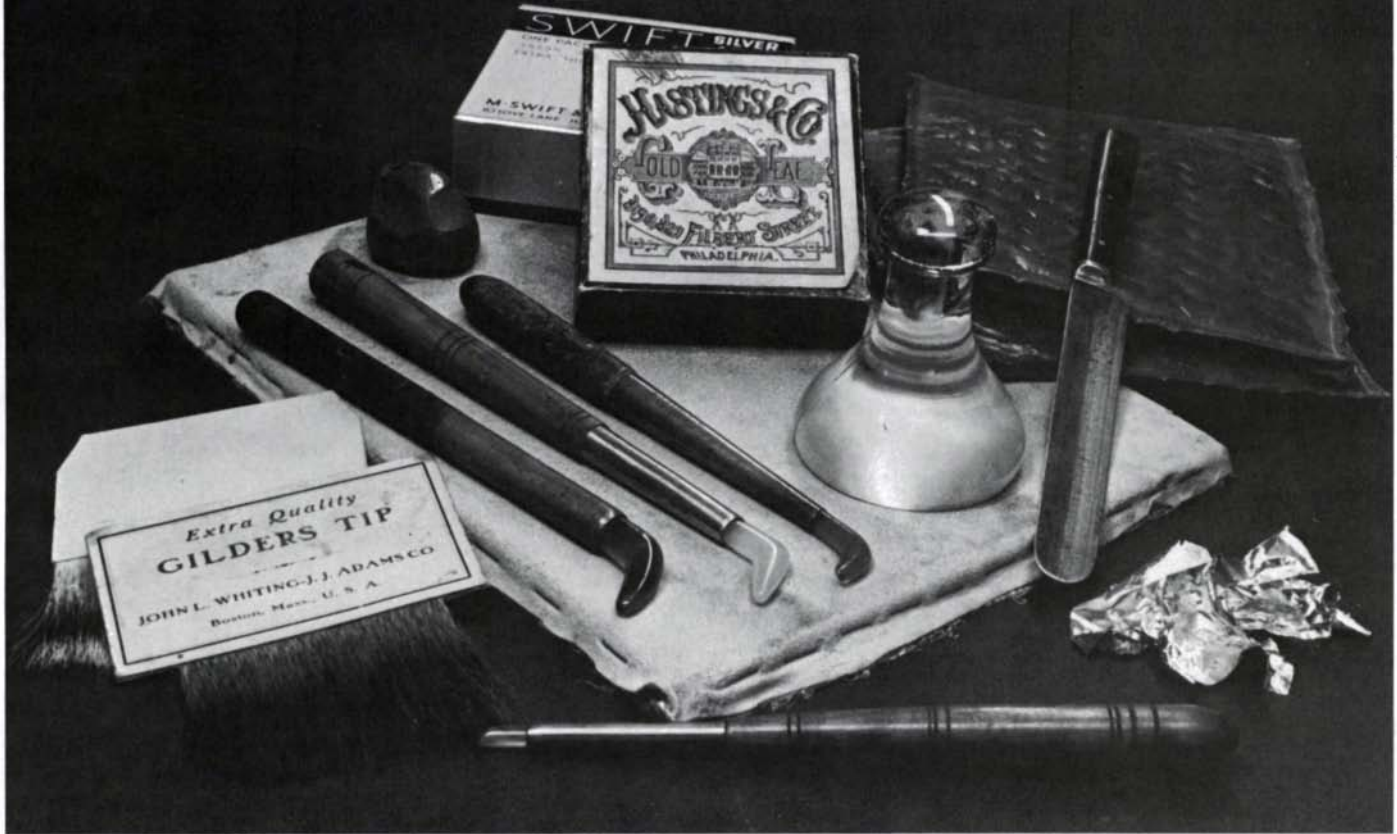
Leaf can be cut on a leather pad with a smooth-edged knife, whose handle here rests on some sheets of rabbit-skin glue. Also shown are agate burnishers, boxes of leaf, and a pestle for grinding lump clay, a piece of which sits at the back of the pad.
