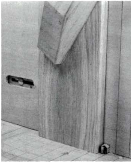
To cut first slot, clamp board vertically against jig face (left), right-hand edge against locating pin. First slot, placed over pin, locates next cut. Pencil lines on jig and router table make it easy to square up board. Bolts in jig face allow sideways
