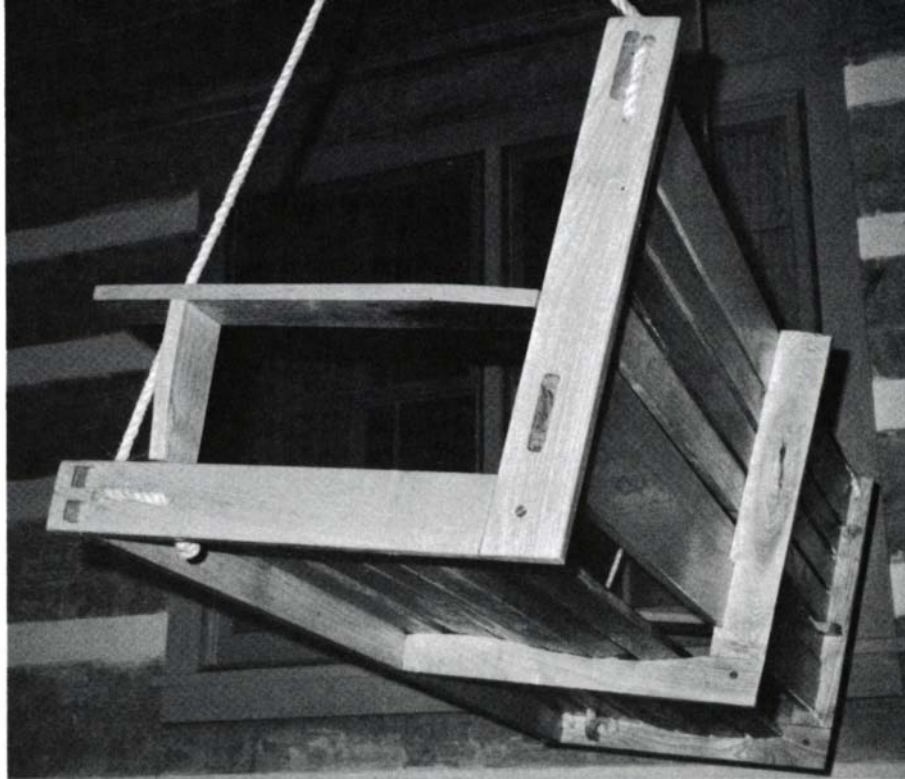
On the facing page, Carter explains how he made this porch swing. This end view shows joinery details, how he curved the seat, and the positions of the rope holes.
