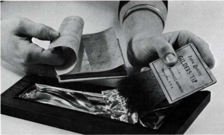
The gilders' tip picks up and transfers the gold from its padded book. A beginner may instead opt to use 'patent gold' (where each leaf comes lightly adhered to a sheet of paper), or to press waxed paper over the leaf for easier handling. The piece here, part of a table by Sam Bush, is shown as it would look being patched after burnishing.
