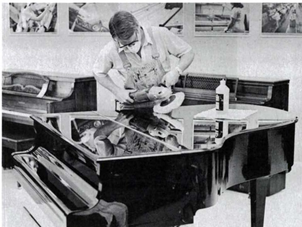
Steinert polishes built-up lacquer by hand or with an automotive lamb's-wool bonnet. He starts with medium-grade compound, finishing with a fine-grit called swirl-mark eliminator.
