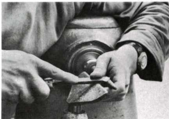
Supporting the work: Any grip can be modified by extending fingers around the work to the back side to keep the wood from flexing (top left). Note how Raffan steadies his body on the lathe in the photo at left. To back up the thin wall of a bowl, above, Raffan uses his left-hand thumb to pin the tool to the rest, while the other fingers support the wood behind the cut.
