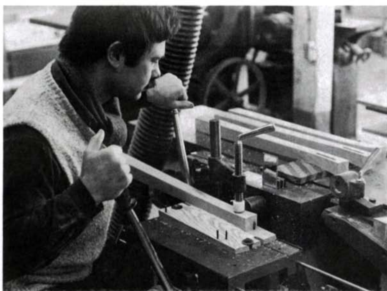
To mill angled mortises in 200 legs, Tracy bolted a 4° ramp to his Steton Combinata. A mirror taped to the machine lets him view the action.
