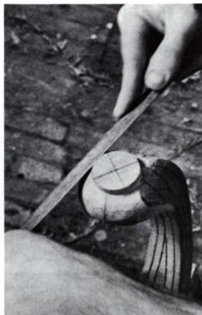
The steps for shaping the underside of the leg yield a round pad and a rounded foot.
