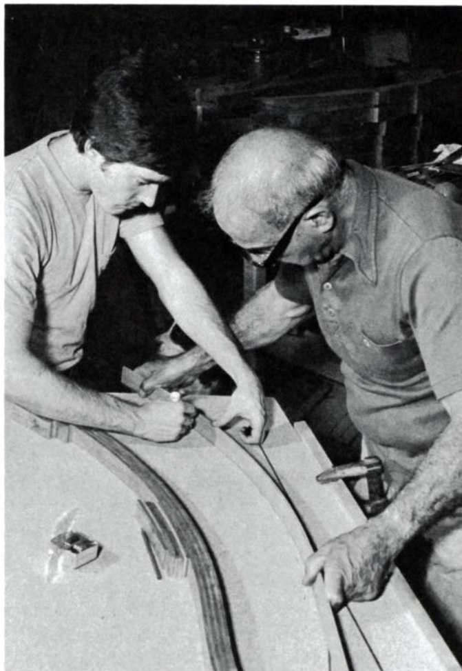
With assistant Mike Johnson tracing the curve, Maloof demonstrates how he casts the shape of a rocker on the piece of particleboard that will be its gluing form. Also shown is the glued-up blank, with platforms for smoothing the transitions between legs and rocker, ready for shaping.
