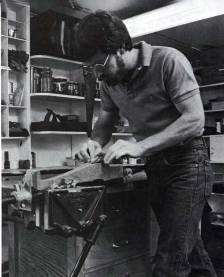
A pipe clamp mounted in the bench vise, above, makes an ideal holding arrangement for working the length of the leg. Here a spokeshave fairs the bandsawn curves, in preparation for the modeling layout.
