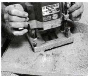
For tabletops, a pivoted router is a safe alternative to the lathe.
