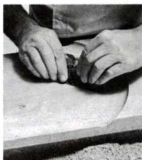
For tabletops, a pivoted router is a safe alternative to the lathe.
