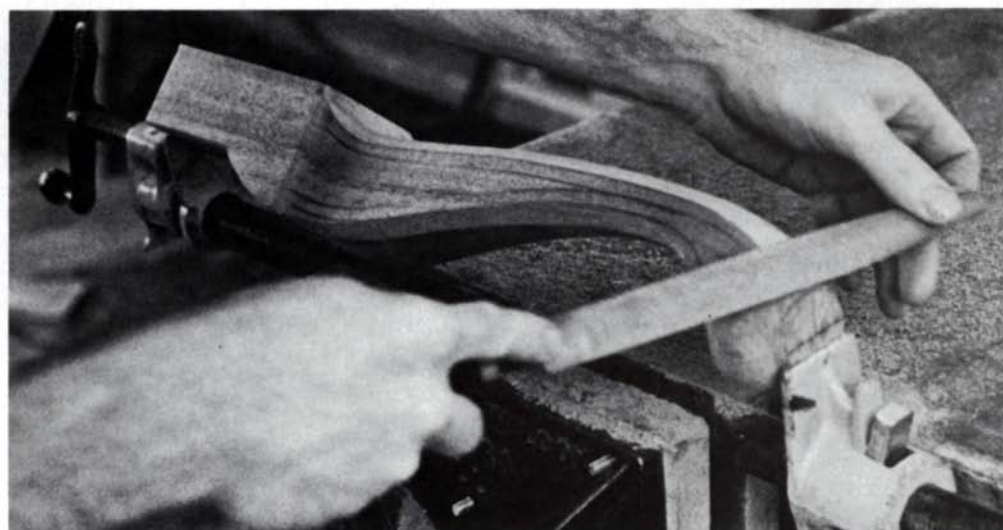
A rasp chamfers the corners of the leg to the outside layout lines, then rounds the leg to the inside layout lines, as detailed in figure 4.
