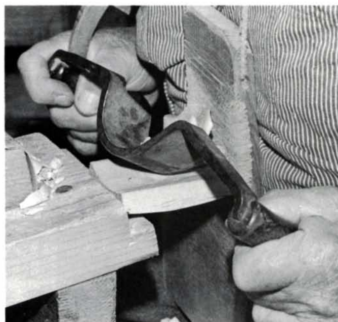
To shave short staves, cooper Ruedi Kohler supports one end of the blank in a rabbit on the front of his shaving-horse ledge, the other against a wooden bib.
