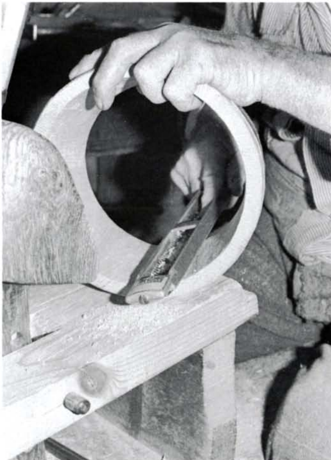
The staves are test-assembled and temporarily held in place with two metal hoops, so that the inside of the cylinder can be smoothed either with a convex-sole plane, as on the front cover, or with a Surform, above.
