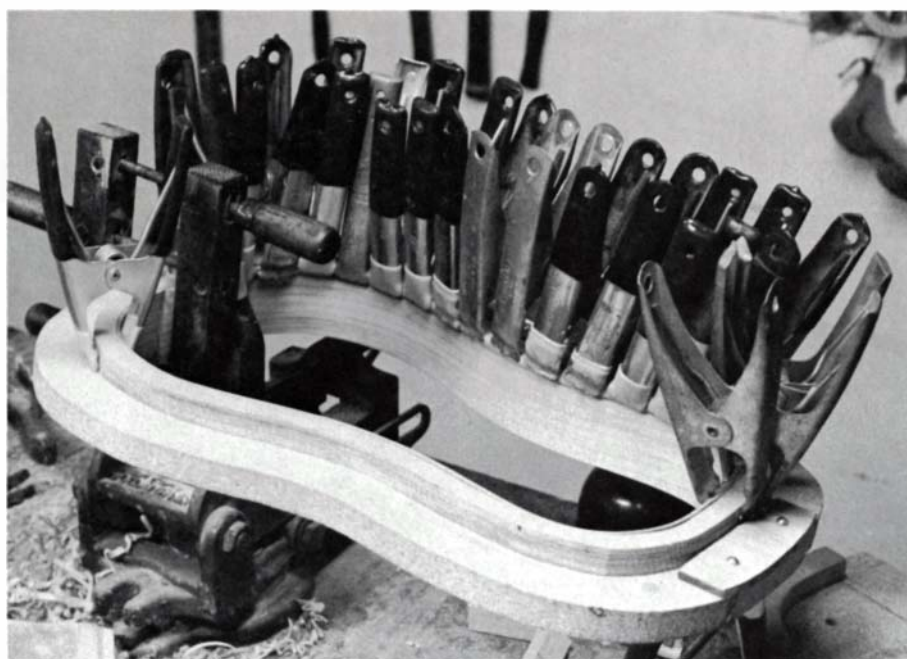
The assembly form: Pre-bent sides and linings are laminated with spring clamps, while the handscrew secures the tail block. The top block will be glued in last.
