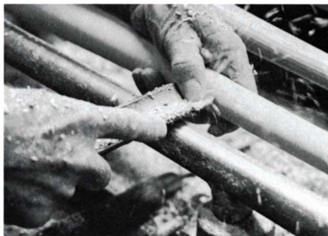
To keep the slender handle of a light bat from breaking, Young steadies the spinning work by hooking his left hand behind it. The thumb presses the gouge to the tool rest, ensuring a precise shearing cut that leaves a smooth surface.
