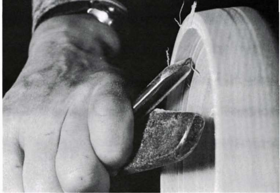
The tools at left were made by regrinding standard carvers' and turning gouges. Smoothing gouges (upper four) have an edge more curved than the edge of roughing gouges (lower two). Above, a gouge smooths the inside of a bowl.
