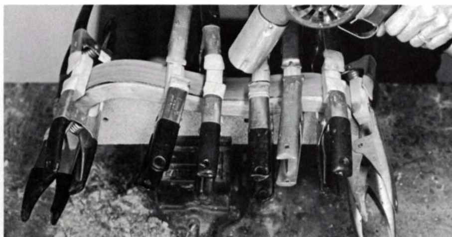
The bending form: Linings are first steamed, then clamped and heated with a hot-air gun or a gas flame to set the bends. Guitar sides can be bent the same way.
