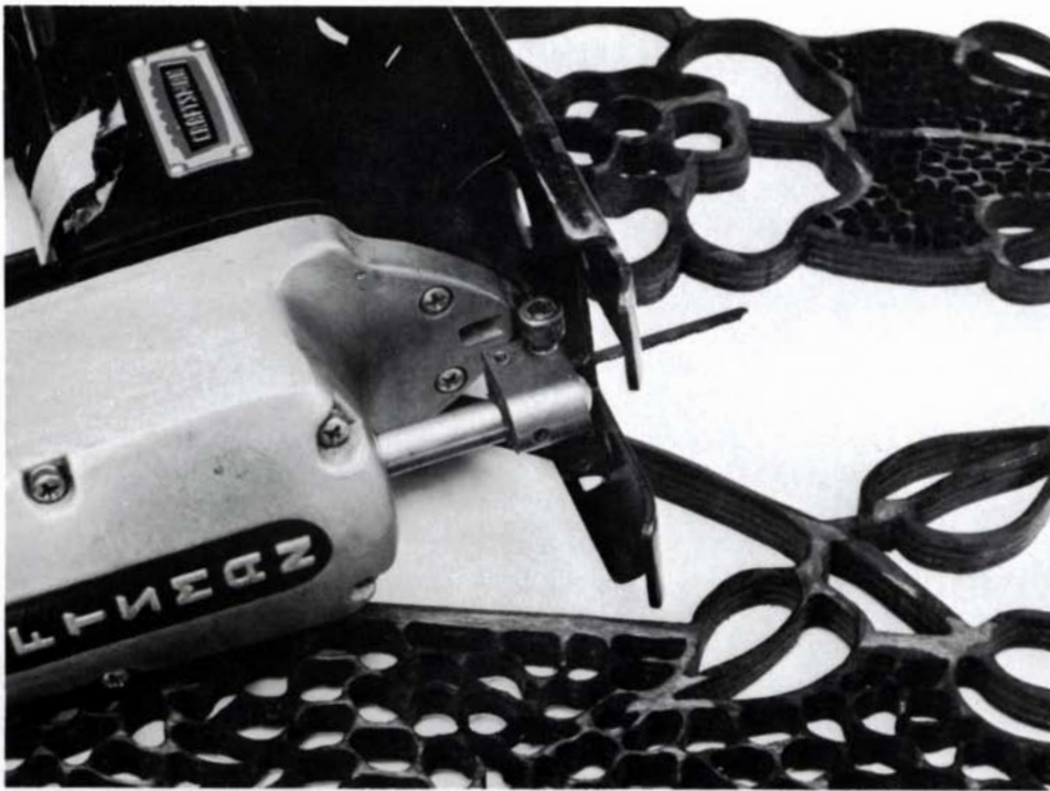
For the tight curves pictured above, Pessolano makes narrow, set-tooth blades by grinding standard blades (right) and mounting them upside down in a blade holder modified to take a larger setscrew. The blades cut on the downstroke, limiting tearout to the back of the plywood. A shim made from a broken blade spreads the blade holder's clamping pressure.
