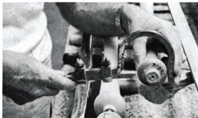
Above, turner Freeman Young sets his sizing tool to the model bat's knob diameter. He'll size the knob on the new bat and then shape it with a small gouge.
