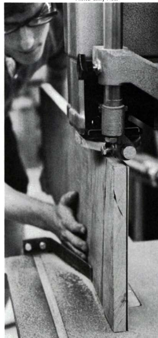
Both resaws tested (Makita, left, and Hitachi, right, in the photo above) are surprisingly small. The saw tables are about 30 in. above the floor, a working height that makes it easier to balance the kind of heavy timber these machines are designed to cut. Blade guides are similar to those of conventional saws. The Makita 2116, top left, has two Bakelite guides adjusted with wing nuts. Those of the Hitachi B600A, bottom left, are similar, though slightly beefier. These saws will cut boards up to 12 in. wide; in the photo at right, Preiss uses the Hitachi to slice a 1/8-in. thick piece of veneer off a wide plank.
