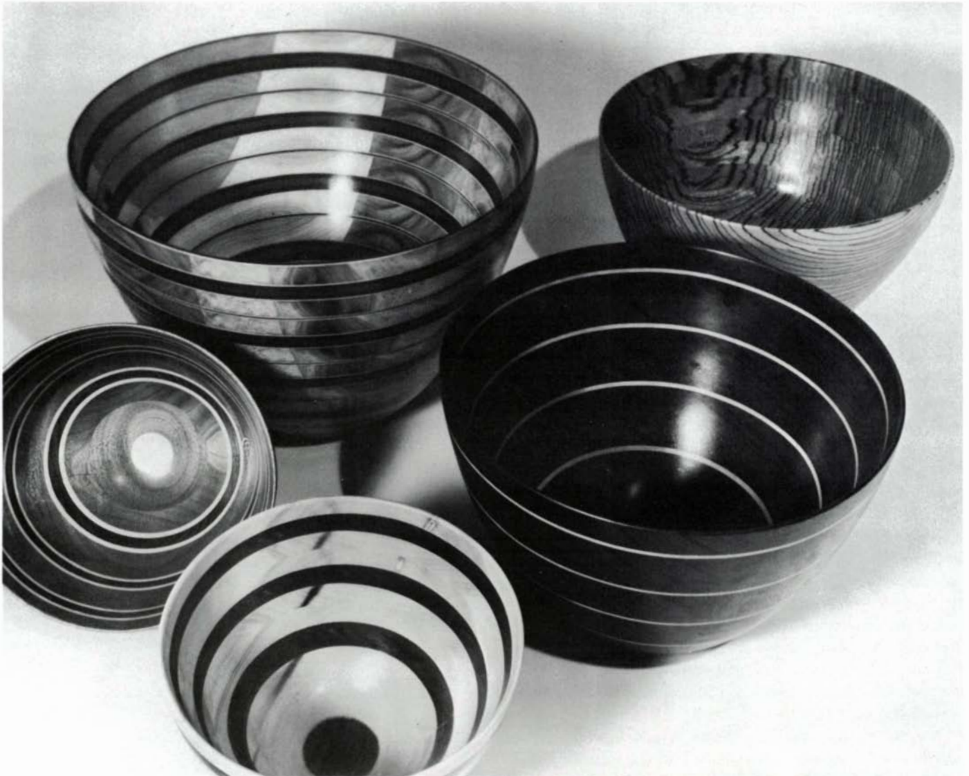
These bowls came not from the lathe but from single, flat boards that were bandsawn into tapered concentric rings and glued together before being shaped with abrasive discs. The bowls can be of one kind of wood or of several contrasting woods.
