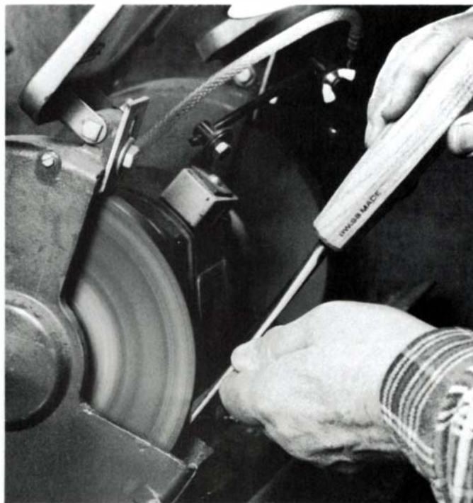
After grinding, Riordan buffs a secondary bevel onto his tool edges, using a hard felt wheel charged with gray compound. He holds the tool so rotation is away from the edge, otherwise the wheel might catch the edge and hurl the tool.
