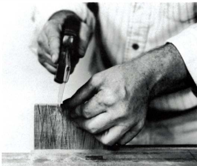
To saw dovetails, clamp the workpiece upright in the vise, and hold the saw to match the tail and pin angle. Guide the cut with your thumb and, keeping the saw flat in the kerf, saw down to the line marking the base of pins and tails.
