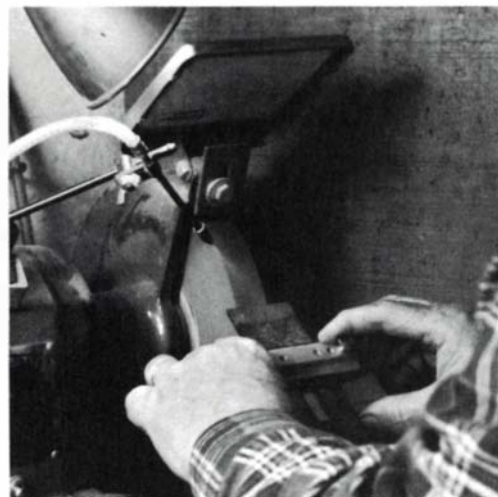
Riordan's full rig consists of an 8-in., 36-grit aluminum-oxide wheel, a misting device, a rest that maintains the proper angle, and a hard felt wheel. To sharpen plane irons, below, he uses a tool holder that slides parallel to the diamond-dressed face of the wheel. The safety shields have been lifted for the photos.
