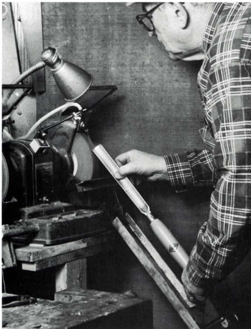
Riordan rotates a gouge, supported by an adjustable V-block, until the bevel is evenly ground. A misting nozzle directs its spray at the cutting edge. Mist, together with a light touch, keeps things so cool that there are hardly any sparks.
