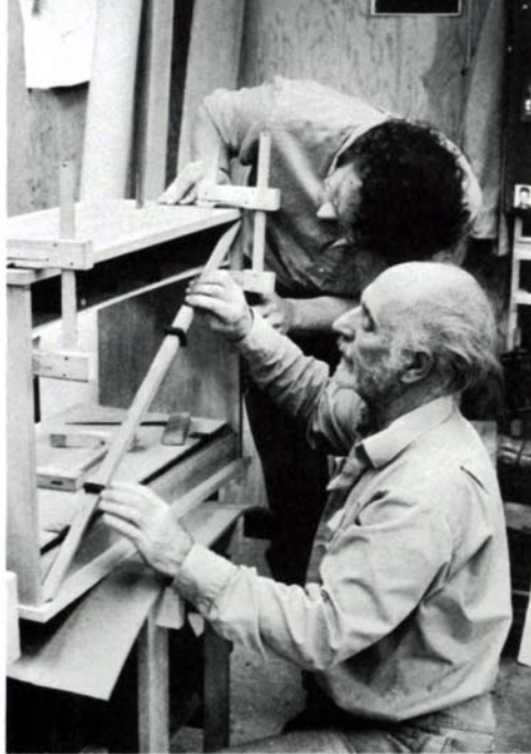
College of the Redwoods students can make what they like, including complex case pieces such as this pearwood desk that Krenov, left, helps maker Creighton Hoke check for square.
