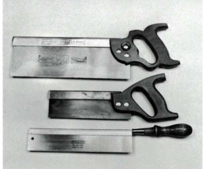
The fine teeth and thin blade stiffened by a brass or steel back make the backsaw an ideal joint-cutting tool. Backsaws are of two types: the larger are called tenon saws, the smaller are dovetail saws. Shown above are a 12-in. English-made brass-backed tenon saw, an 8-in. dovetail saw, and a 7-in. dovetail saw with the straight turned handle preferred by some craftsmen.
