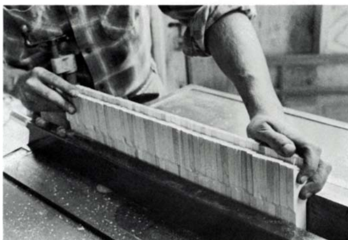
Stacks of parts are dadoed in a 'chute' composed of the tablesaw fence and a length of wood clamped to the table.
