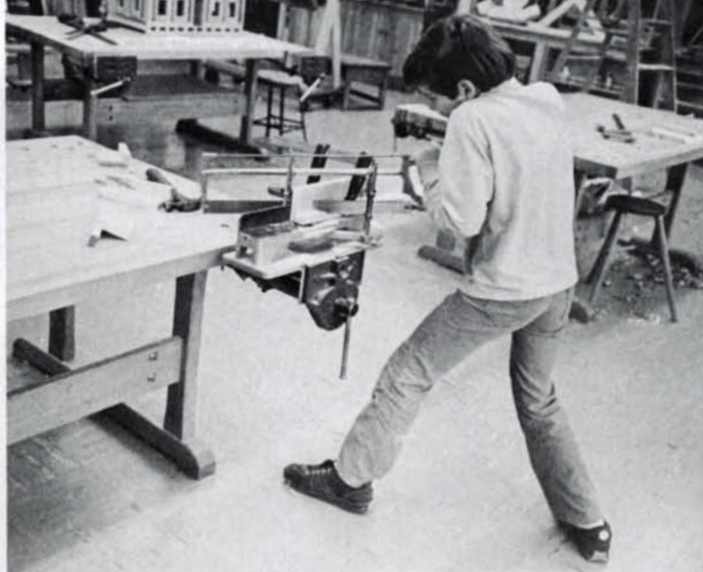
After Starr rips the sides for the hockey board on his radial-arm saw, he has the kids nail and glue ledger strips to the bottom edges, left. Children should be reminded not to put nails too close to the ends of the boards, to avoid sawing through them when the sides are mitered. At first, mitering is confusing for children, so Starr hangs a mitered mirror frame on the wall as a teaching aid. Above, a fifth-grader saws a miter on one end of a board hockey frame.
