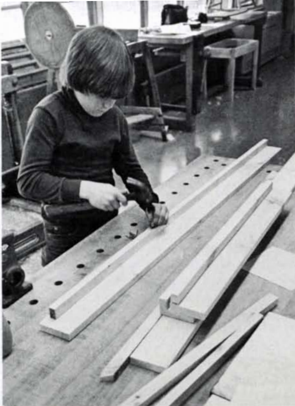
After Starr rips the sides for the hockey board on his radial-arm saw, he has the kids nail and glue ledger strips to the bottom edges, left. Children should be reminded not to put nails too close to the ends of the boards, to avoid sawing through them when the sides are mitered. At first, mitering is confusing for children, so Starr hangs a mitered mirror frame on the wall as a teaching aid. Above, a fifth-grader saws a miter on one end of a board hockey frame.
