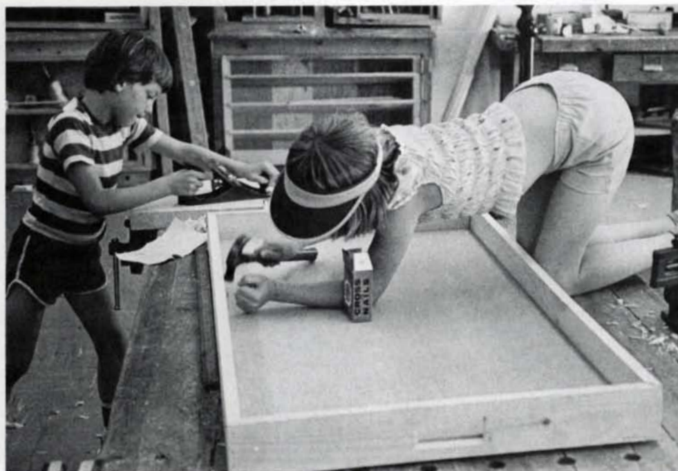
After Starr rips the sides for the hockey board on his radial-arm saw, he has the kids nail and glue ledger strips to the bottom edges, left. Children should be reminded not to put nails too close to the ends of the boards, to avoid sawing through them when the sides are mitered. At first, mitering is confusing for children, so Starr hangs a mitered mirror frame on the wall as a teaching aid. Above, a fifth-grader saws a miter on one end of a board hockey frame.
