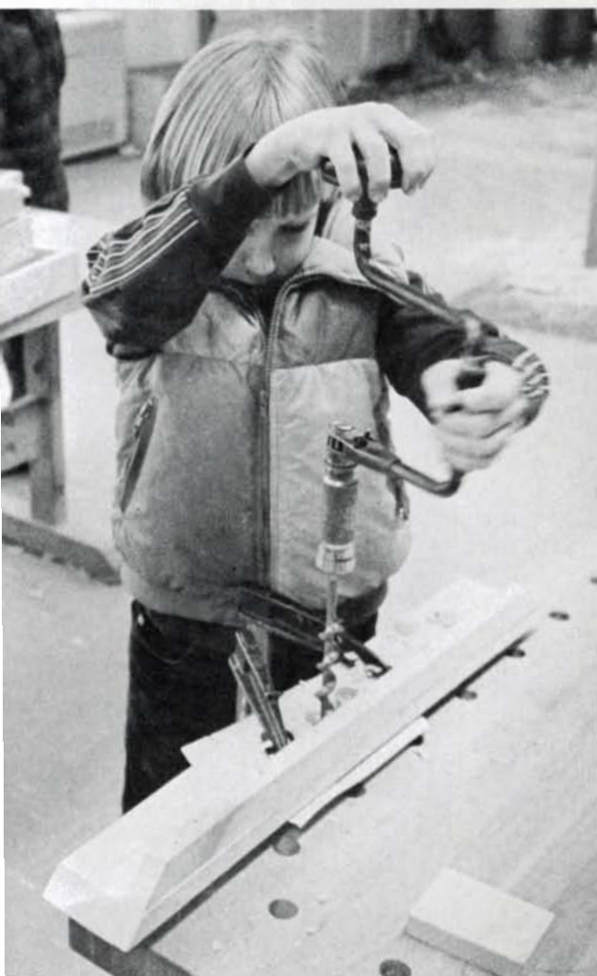
Making a board hockey game gives children a chance to learn several basic skills: sawing, boring, chiseling and nailing. Above, a second-grader uses an auger to hog the waste out of one of the hockey board's goal openings. He'll finish the job with a chisel and a file. Above right, a student nails the plywood bottom into the hockey board. The completed board, right, will be given a coat of shellac, followed by wax for a fast-playing surface.
