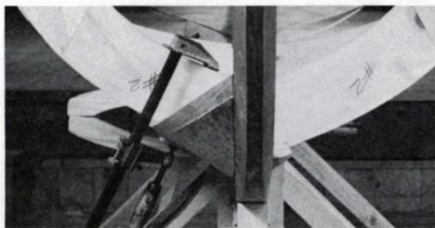
The boat's bottom plank, called the garboard, gets a considerable twist, which can be achieved only by soaking the end in boiling water, or steaming it, and clamping it in place to cool. This bow-on view shows how the stem is tapered back from its leading edge.
