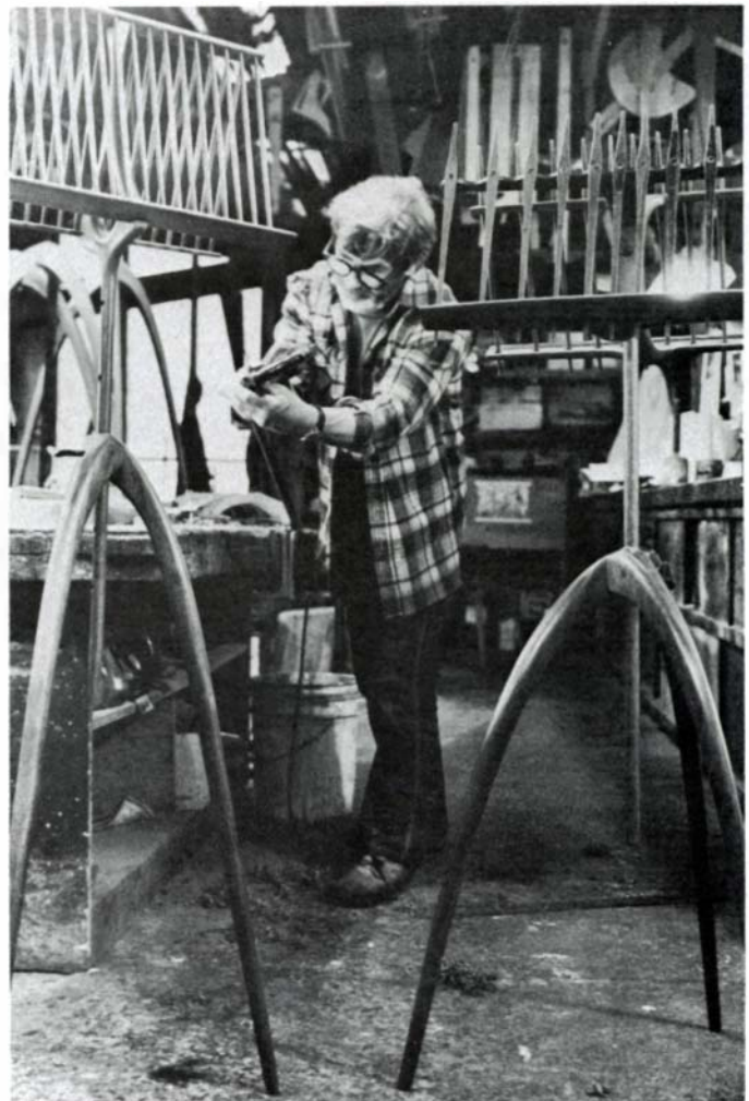
After routing, Carpenter shaves an upright for a run of music stands, the master for which is at right, an earlier version at left. He prefers doing small batches of furniture, up to 15, because he can get production momentum without getting bored.
