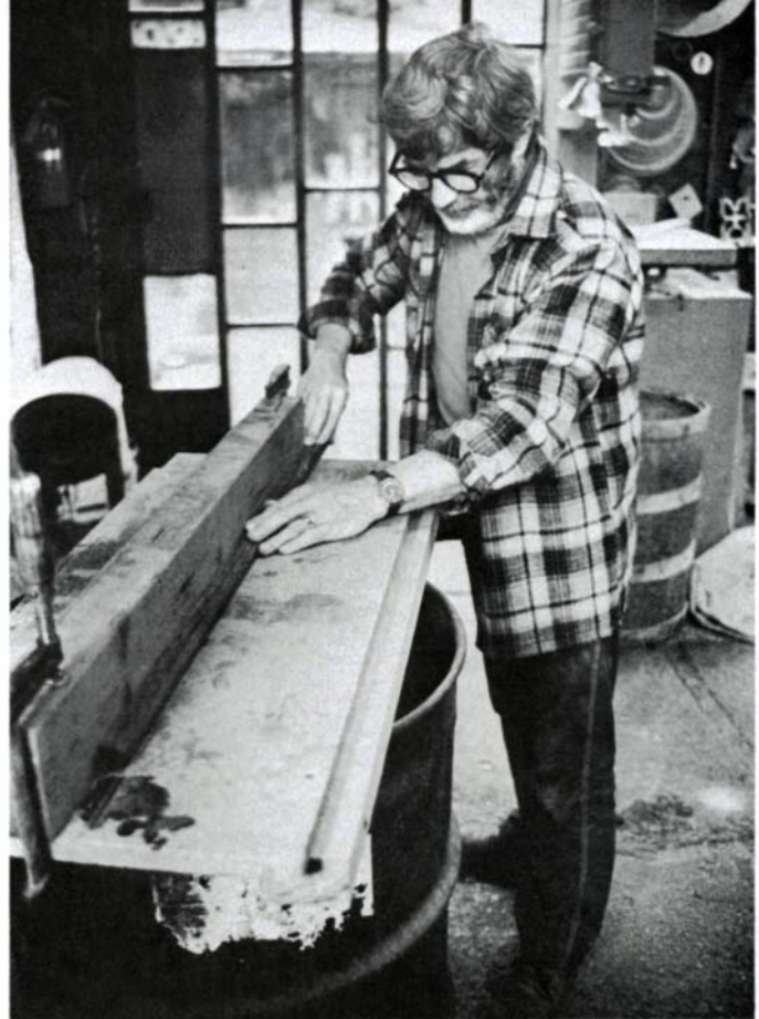
Carpenter's equipment is as modest as some of his designs. His router table is a piece of particleboard with router and fence attached, all placed on an empty oil drum, to catch shavings.
