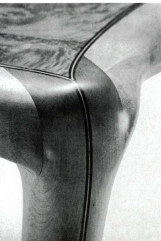
Sculptural furniture is frequently made of glued-up baulks of wood carved and sanded to shape. In this maple table, Charles Becker, of Philadelphia, combined that technique with veneering. The tabletop is maple burl veneer over particleboard. The legs are inlaid with sandwiched purpleheart and maple. Becker made the table specifically for showing at the Baltimore Winter Market.
