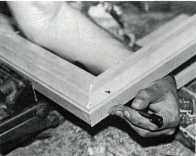
Free side of the frame must be hand-supported at all times until the corner comes out of the vise. Nails pull the miter as tight as it will go—tighter than a corner vise can be set.
