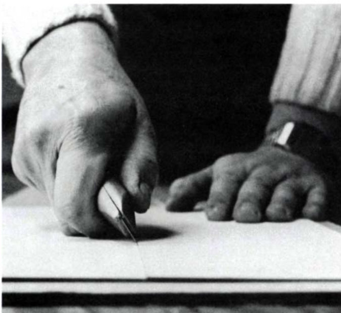
A mat cutter's grip presses the backs of the fingers against the surface to hold the bevel angle. Practice canting the knife until the blade travels straight, pulled by the entire body, not the arm. Once the grip is mastered, a straightedge can be used for peace of mind. Blades are cheap—use a new one for every mat.
