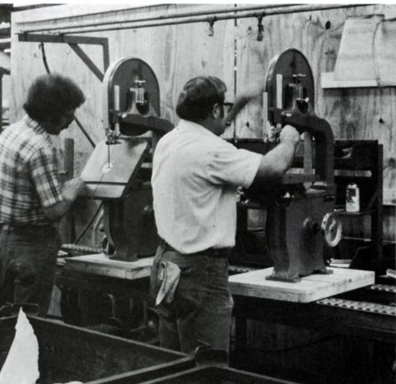
Above, at the end of a long assembly line, these workers in Rockwell's Tupelo, Miss., plant make the final checks on 14-in. bandsaws. One adjusts the blade-guide system, while the other sets the 45° positive stop on the tilting table. From here the machines go to be packaged and to await shipping.
