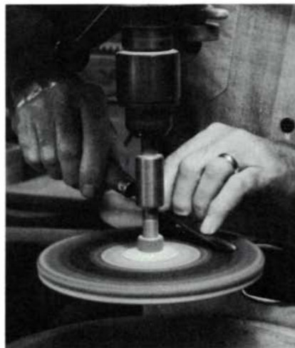
To make honing quick and tidy, Schramm constructed this rotary strop (above left) from plywood and leather. He mounts it in his drill press and charges the surface with white rouge, a simple arrangement for keeping a razor-edge on all his tools, without the mess made by oilstones. Pinwheel sander (above right), when chucked in lathe or drill press, is good for finishing contoured furniture parts like cabriole legs.
