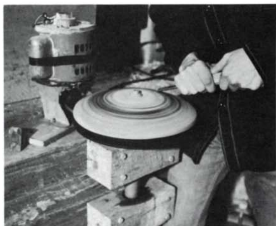
White's horizontal sharpening system, which rotates at only 300 RPM, can be fit with a grindstone, an abrasive disc or a leather-covered stropping wheel. An old washing-machine motor provides power.
