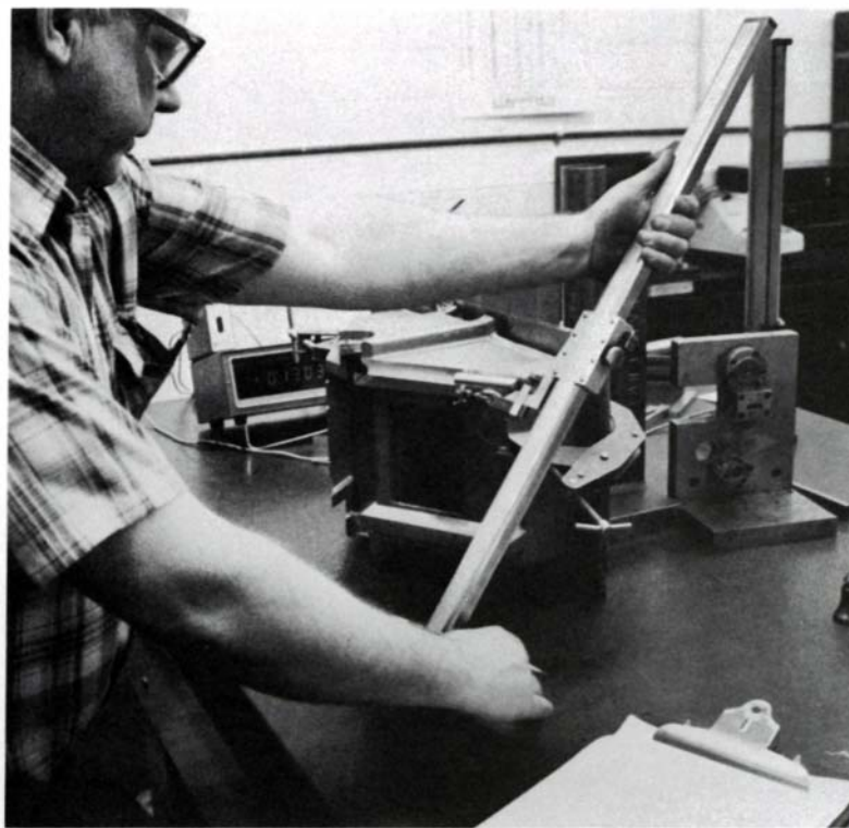
A quality-control engineer uses mechanical and electronic gauges to see whether the milled dovetailed ways in this base for a Rockwell 8-in. jointer fall within the prescribed tolerances. The engineers select bases off the line at random during the day. A test failure stops the run until the error is corrected. Rejected parts are re-machined or scrapped.
