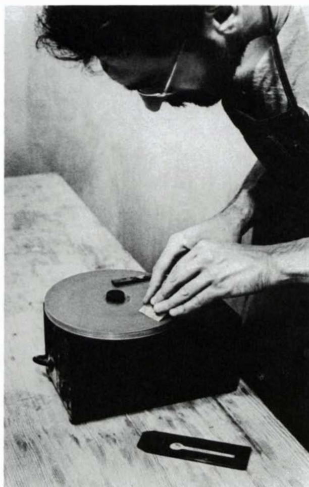
The Xenix Hone, left, is a motorized strop, using a slowly rotating plate composed of reconstituted leather mixed with rouge. The plate of the Belsaw Power Hone, above, is studded with 600-grit diamond dust.
