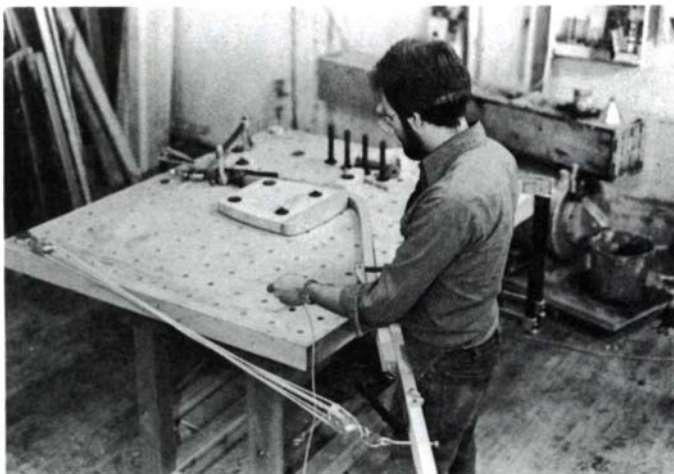
Above, Fortune begins to pull in the block and tackle for the first bend of a chair seat. The stock is first steamed in the plywood box in the background; steam is generated by a salvaged boiler containing a 4.5-kilowatt immersion heater. Below, with the first corner turned, Fortune slackens off the adjustable end-stop before levering the wood around the second bend.
