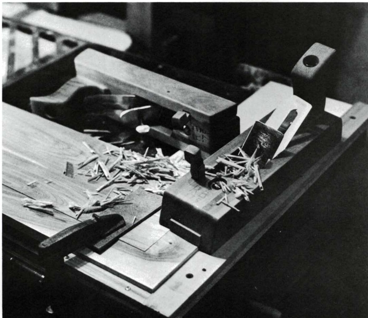
Tear-out from planing against the grain, always a problem when using a single panel-raising plane, is minimized by having two, a left-hand and a right-hand model. No matter how the grain runs, one plane or the other can follow it.
