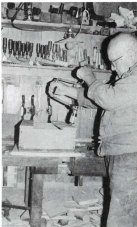
Kohler uses a wooden box with slots in boards across the top to jig his brace and bit to the proper angle for boring the leg mortises.
