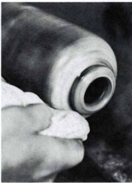
Author sands turning with orbital sander, above, which eliminates cross-grain scratches and does not dip into soft areas of grain, as does hand-held sandpaper. A thin strip of sandpaper backed with Mylar tape, above right, reaches places where the sander will not go. Turnings can be 'French polished,' right, by applying a shellac-and-oil mixture and rubbing it out with the lathe at high speed until the mixture has been driven into the wood.
