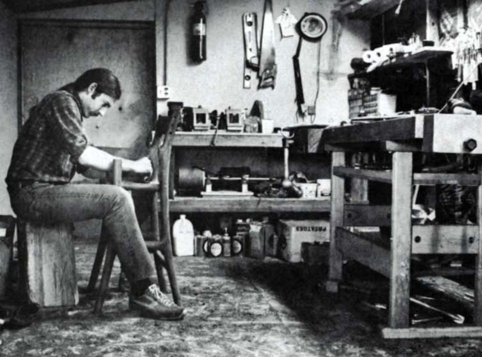
Craig Marks scrapes the seat of a rosewood high chair (left). Photo: Staff. Writing desk by Marks (right), 37½ in. by 23 in. by 29 in., Honduras rosewood and California walnut, was judged best in show at Thanksgiving.
