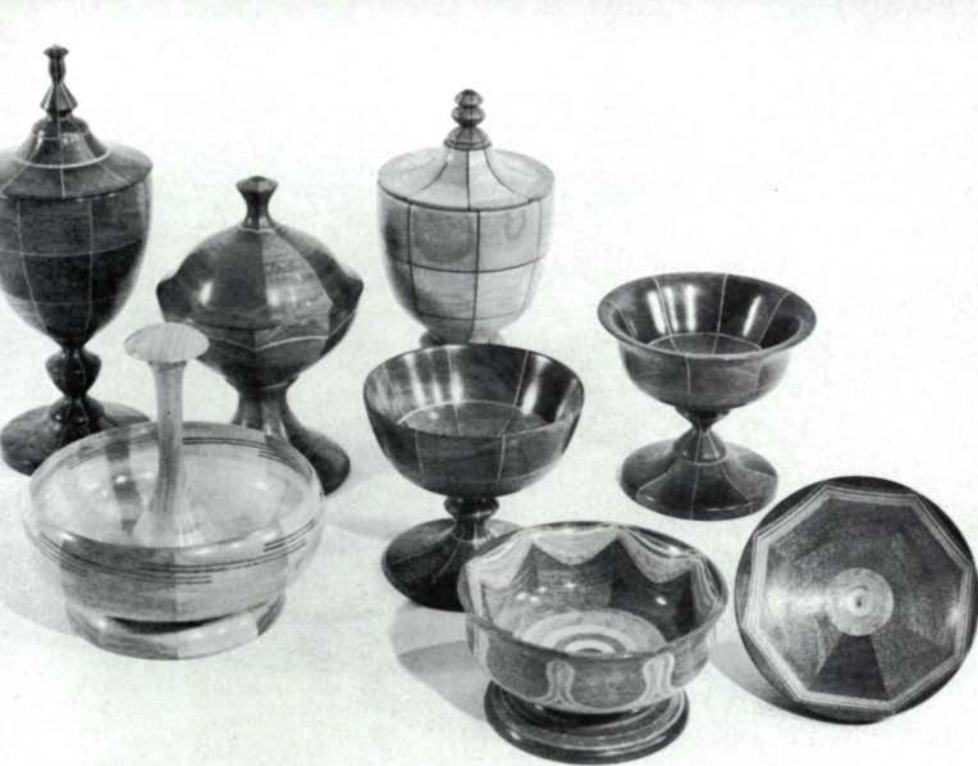
Barklow's geometric turnings begin as wood-and-veneer sandwiches that are segmented and glued up into octagonal turning blanks. Woods in the collection of turnings above are mainly walnut, basswood and maple. Detail of nut bowl is shown at right.
