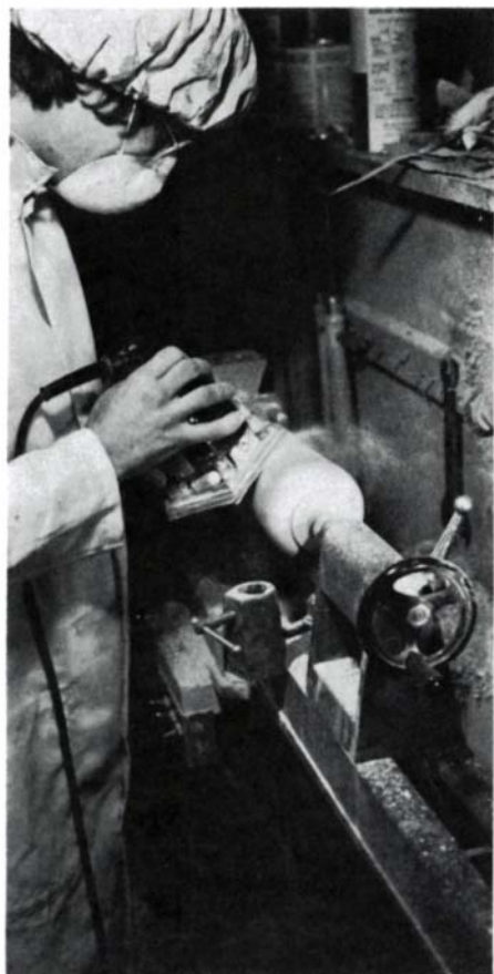
Author sands turning with orbital sander, above, which eliminates cross-grain scratches and does not dip into soft areas of grain, as does hand-held sandpaper. A thin strip of sandpaper backed with Mylar tape, above right, reaches places where the sander will not go. Turnings can be 'French polished,' right, by applying a shellac-and-oil mixture and rubbing it out with the lathe at high speed until the mixture has been driven into the wood.
