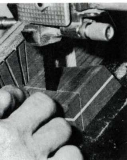
After gluing up a stack-board of wood and veneer, Barklow saws it into compound-angled segments, left. These are machined to precise angles on the disc sander, then rub-joined into turning-blank halves. He machines one of the halves before final assembly, center. Barklow also makes cufflinks and pendants, applying the principles of the turned veneer sandwich to little scraps of wood, right.
