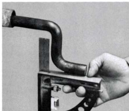
Fig. 6 (above): Crank rod is checked for squareness after being heated cherry red and bent into shape. Fig. 7 (right): Crank, take-up bearing, throw-rod and U-shaped coupling connect flywheel to lower arm of saw. Metal plate bolted to flywheel opposite crank acts as counterbalance.
