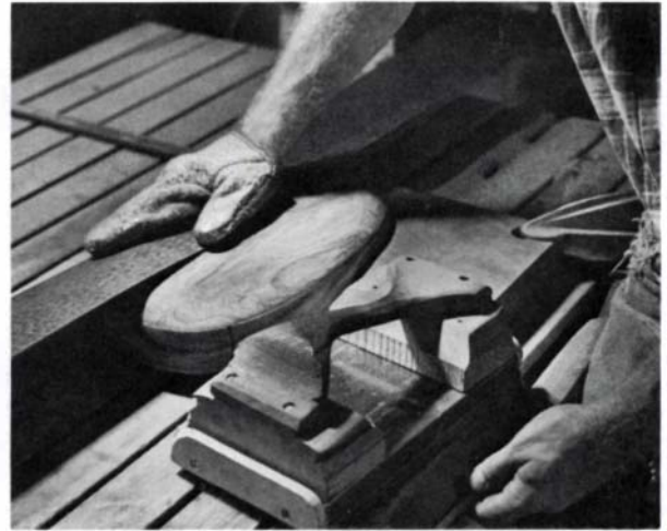
5. Because there are fewer and easier machine setups, the rest of the production run is divided into smaller groups so more attention can be given each box. Drawers are fitted to their carcasses and, after bandsawing the outline and rounding it over on the shaper, the top and bottom surfaces are crowned on the stroke sander. A padded, graphite-covered hand platen is used first, then a graphite-coated glove.
