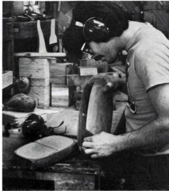
4. Parts are selected according to figure, and 4/4 top and bottom are glued to 8/4 carcass center. Using aliphatic resin glue for joint elasticity, the gluing surfaces are sized (precoated for maximum fiber penetration) and stacked in specially made egg-box clamp. Pressure applied evenly through threaded rods achieves optimum 0.002-in. glue line.
