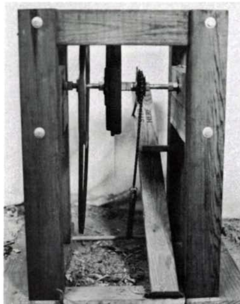
Maier's band saw, right, has frame, housing, column and table made entirely of wood. So this saw can be foot driven, a threaded-rod drive shaft fits into tapered roller bearings (above), which are mortised into cross members in frame. Drive pulley, flywheel and five-speed sprocket cluster were all purchased as used parts. It can, of course, be equipped with an electric motor.
