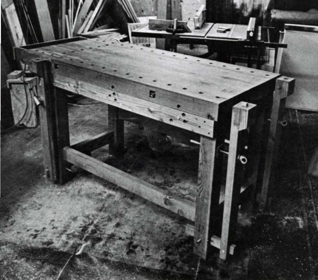
Three leg vises and three rows of dog holes give Schuldt's bench large holding capability. Side view of leg vise, right, shows threaded rod, pivot foot and steel strap stiffener.
