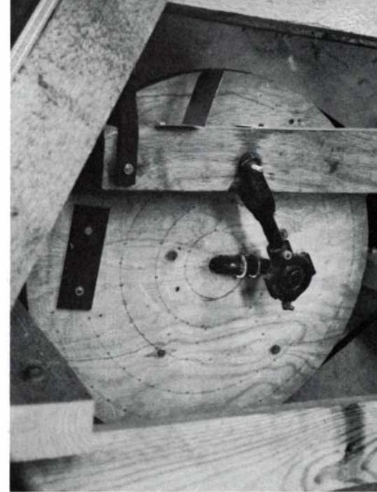
Fig. 6 (above): Crank rod is checked for squareness after being heated cherry red and bent into shape. Fig. 7 (right): Crank, take-up bearing, throw-rod and U-shaped coupling connect flywheel to lower arm of saw. Metal plate bolted to flywheel opposite crank acts as counterbalance.
