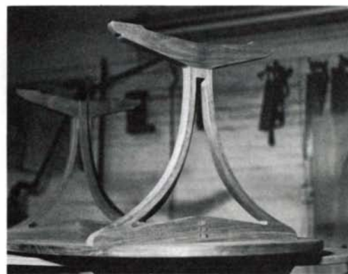
rosewood inlaid with sycamore, and measures 42 in. long and 33 in. high. Right, a typical laminated table understructure. The curved legs are attached to the feet and top bearing rails with splines instead of mortise-and-tenon joints, with the grain of the spline crossing the line of the joint.
