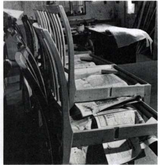
A partially complete set of dining chairs, with dovetail ways cut before assembly in the seat rails and mortises in the back posts. The arms can still be wiggled into place, since the tenon will enter the mortise before the dovetail is tightly home.
