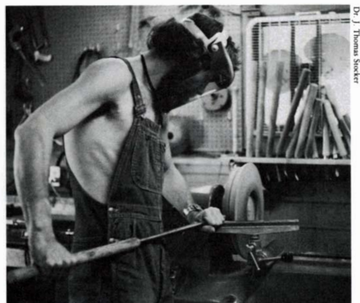
To shape the outside of a bowl, Ellsworth uses a 3 ft. long, \frac{3}{8} in. roundnose tool.
