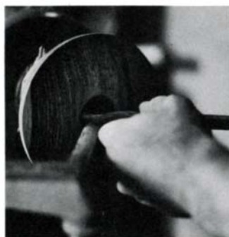
Internal turning begins with a \frac{3}{8} -in. arrowhead-shaped tool.
