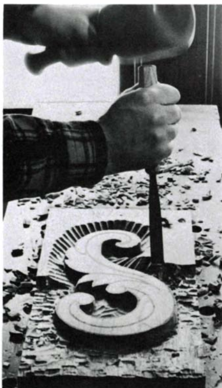
Remove background waste with closely spaced vertical cuts.
