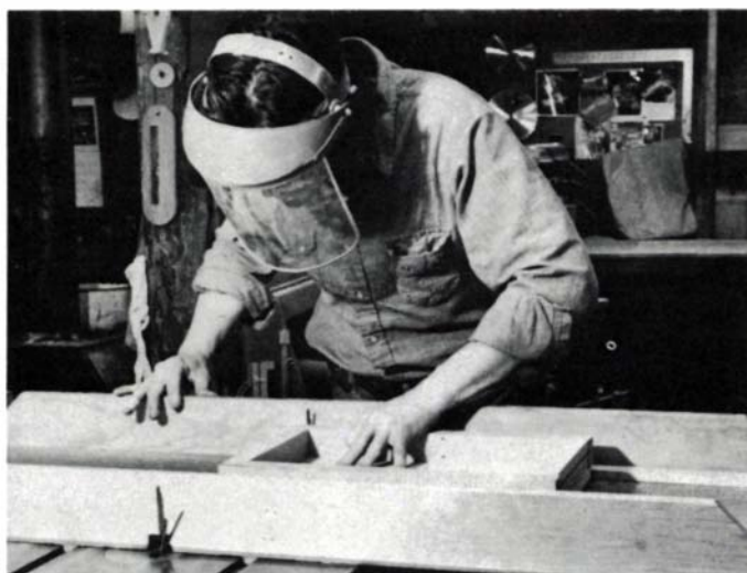
Crosscutting cradle guides trim cuts on stationary housing.
