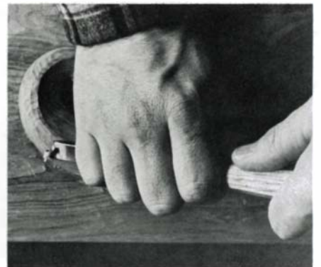
A firmer smooths the outside curves, again with long sweeping cuts.
