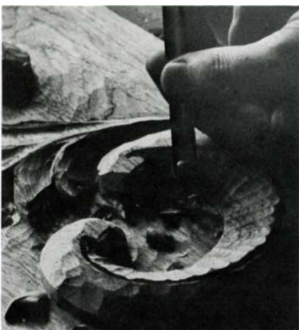
A quick gouge rough-shapes the wood on the inside curves.
