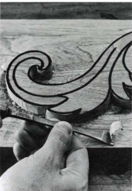
A #5 gouge levels and smooths rough cuts.
