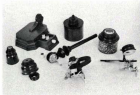
Parts of the Marshall microscope. Specimen stage, right, carries mirror for reflecting light, spring-retained slide mounting and small specimen tweezers. Drawer in base contains several objective lenses.
