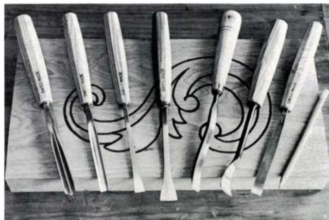
Relief carving tools (from left): V-tool for outlining, three gouges for general shaping, long bent grounder for backgrounds, spoon gouge, and flat or firmer gouge. The blank is butternut, held to the bench by a long screw from underneath.
