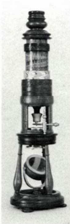
Parts of the Marshall microscope. Specimen stage, right, carries mirror for reflecting light, spring-retained slide mounting and small specimen tweezers. Drawer in base contains several objective lenses.
