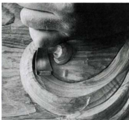
Long sweep cuts leave a smooth finish. A bent gouge or spoon gouge may be best for inside curves. The right hand powers the tool, while the edge of the left hand rests firmly on the work.
