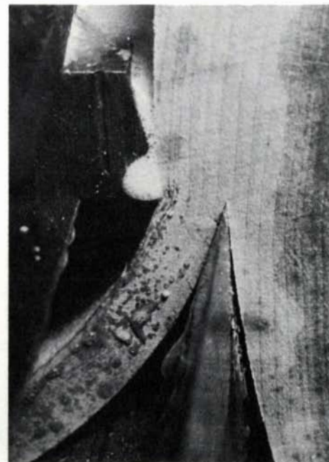
checking. When the nosebar pressure approaches 15% to 20% of the veneer thickness, right, checks are nearly eliminated.
