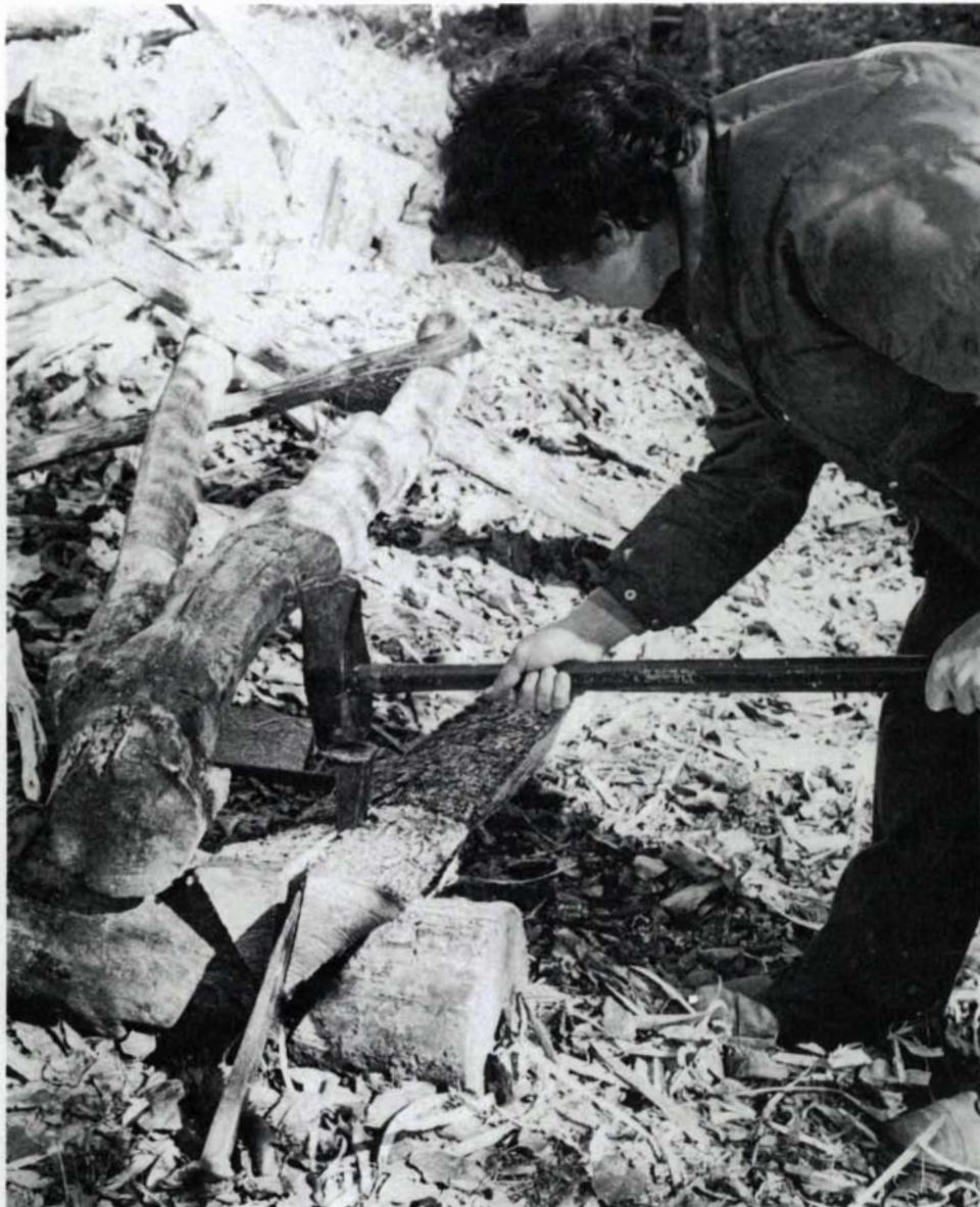
Hewing: With an iron wedge driven into the end of a white oak log (top left), wedges are leap-frogged along the cleft. Two 3-in. gluts and a dogwood cudgel complete the split (bottom left). Then quarters are cleaved into eighths with a pair of wedges and a 10-lb. go-devil (above). Note the splitting break at left, propped up by crossed saplings.
