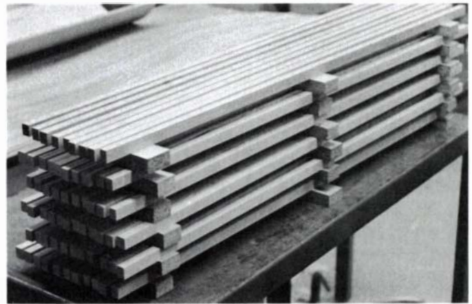
Stickered tambours dry unrestrained; warped ones will be discarded.
