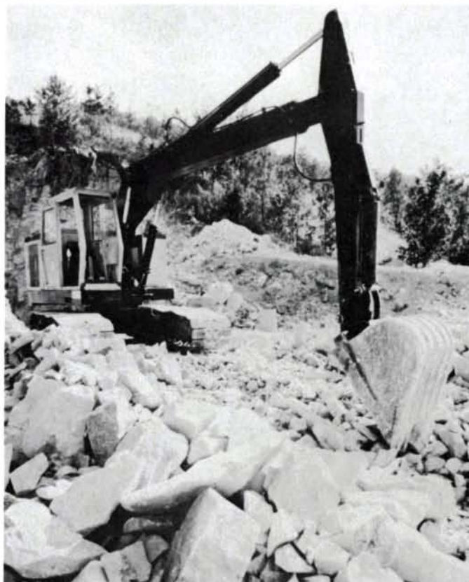
Blocks of novaculite blasted out of a quarry at the Hiram A. Smith Whetstone Co., Hot Springs, Ark. Only about 5% of the novaculite quarried will become finished whetstones.
