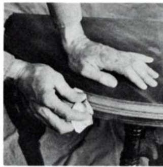
Molded edges can be sanded with a wadded-up piece of used sandpaper. Start with 120 grit, follow with 180 grit, and finish with dry 4/0 steel wool.
