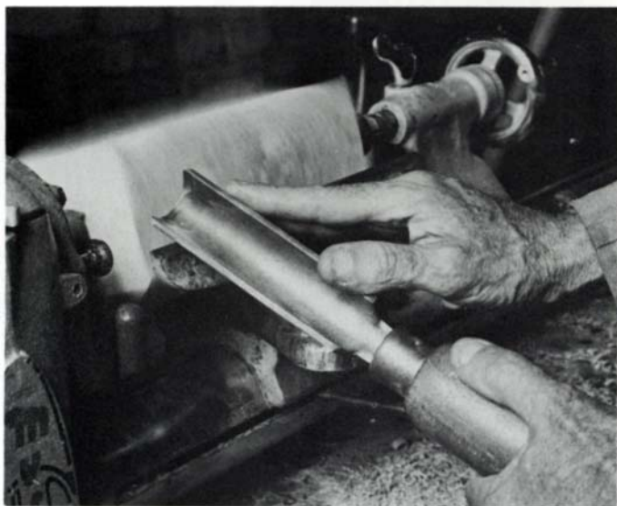
To rough from square to round: Lift the handle until the edge contacts the blur, traverse from left to right and roll the gouge.
