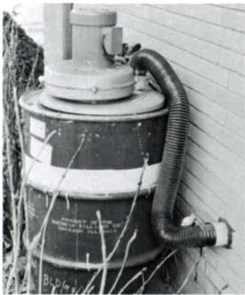
Collector mounted outdoors on 55-gal. drum, left, is connected to machinery inside shop in various ways. Center, semicircular catcher of \frac{1}{4} -in. Masonite and \frac{1}{2} -in. plywood funnels debris from radial arm saw into the pipe about 1 in. above catcher bottom. Blade-guard
