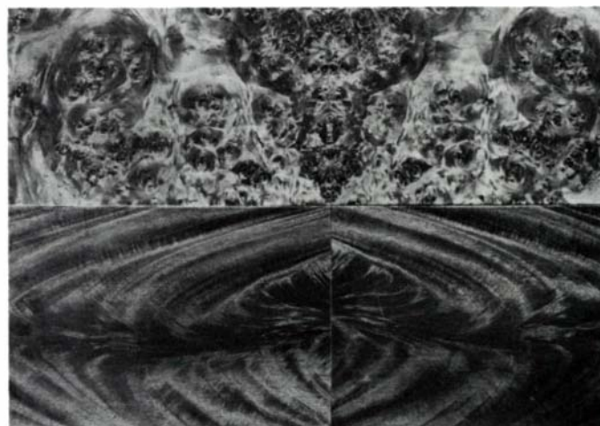
Top, ferrous sulfate brings out contrasting figure in 'palazota' maple, Bottom, mahogany treated with potassium dichromate gives illusion of great depth.
