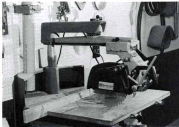
Collector mounted outdoors on 55-gal. drum, left, is connected to machinery inside shop in various ways. Center, semicircular catcher of \frac{1}{4} -in. Masonite and \frac{1}{2} -in. plywood funnels debris from radial arm saw into the pipe about 1 in. above catcher bottom. Blade-guard
