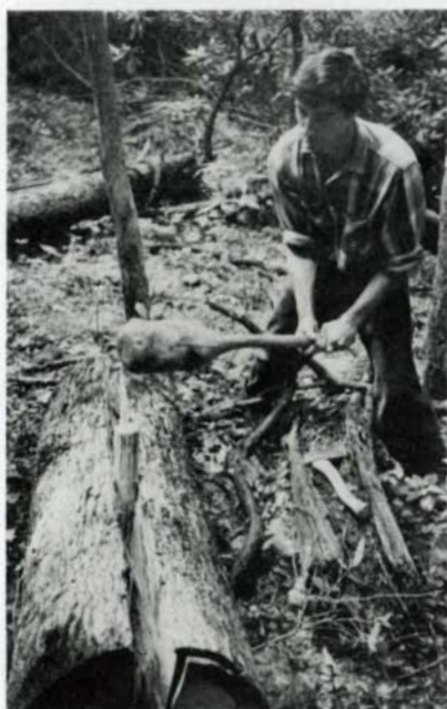
Hewing: With an iron wedge driven into the end of a white oak log (top left), wedges are leap-frogged along the cleft. Two 3-in. gluts and a dogwood cudgel complete the split (bottom left). Then quarters are cleaved into eighths with a pair of wedges and a 10-lb. go-devil (above). Note the splitting break at left, propped up by crossed saplings.
