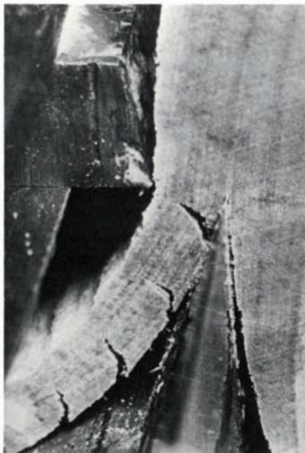
With nosebar retracted, left, veneer checks seriously as it curls over the knife. A little nosebar pressure, center, reduces the amount of
