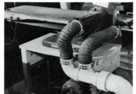
Shaper setup, above, has 45° PVC elbow with sheet-metal sleeve inside. A \frac{3}{8} -in. threaded rod, bent L-shaped and clamped to elbow with plumber's tape, secures hose to table. Sheet metal closes off area behind cutter. Hose unit swings away to change cutters. Wiring for dust-collection system is diagrammed at left.
