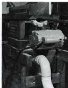
Shaper setup, above, has 45° PVC elbow with sheet-metal sleeve inside. A \frac{3}{8} -in. threaded rod, bent L-shaped and clamped to elbow with plumber's tape, secures hose to table. Sheet metal closes off area behind cutter. Hose unit swings away to change cutters. Wiring for dust-collection system is diagrammed at left.
