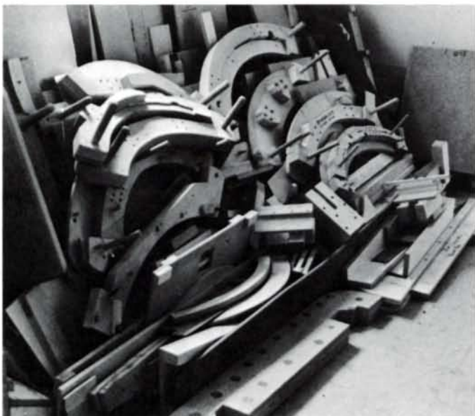
Jigs that made the woody's parts (top) would fill the finished car. Wheel-well apron (center) is shaped from square stock. Rebuilt Model A has chassis by Ford, body by Kariher.
