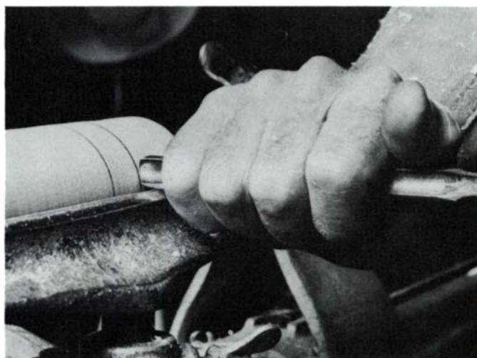
To start a cove, hold the gouge firmly and push its point in slowly.
