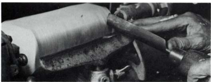
End of first cut; small chips are ‘corners’ wood. Now go back again, slowly rolling the gouge, handle always lower than cutting edge.
