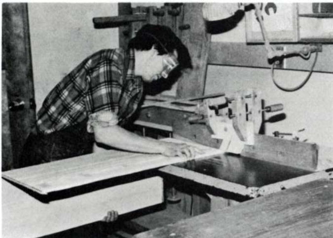
After tambour is glued up, tongue shoulders are sawn (left), then waste is routed from front and back (above). Canvas flap is for attaching handles.
