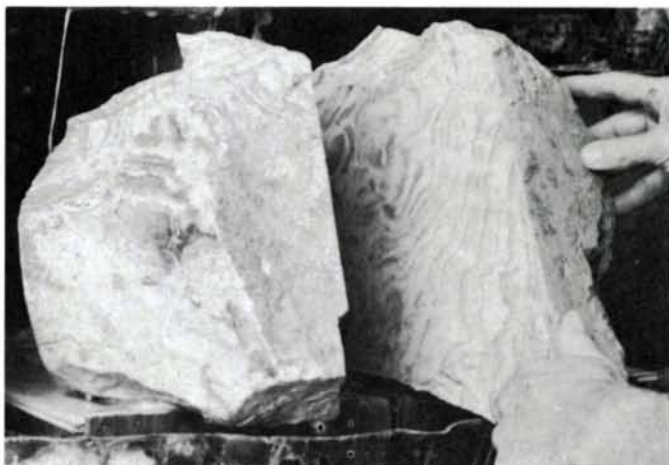
Raw Washita stone has been halved on diamond-edged steel wheel.
