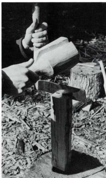
A froe is driven into the wood with a mallet, then worked along the long fibers by leverage. Long pieces of wood may be supported in a brake (far left); short chunks can rest on a stump (left). The diagram shows the cleaving sequence for basket splints. Heartwood is usually discarded; squared-off sapwood is split into halves, quarters, eighths and sometimes sixteenths. A froe makes the first cuts; finer splits are made with a knife.
