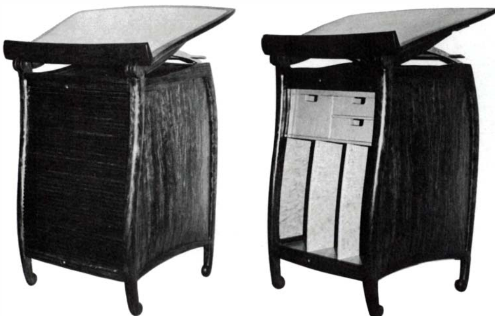
Left, author's writing cabinet, bubinga and figured maple. Above, detail of Richard Tannen's tall maple cabinet; fixed slats are filler strip.
