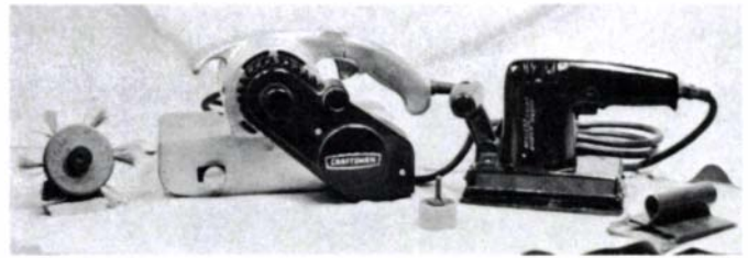
Sanding equipment includes (left to right) a Merit Sand-O-Flex, a belt sander, a drum sander, an orbital sander and a sanding block.
