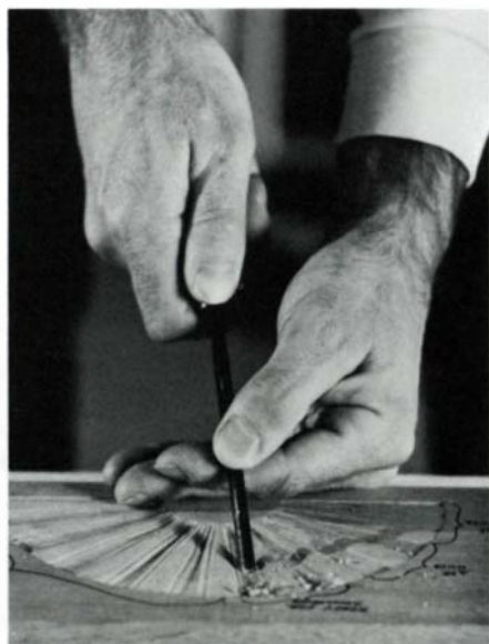
Author uses 6-mm #7 gouge to hollow concave portion of concave-convex fan. Simple convex fan enhances author's reproduction of Queen Anne lowboy, circa 1750.
