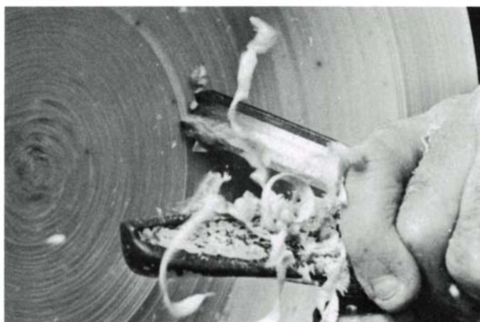
Gouge nears completion of cut, top, coming down toward center line before horizontal push to center itself. Close-up shows full left half of blade cutting, but tip of wing is clear.
