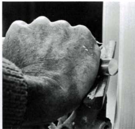
Starting a cut: Gouge just contacts wood, with left-hand corner of blade clear to avoid a dig-in. The bevel, center, as yet has no support
