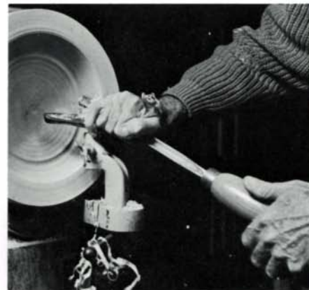
from the wood, so the tool must be held very firmly and pushed straight in to start its arc toward the center.
