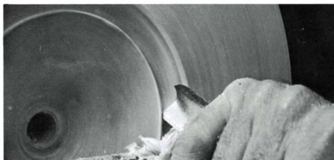
Turner fails to shuffle to right, and left corner of gouge enters wood, causing a jamming ridge.
