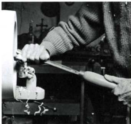
Starting a cut: Gouge just contacts wood, with left-hand corner of blade clear to avoid a dig-in. The bevel, center, as yet has no support
