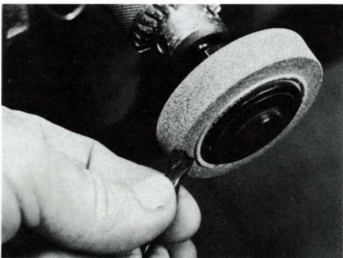
Ordinary drill bit is reground, on slightly rounded edge of small stone, to leave sharp center spur and clean-cutting edges.
