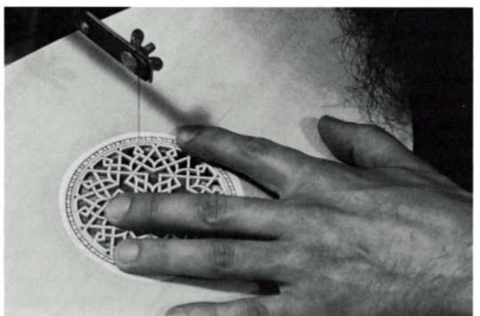
In German method, which author prefers, paper pattern is glued to front of belly and cut with a fretsaw.
