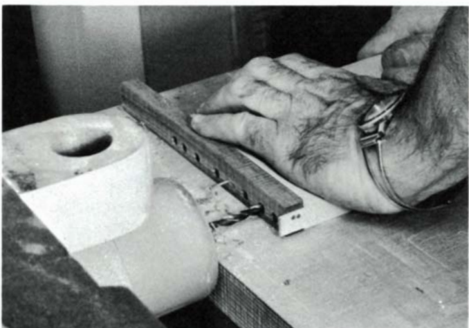
With heel tight against back edge of board, a single nail holds doweling jig in place for drilling on horizontal mortiser.
