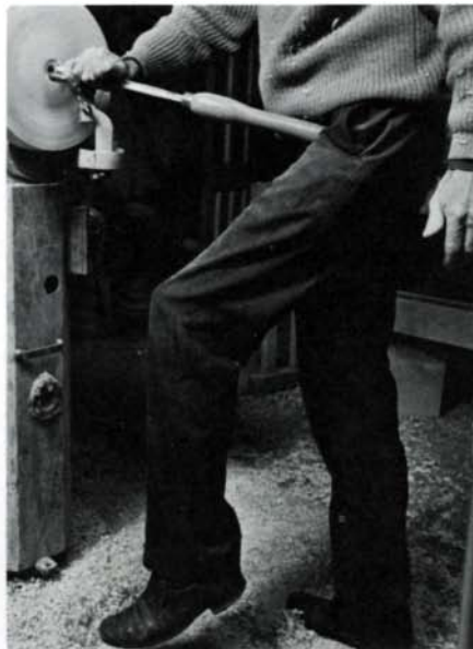
Cut taken without use of left hand demonstrates proper body control. With right hand as stationary pivot, power comes from thigh as left foot lifts entirely off floor. Photo at right shows full-power cut:
