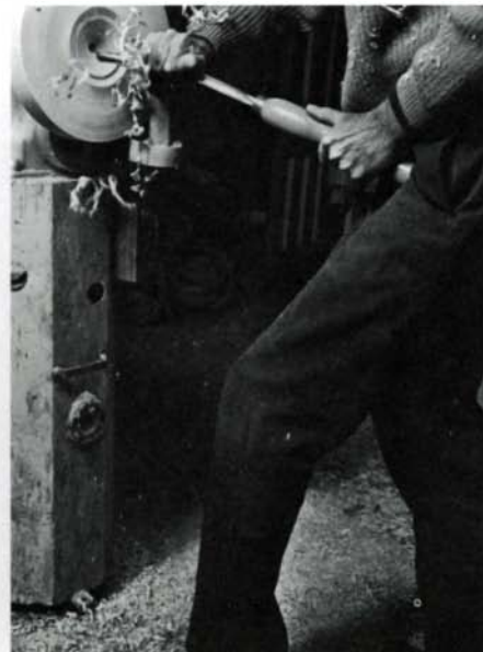
Left leg provides lift, while left hand governs forward roll of tool. Palm of right hand does not move, but turner swings to right to keep blade cutting without jamming.
