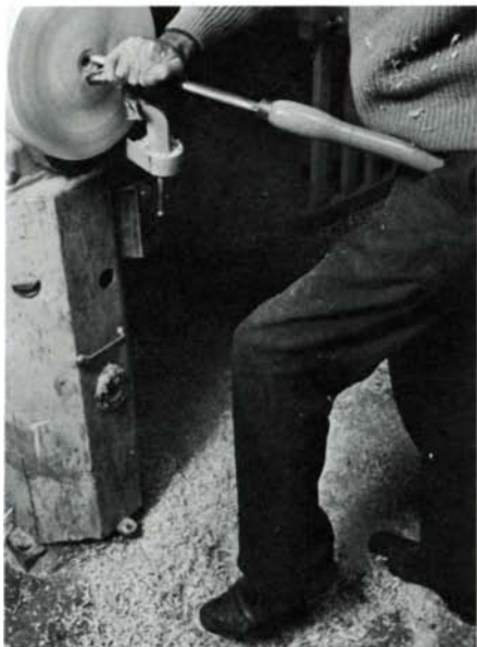
Cut taken without use of left hand demonstrates proper body control. With right hand as stationary pivot, power comes from thigh as left foot lifts entirely off floor. Photo at right shows full-power cut:
