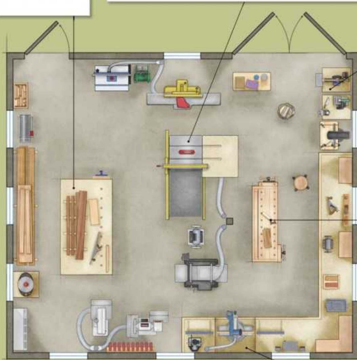
Versatile (and very big). The 50-in. by 90-in. MDF-topped assembly table is well positioned for stacking lumber and workpieces while milling. Outfitted with a vise and dog holes, it also serves as an auxiliary planing bench.
