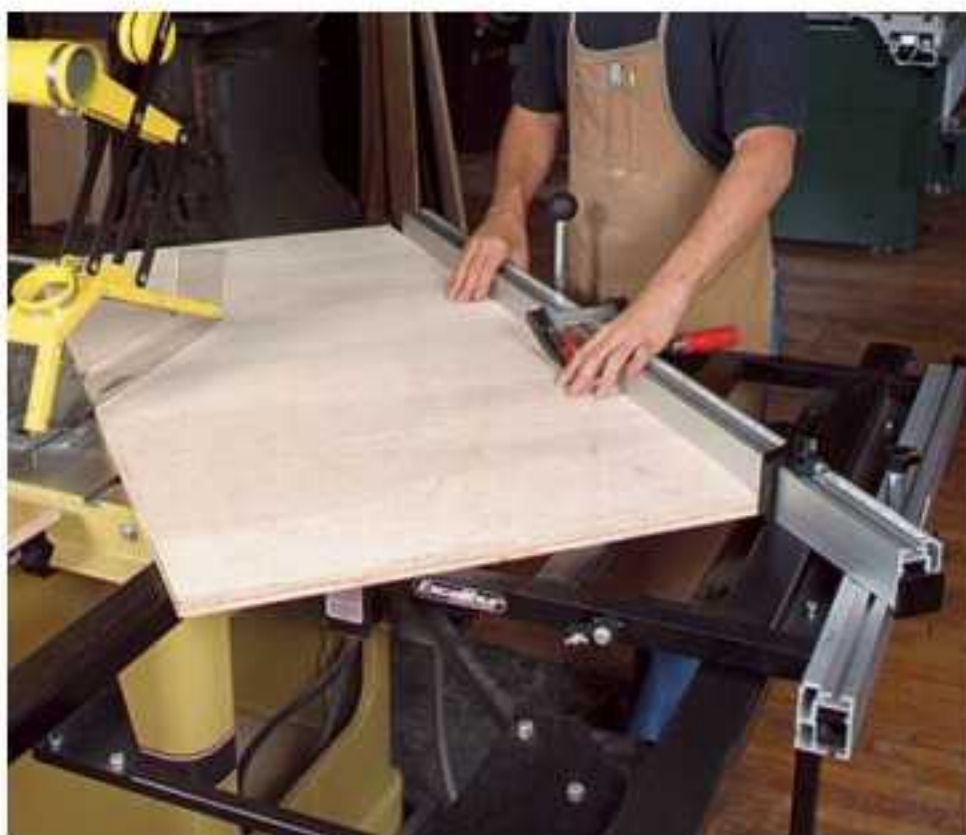
Suit it to your work. Some aftermarket sliding tables are larger than others. If you mostly work with sheet goods, consider a large table for more workpiece support.
