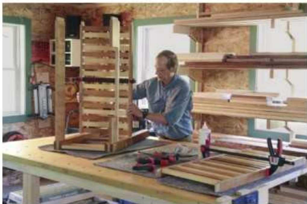
Versatile (and very big). The 50-in. by 90-in. MDF-topped assembly table is well positioned for stacking lumber and workpieces while milling. Outfitted with a vise and dog holes, it also serves as an auxiliary planing bench.
