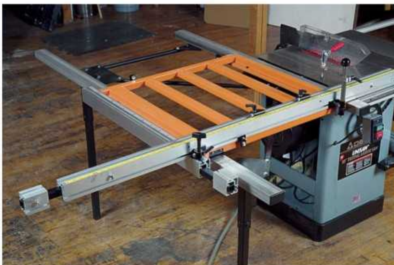
Suit it to your work. Some aftermarket sliding tables are larger than others. If you mostly work with sheet goods, consider a large table for more workpiece support.
