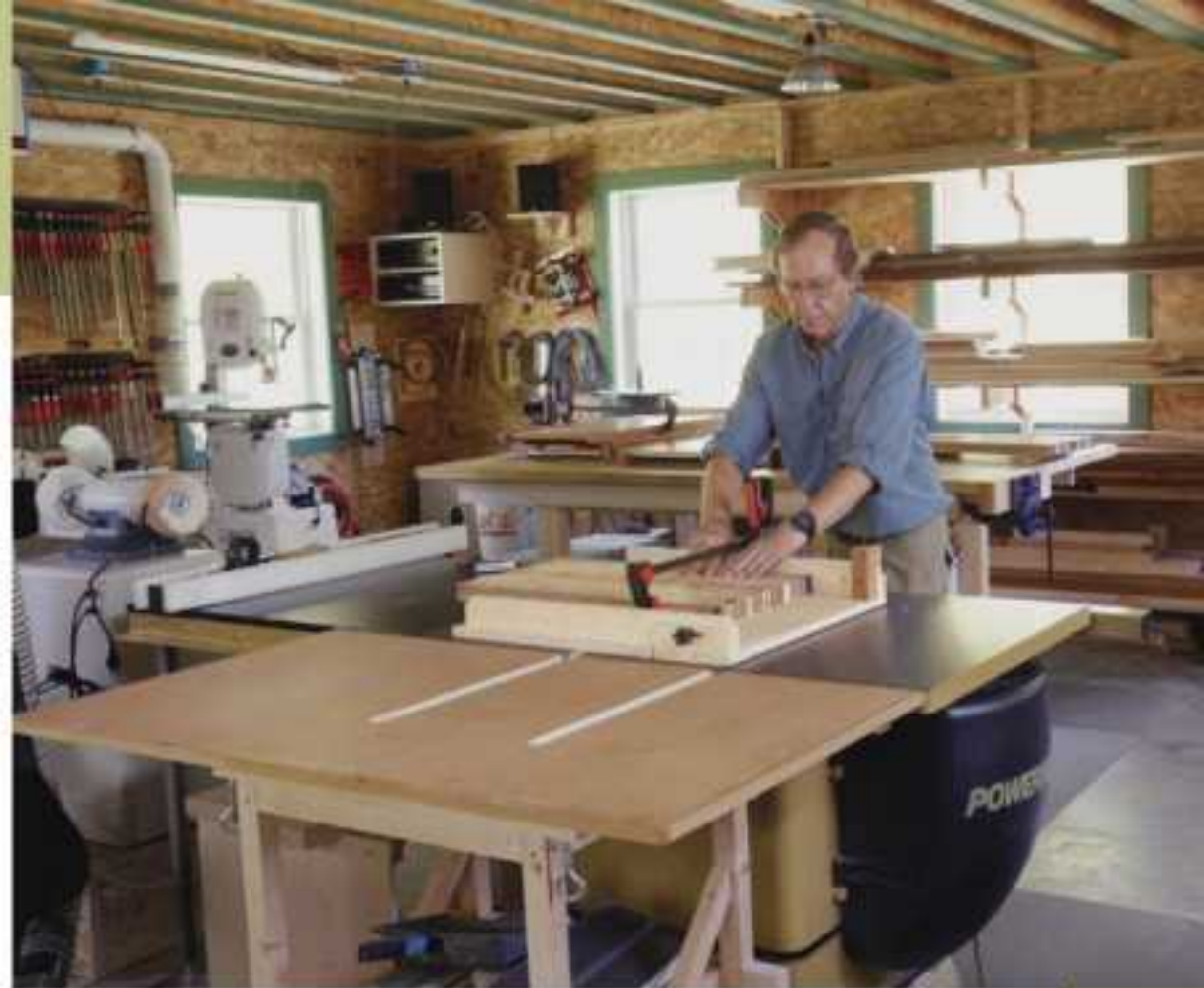
Saw at the center. Located right at the heart of the shop, Bauer's tablesaw is equally convenient to his milling machines, workbench, and assembly table.
