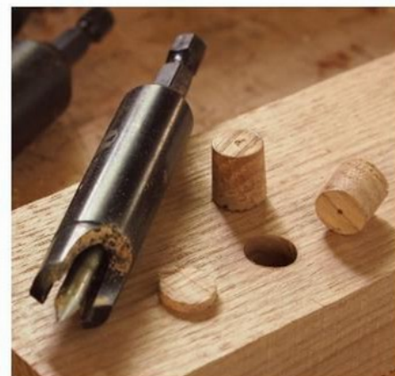
Plug away freehand. The self-centering bit means accurate results with simply a handheld drill (left). The bit is tapered just a little, so plugs will fit snugly.
