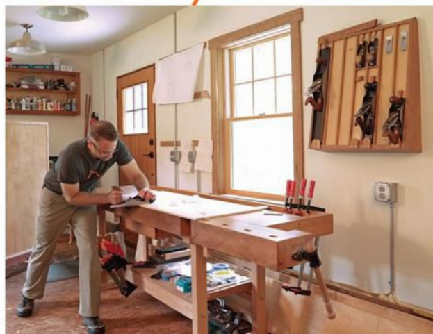
Best spot for the bench. Korsak located his workbench along the south wall, where the natural light is best. He made a wall-mounted till to keep his handplanes within easy reach.
