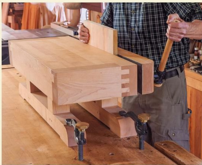
Same features as the main bench. By adding a vise to the auxiliary bench, Becksvoort keeps his usual methods intact while working at the optimal height.
