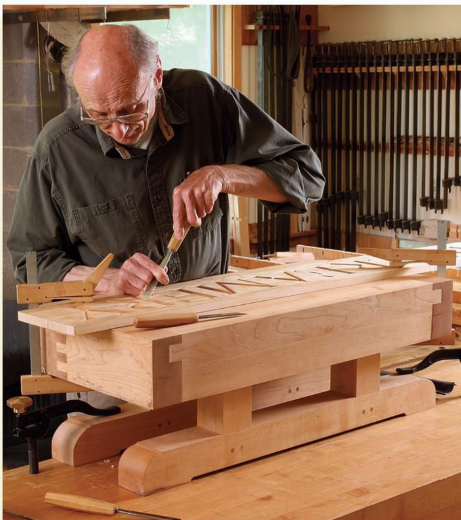
Bring the work up. With the smaller bench clamped to the main bench, Becksvoort can work at a level that will be comfortable for extended periods of time and allow him to use his body position productively.
