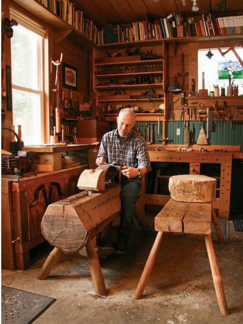
Fine shop furniture. Fisher's canted-leg low bench (below) serves him for chopping, carving, and for reaching his library of woodworking books. His bowl horse (left), made from a stout log, pinions a workpiece from front and back.
