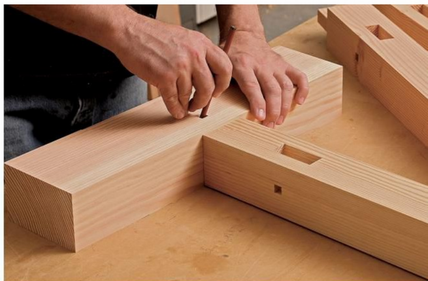
Mark and move. After assembling the post-to-foot joint and marking the location of the drawbore hole, Cullum chops the mating mortise \frac{1}{16} in. closer to the tenon shoulder.
