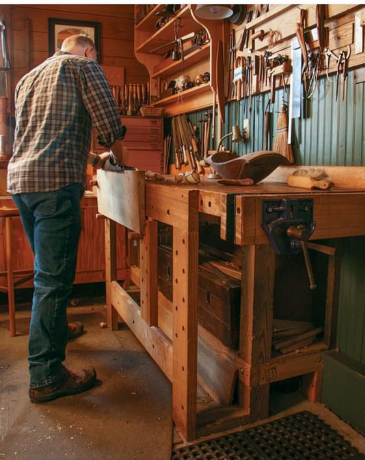
Rudimentary and rock-solid. Fisher's built-in bench, made years ago from construction lumber and exterior plywood, was upgraded for handwork with the addition of a frame with a sliding deadman.
