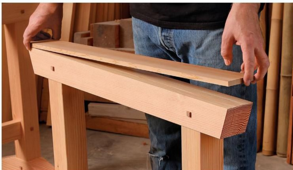
Protect the top. A couple of strips of double-sided tape hold a sacrificial cap piece in place on the beam. The softwood cap protects both the beam and the workpiece from damage.
