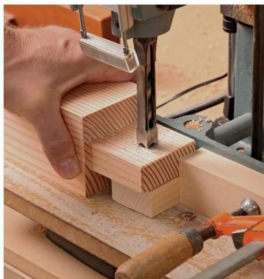
Mark and move. After assembling the post-to-foot joint and marking the location of the drawbore hole, Cullum chops the mating mortise \frac{1}{16} in. closer to the tenon shoulder.
