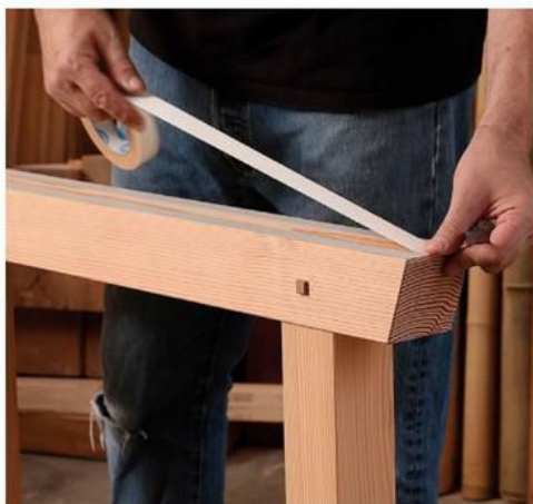
Protect the top. A couple of strips of double-sided tape hold a sacrificial cap piece in place on the beam. The softwood cap protects both the beam and the workpiece from damage.
