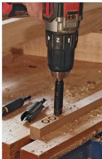
Plug away freehand. The self-centering bit means accurate results with simply a handheld drill (left). The bit is tapered just a little, so plugs will fit snugly.
