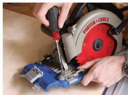
Screw, set, saw. Securing the sled to the saw is simply a matter of tightening some set screws. Once in place, the sled rides along the track for a non-slip cut.
