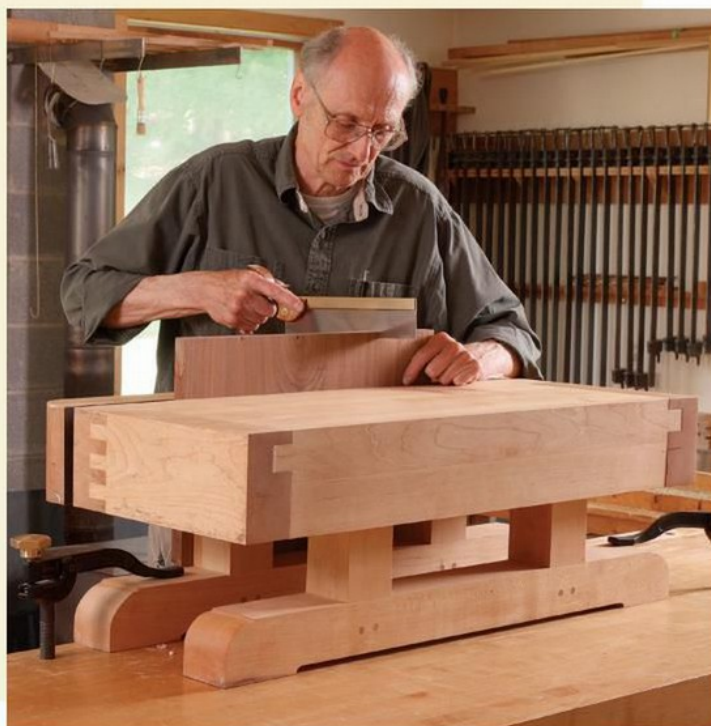
Bring the work up. With the smaller bench clamped to the main bench, Becksvoort can work at a level that will be comfortable for extended periods of time and allow him to use his body position productively.
