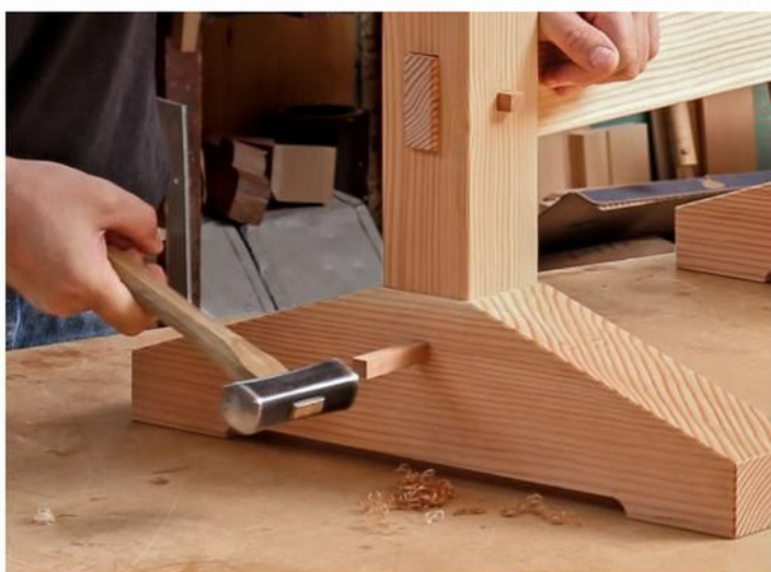
Assemble in stages. Cullum first drives the pins connecting the stretcher to the posts, then fits the posts into the beam (right).
