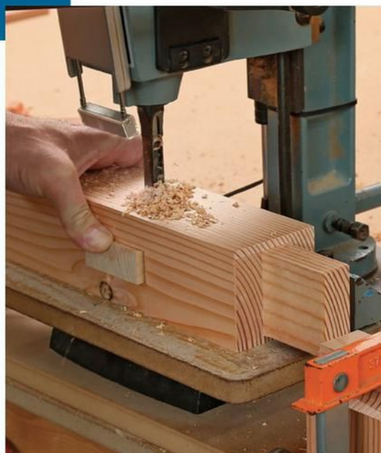
Make way for the pins. With a sacrificial spacer inserted in the through-mortise, Cullum chops a hole for the drawbore pin.
