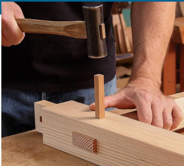
Assemble in stages. Cullum first drives the pins connecting the stretcher to the posts, then fits the posts into the beam (right).
