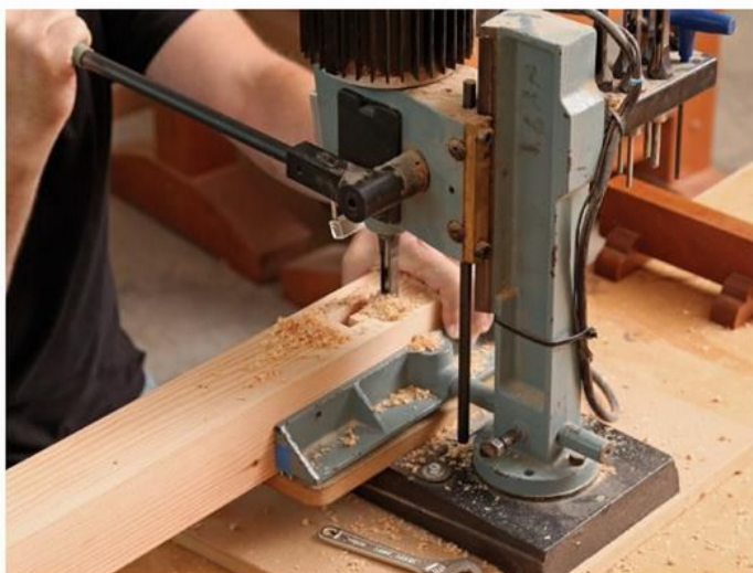
Both sides now. Cullum cuts the through-mortises for the stretcher tenons at his mortiser, chopping from both faces to the middle.
