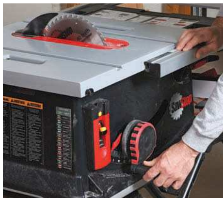
Super-fast height adjustment. One turn of the handle brings the blade to full height, but there is still enough finesse in the mechanism to fine-tune the height for precise work.
