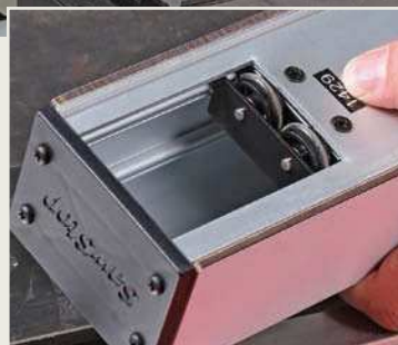
Slick fence. Sturdy and deflection-free, the SawStop's fence locks down tight (above). It also glides over the table as if it were floating on air, thanks to a pair of small wheels at the end (left).
