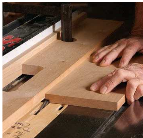
Rabbets, too. To cut rabbets, clamp a sacrificial fence to the rip fence and position it over the blade. Set the depth of cut and run the stock against the fence.
