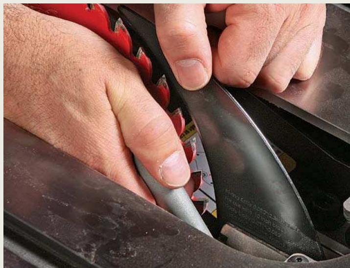
Quick exchange from riving knife to guard. A big, easy-to-reach lever is all you need to free them on the SawStop.
