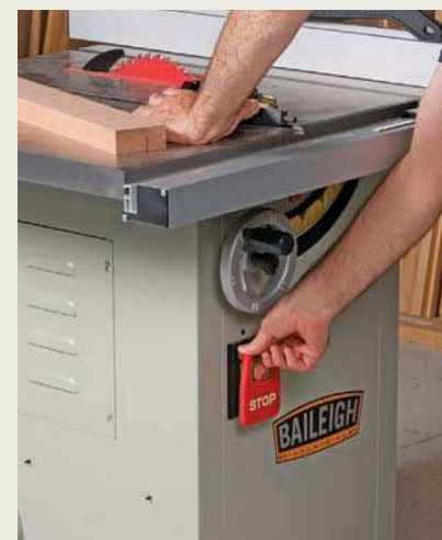
Long reach for the power switch. Located beneath the height adjustment wheel, the switch requires you to lean over too far.
