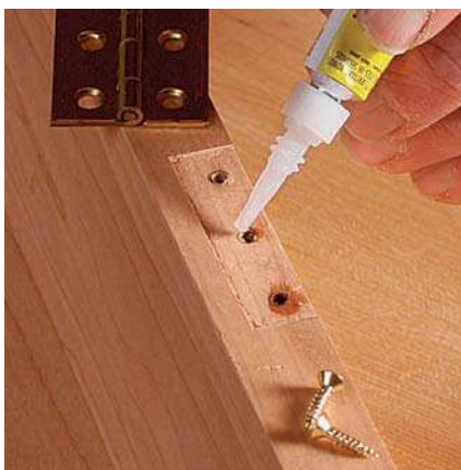
Reinforce screw holes. Neptune uses CA glue in softer woods where he has to insert shallow screws, such as for hinges.
