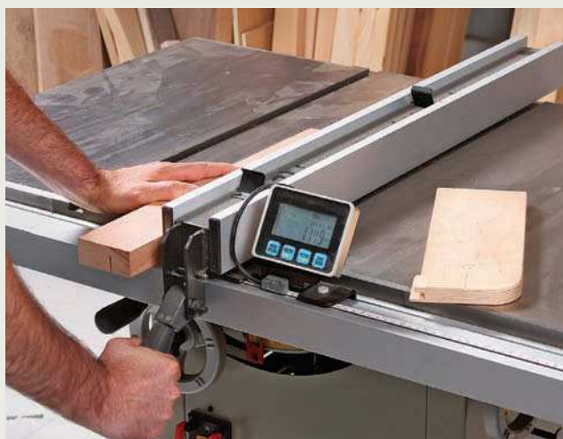
Digital fence readout. The distance from the blade to the fence is displayed to a thousandth of an inch, and it's accurate.
