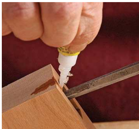
Open wide. Use a flat screwdriver or other narrow blade to pry open the crack so that glue flows down into it.
