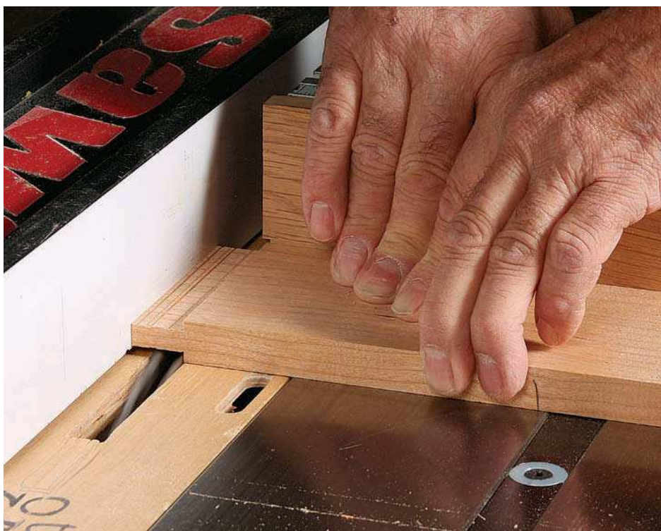
Tenons made simple. Cutting tenons with a dado set is fast and easy. Use a miter gauge to hold the workpiece and the rip fence to set the tenon's length. A few passes on each cheek will produce tenons ready to be fitted by hand with a shoulder plane.
