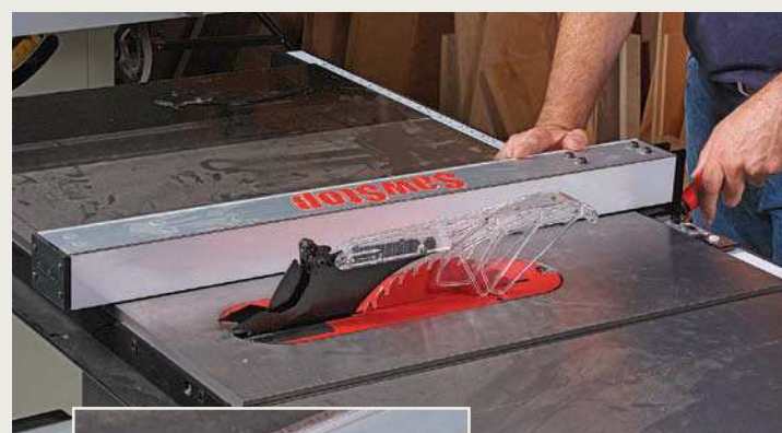
Slick fence. Sturdy and deflection-free, the SawStop's fence locks down tight (above). It also glides over the table as if it were floating on air, thanks to a pair of small wheels at the end (left).
