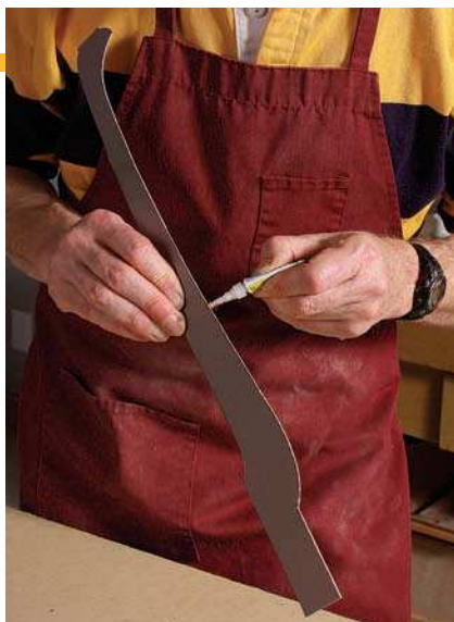
Harden edges of templates. Will Neptune uses mat board to make templates for chair back splats, cabriole legs, etc. He lets thin CA glue soak into the edges and after it dries "as hard as laminate," he can refine the profile by filing or sanding.
