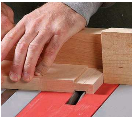
Plenty of power for a dado set. With a \frac{3}{4} -in.-wide dado stack on the arbor, the saw easily cut dadoes and tenons.
