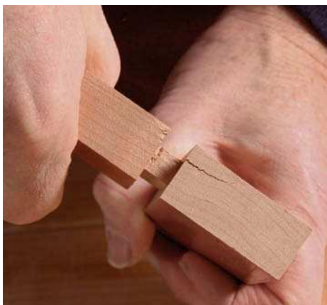
Low viscosity is ideal for hairline cracks. Forcing a too-tight tenon into a mortise cracked the wood.
