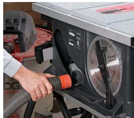
Great dust collection. With a shop vacuum hooked up and the blade guard in place, the saw collected just about all of the dust and chips created.
