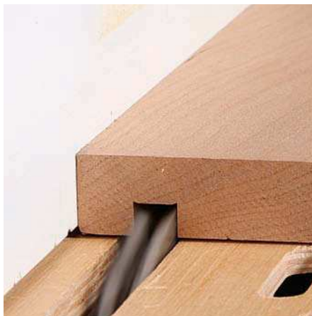
Easy grooves and dados. To cut grooves and dados, stack the blades and set the depth of cut.
