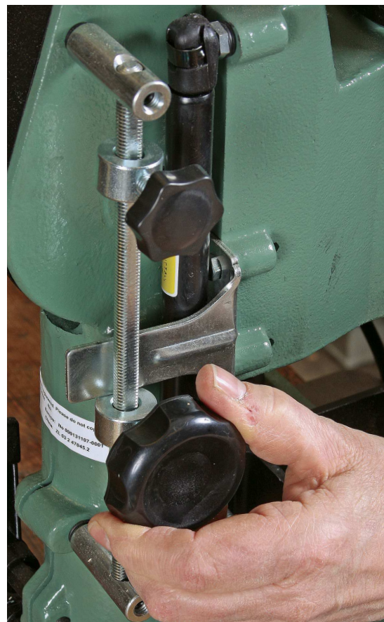
Easy stop. A ratchet handle tightens the Powermatic's stop against the dovetailed ways. It was easy to adjust and tighten.
