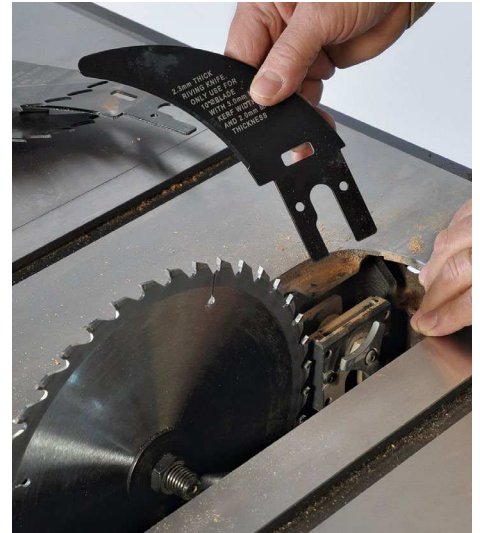
Quick-change riving knife. With the twist of a star knob, you can change from the blade guard to the riving knife in no time at all.
