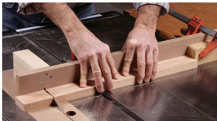
Set the stop. The long MDF auxiliary fence lets you set up a stop at the far end for cutting a series of workpieces to the same length.
