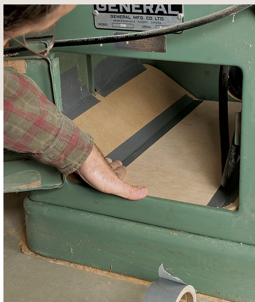
Add intake. Christiana had a plywood box covering the motor opening. So he just routed three slots, positioned to wash cool air over the motor.
