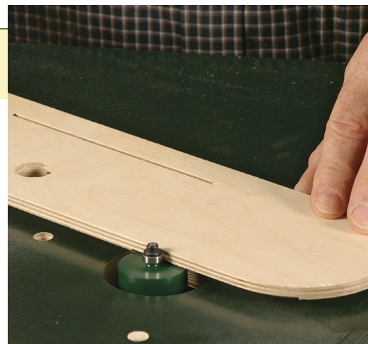
Cut to the line. Take \frac{1}{16} -in. passes with a rabbeting bit, and check the insert in the throat after each pass. If you take off too much, just use tape to raise it up.
