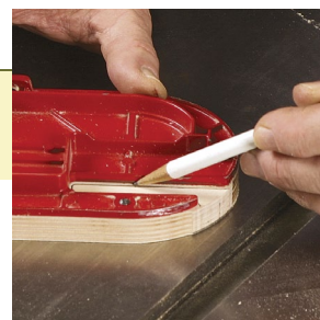
Two openings to cut. Hold down the blank with a push stick (left), staying away from where the blade will come through. Raise the blade slowly. Afterward, mark the opening for the blade-guard assembly (above) and cut it with a bandsaw or jigsaw.
