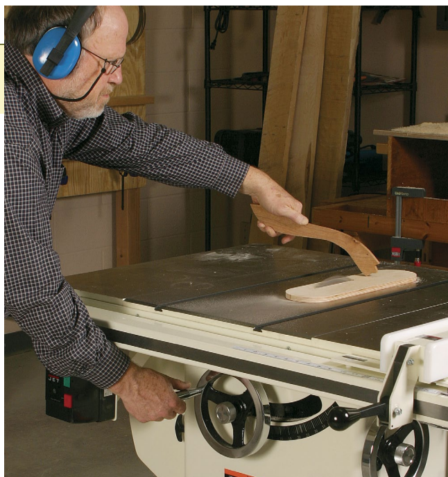
Two openings to cut. Hold down the blank with a push stick (left), staying away from where the blade will come through. Raise the blade slowly. Afterward, mark the opening for the blade-guard assembly (above) and cut it with a bandsaw or jigsaw.
