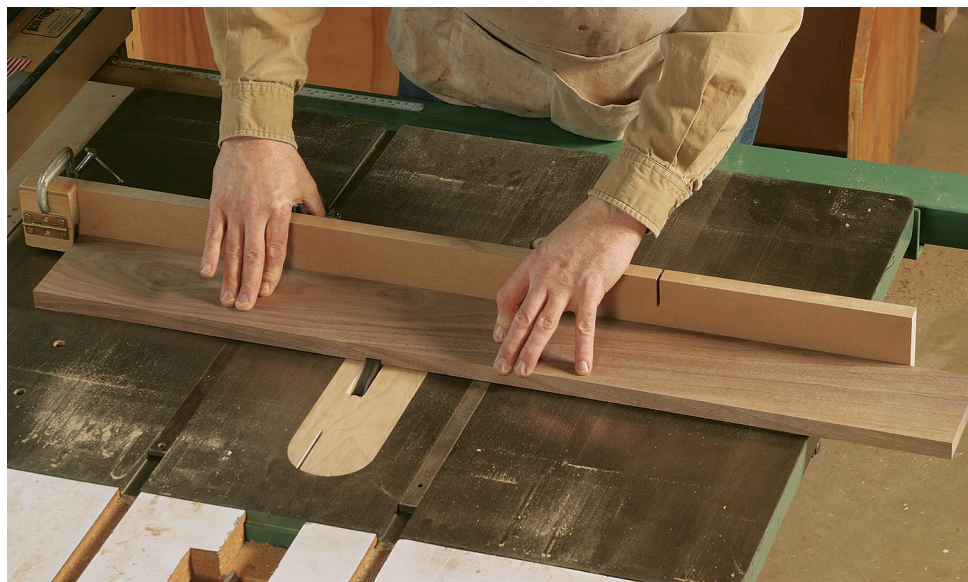
Cut accurate dados. The twin-gauge setup works well for making cuts across the middle of a long workpiece. Used miter gauges are inexpensive and easy to find at flea markets or online.
