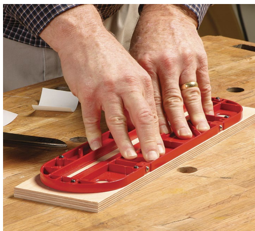
Throat plate becomes template. Attach the throat plate to the blank with double-sided tape.
