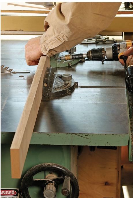
Two gauges run side by side. One sits in each slot; together they support a long fence.
