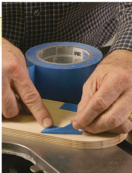
Easy fix for low spots. The plate is supported by a lip or tabs in the saw's throat opening. Apply tape to the low spots to raise the insert flush with the saw table.
