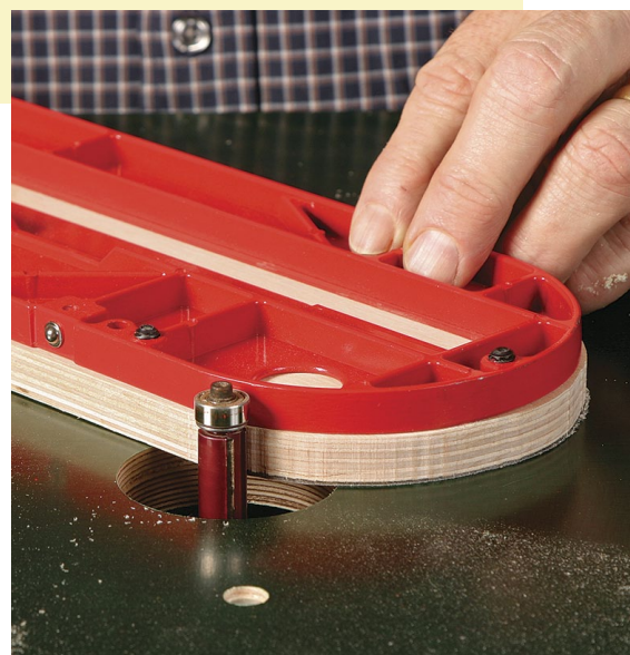
Trim the blank. Rout the insert flush to the throat plate with a bottom-bearing, flush-trimming bit.
