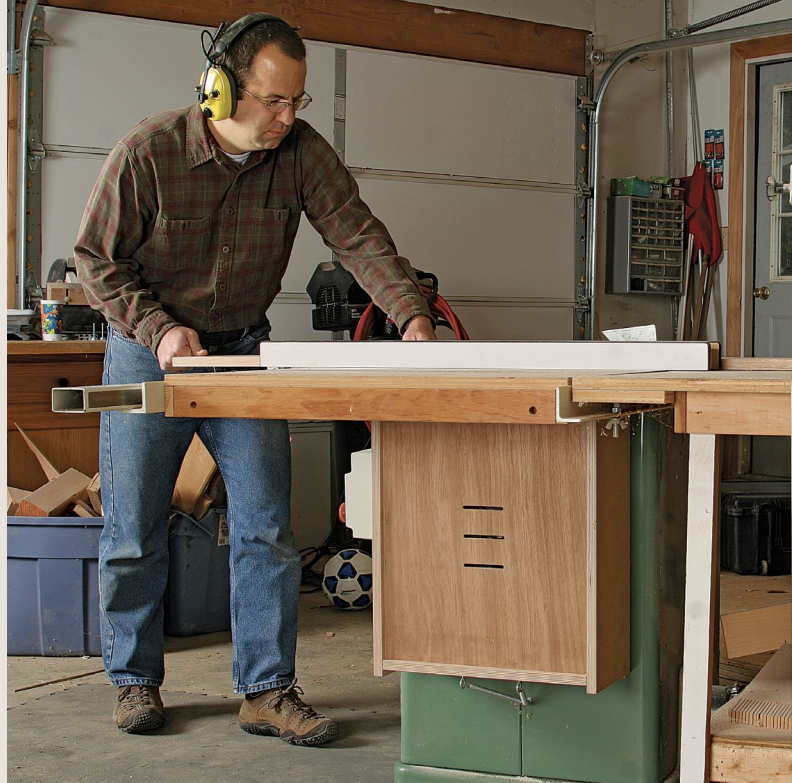
Add intake. Christiana had a plywood box covering the motor opening. So he just routed three slots, positioned to wash cool air over the motor.
