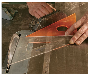
Setting up an angled cut. Use a pair of drafting triangles to set the gauge for a 45° cut. Also be sure the triangle is against the body of the blade and not a tooth, and set the gauge so the leading end of its fence points toward the blade.
