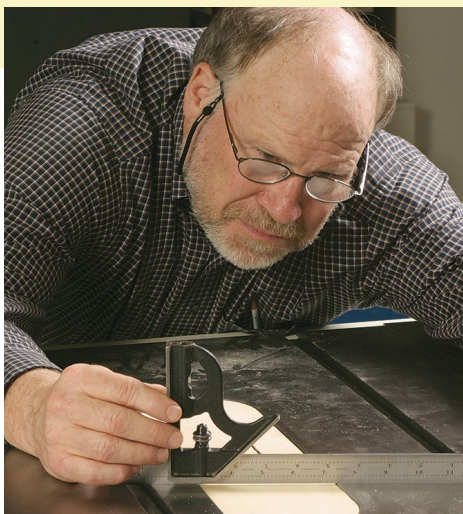
Check for level. The insert should be flush with the saw table. Use a steel ruler to check for high and low spots.
