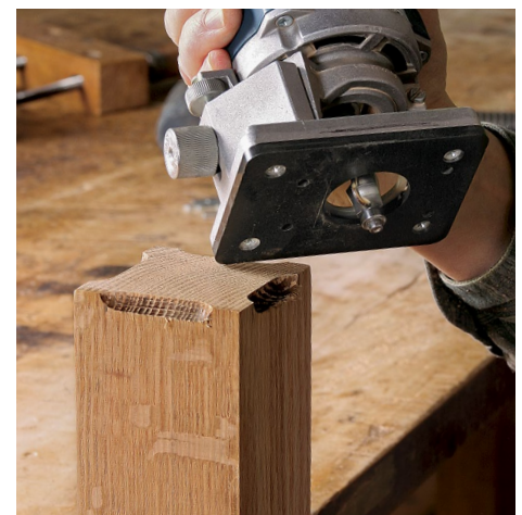
Coves lighten the feet. With the leg post in a vise, using a handheld laminate trimmer (with a 1/4-in. bearing-guided cove bit), move in at one pencil mark and out at the other.
