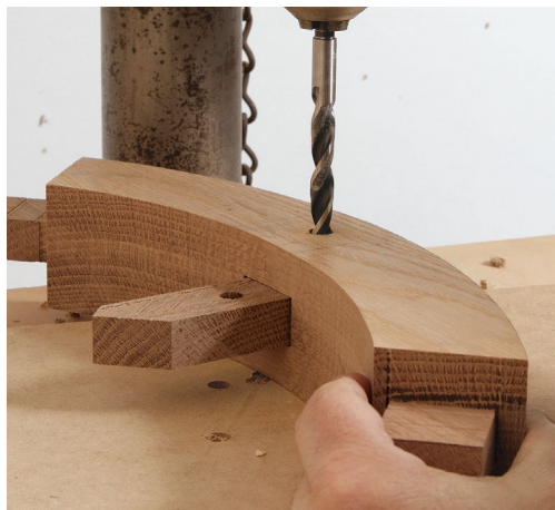
Drill through the mortised parts. Insert a scrap into the mortise to prevent blowout inside.
