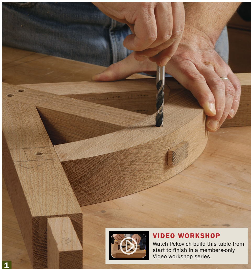
Drill through the mortised parts. Insert a scrap into the mortise to prevent blowout inside.
