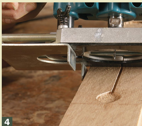
2 Remove most of the recess. Rout close to the inlay border, leaving a bit of waste to clean up by hand.
