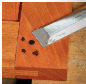
Paring pegs. A chisel is more precise than a handplane and is neater than a sander when leveling a pin.
