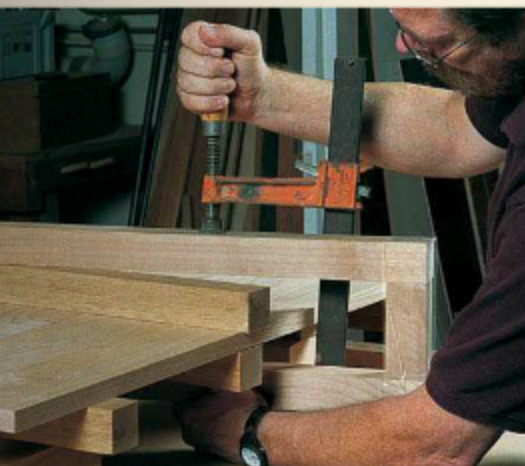
Tape and scrap make simple and effective deep-reach clamps. Tape a spacer between two stout scrap boards and slide the assembly over the cauls. Pressure applied near the edge is transferred to the middle of the panel.
