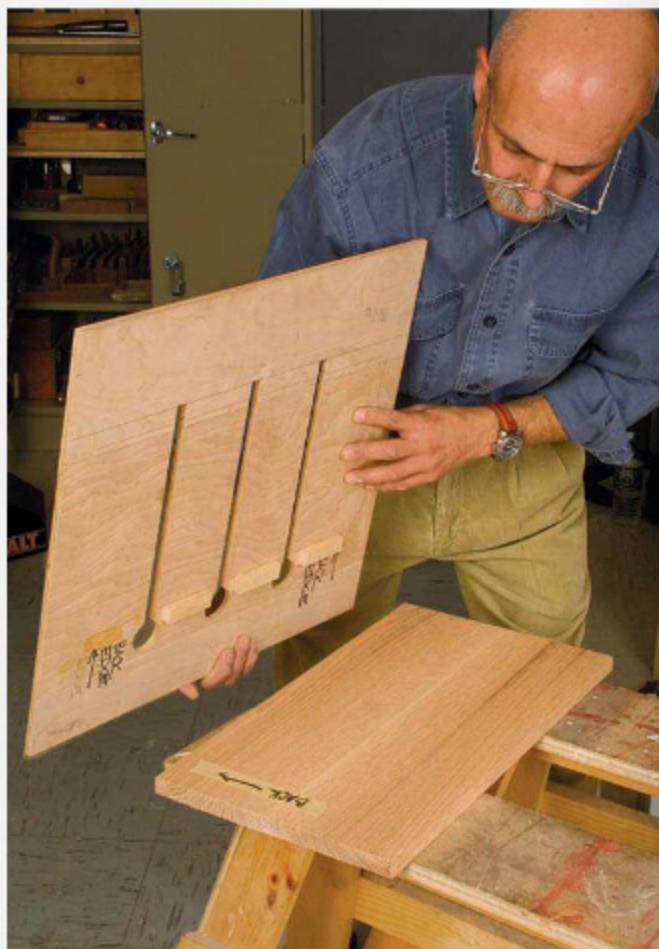
Router template spaces partitions evenly. Because the stopped dadoes for the partitions must be cut precisely and in identical positions on both the upper shelf and the top, it is best to use a plywood template to guide the router.
