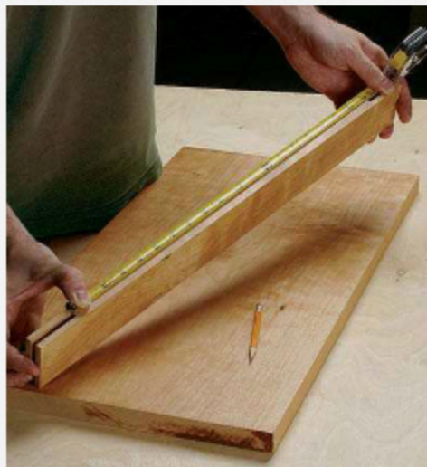
Measure and crosscut. To determine the panel length, Teague measures the distance between the stile mortises (above). Don't try to cut a wide panel using a miter gauge. A shopmade crosscut sled makes the operation easier and safer (right).
