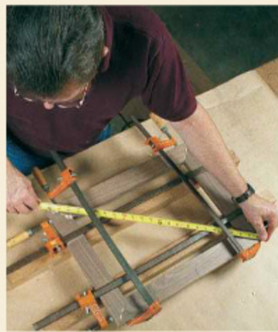
Use two biscuits. A pair of biscuits provides ample gluing surface and keeps the pieces aligned. Once clamps go on, measure the diagonals to make sure everything is square.
