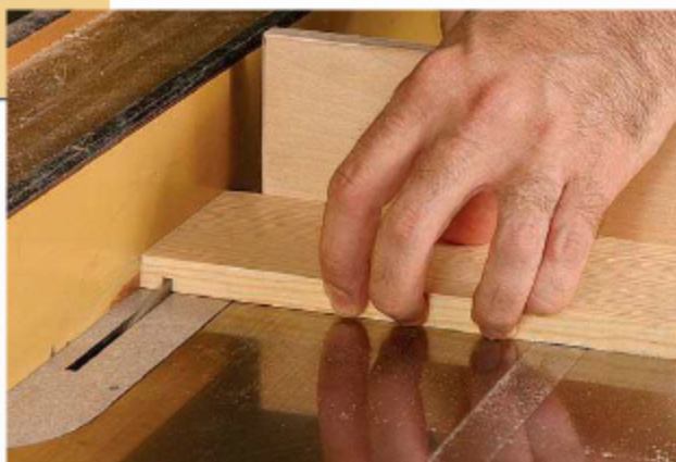
Cut dados in the drawer sides. The positions of the dados on the drawer sides are determined by the thickness of the front and rear drawer pieces.
