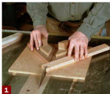
1 The first cut is made on the left-hand side of the jig. If the work slips, it will do so away from the blade.
