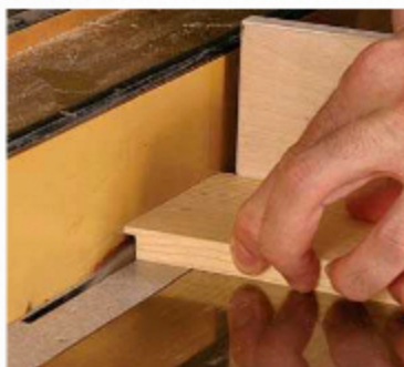
Rabbet the front and rear pieces in two steps. Using a commercial tenon jig to support the workpiece (above), make a vertical cut on the ends of each drawer box front and back. With the piece flat on the table (left), make the second cut, leaving a tongue that will connect with the side pieces.
