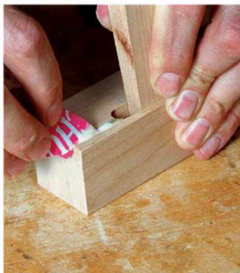
Get glue deep into the crack for a good repair. A piece from a snack-food package or candy wrapper can be used to force glue into a crack.
