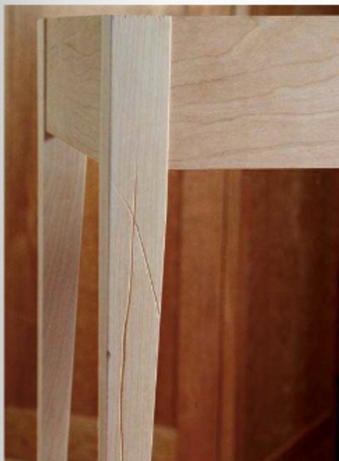
Don't give up on a piece, even if the damage seems severe. Shopmade veneer can be used to conceal cosmetic damage.
