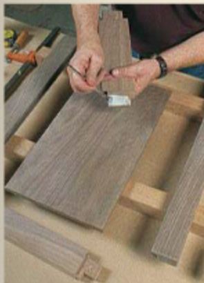
A little glue goes a long way. To keep squeeze-out to a minimum, apply glue deep into the mortise and on the end of the tenon only.
