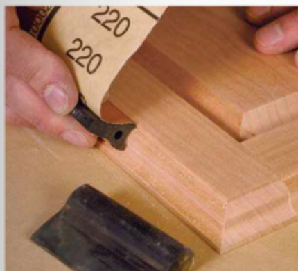
Rubber profiles. Using a rubber pad that fits the molding helps keep the edges of the profile sharp.
