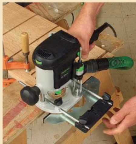
After cutting the stopped dados for the partitions, add an adjustable fence to the router and cut the stopped dados at both ends of the top to receive the sides.
