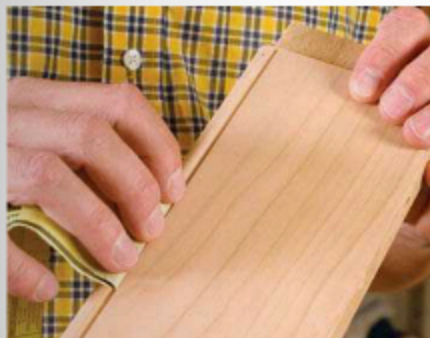
Sanding curves by hand. Contour the paper to fit curves in the wood.
