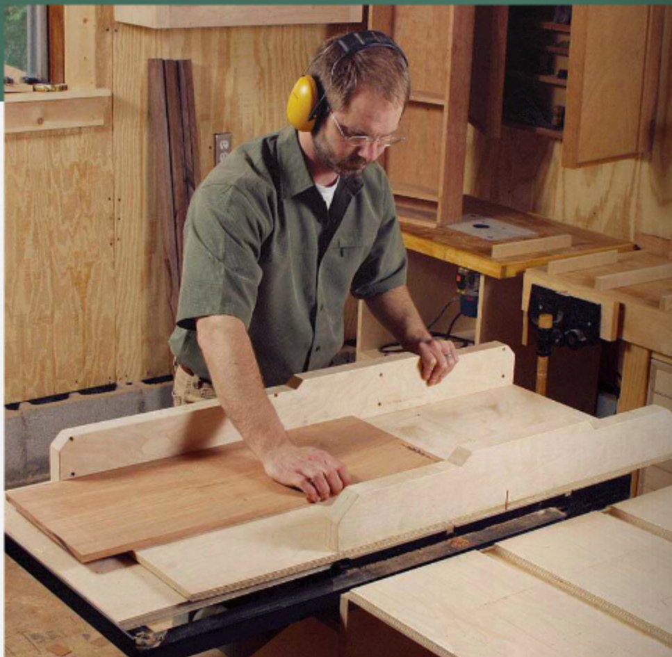
Measure and crosscut. To determine the panel length, Teague measures the distance between the stile mortises (above). Don't try to cut a wide panel using a miter gauge. A shopmade crosscut sled makes the operation easier and safer (right).
