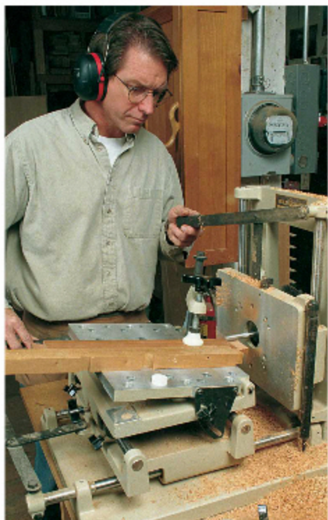
Routing machines for production work. Guided by templates or set by hand, the horizontal routing machine takes a little work to set up but can cut countless tenons in no time at all. The table also tilts to make easy work of angled tenons.
