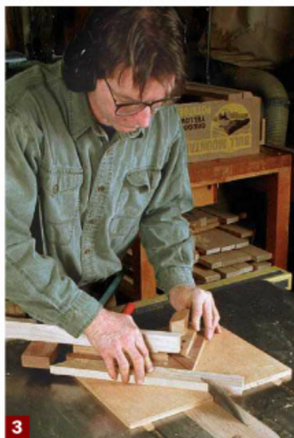
3 Make the second cut on the right-hand side of the jig. With the stop block in place, you are assured of consistent cuts.
