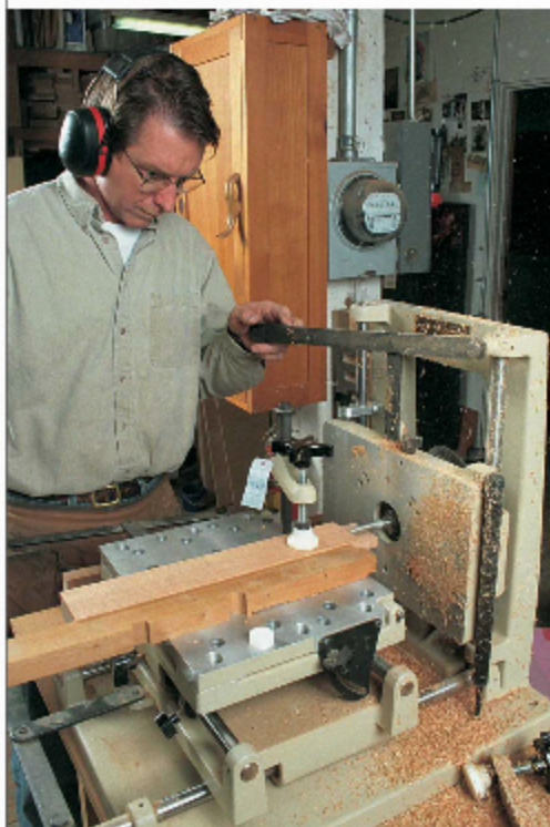
Routing machines for production work. Guided by templates or set by hand, the horizontal routing machine takes a little work to set up but can cut countless tenons in no time at all. The table also tilts to make easy work of angled tenons.
