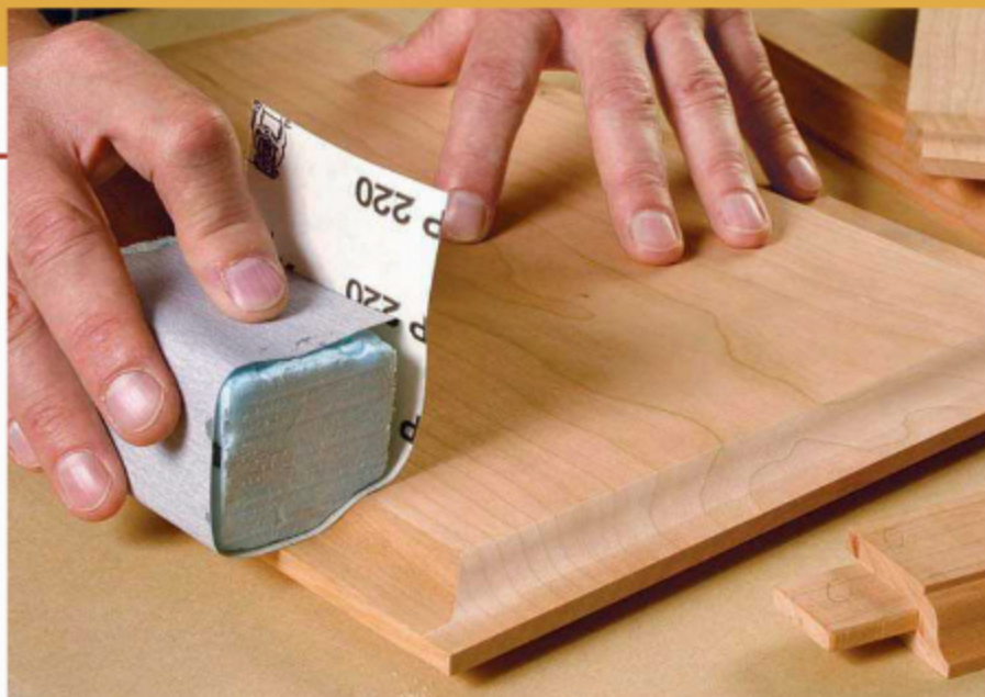
Rubber profiles. Using a rubber pad that fits the molding helps keep the edges of the profile sharp.
