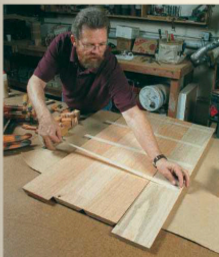
Packing tape binds the box. Stranded tape with embedded fiber has tremendous strength. Strips of tape are laid on the face side of the box, keeping everything in place.
