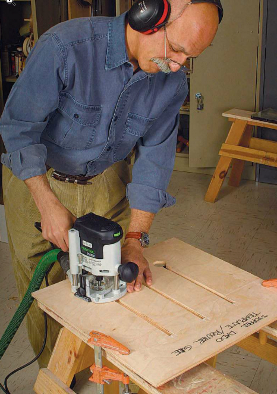
The template guides the router. A rub collar (or template guide) screwed to the router base runs against the template, guiding the router bit.
