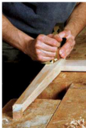
Plane the patch flush with the stock. Finally, ease the corners to protect the veneer and help blend it in.
