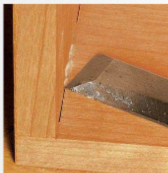
Cleaning up glue squeeze-out. A scraper works best for large areas, but for small areas, a chisel offers more control.
