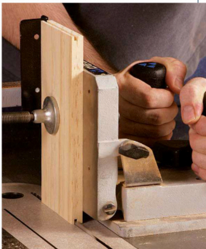
Rabbet the front and rear pieces in two steps. Using a commercial tenon jig to support the workpiece (above), make a vertical cut on the ends of each drawer box front and back. With the piece flat on the table (left), make the second cut, leaving a tongue that will connect with the side pieces.
