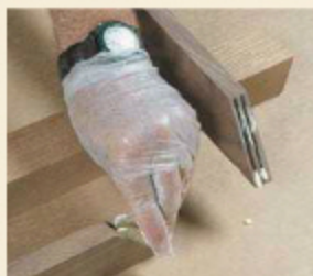
Use two biscuits. A pair of biscuits provides ample gluing surface and keeps the pieces aligned. Once clamps go on, measure the diagonals to make sure everything is square.
