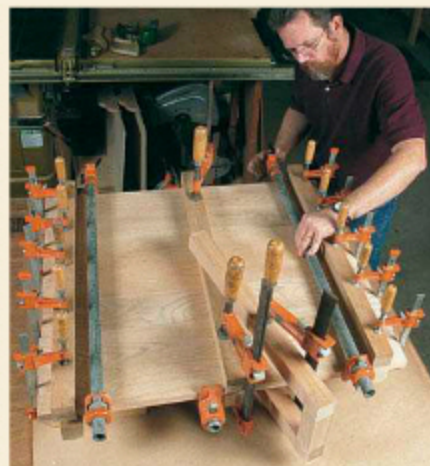
Bar clamps squeeze the joints together. Apply just enough pressure to close the joints—too much pressure will force glue out. Keep the bar clamps above the surface because black marks will appear everywhere the clamps touch the wet glue.
