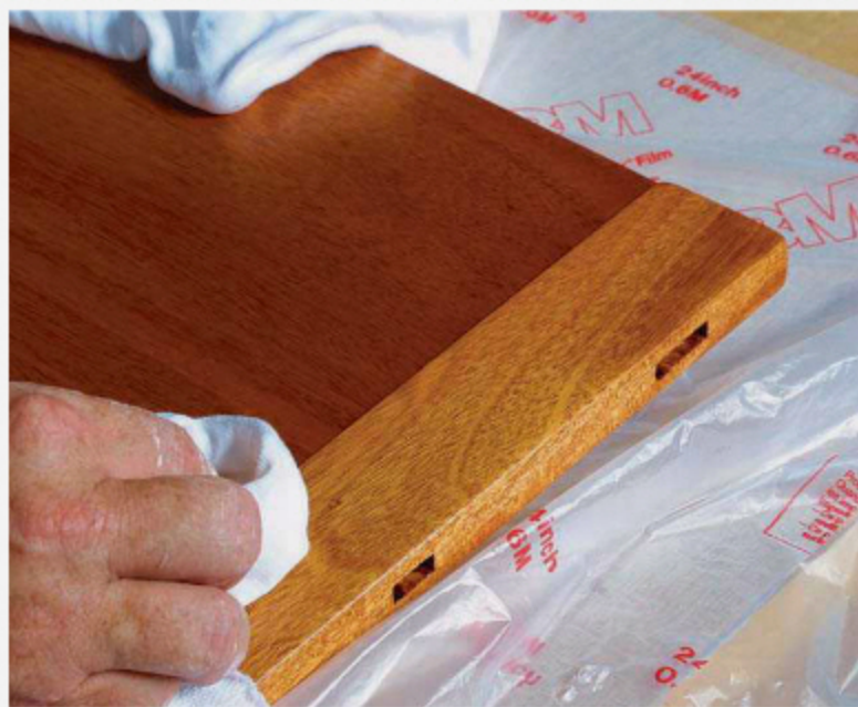
Sand on and wipe off. Before the varnish becomes tacky, wipe off the surplus using clean cotton rags. Keep changing the rags until no more finish can be removed and the surface can be buffed smooth.
