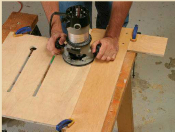
Cut the template guide. With a T-square guide clamped to the edge of the plywood template, rout the slots for the template guide to ride in.
