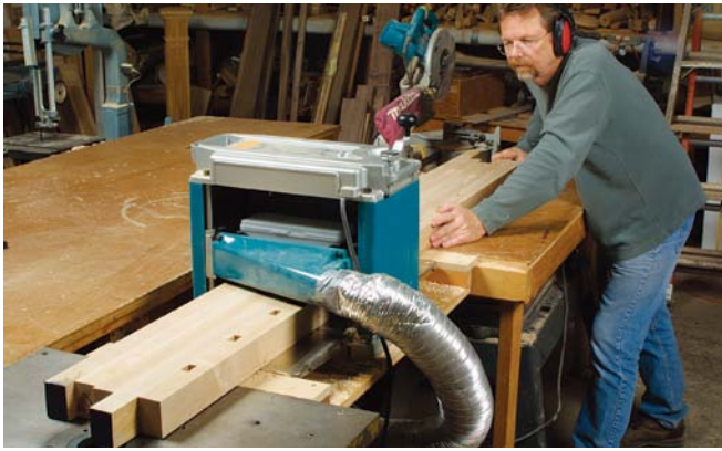
Flatten the slab. A five-board section of the top slab is narrow enough to fit through a benchtop planer.
