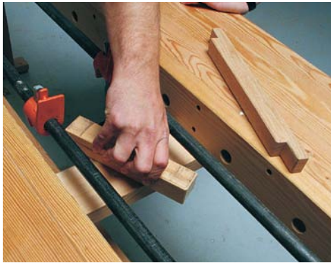
Pipes rest on blocks that turn. Tail-vise pipe clamps are supported by blocks fastened with one screw. To slide a clamp past, turn the block.
