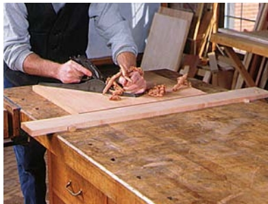
Securing the workpiece without clamps. A hardwood batten thinner than the workpiece butts against two benchdogs in the top to serve as a stop.
