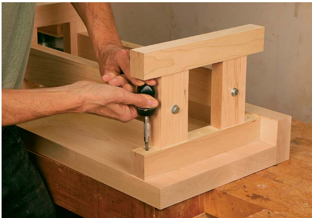
Attach the base. Mount the top to the base by driving three screws through holes (two slotted, one round) in each apron.
