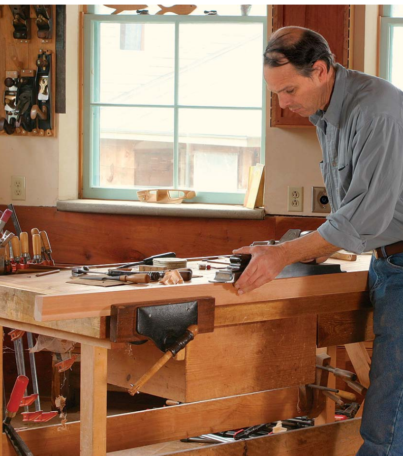
Secure long boards on edge. A block clamped in the tail vise supports the opposite end.
