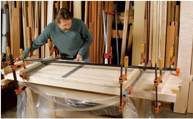
Now glue three sections into one big slab. Place a try square across the dog holes and use a long bar clamp diagonally to correct any misalignment. Again, use lots of clamps and cauls to keep the sections level.
