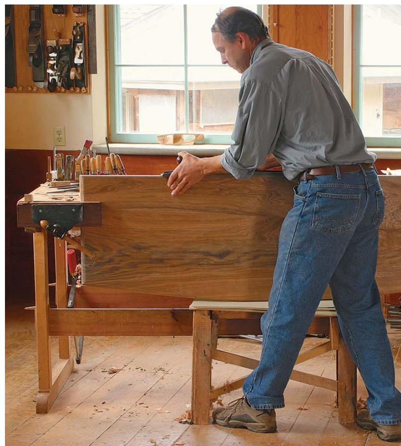
Steady a wide panel. A sawhorse provides support underneath, with the opposite end clamped to the bench apron.
