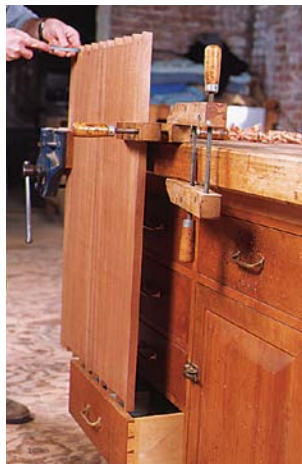
Drawers do more than hold things. In combination with the vise, they also support workpieces such as this large mahogany carcass piece.
