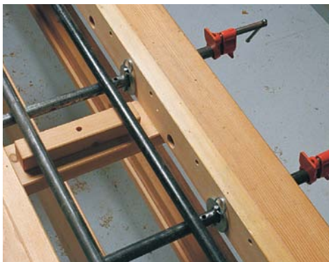
Front clamps are easy to adjust. The clamps fit in holes in the bench front and are secured with large washers and speed pins.
